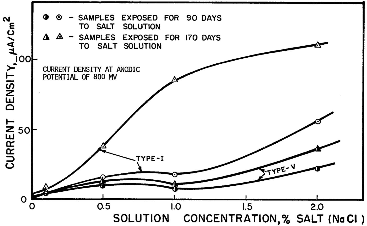
FIG. 30. PRESENTS THE ANODIC CURRENT DENSITY AS A FUNCTION OF SALT CONCENTRATED SOLUTIONS FOR TWO DIFFERENT TIME OF EXPOSURE.
