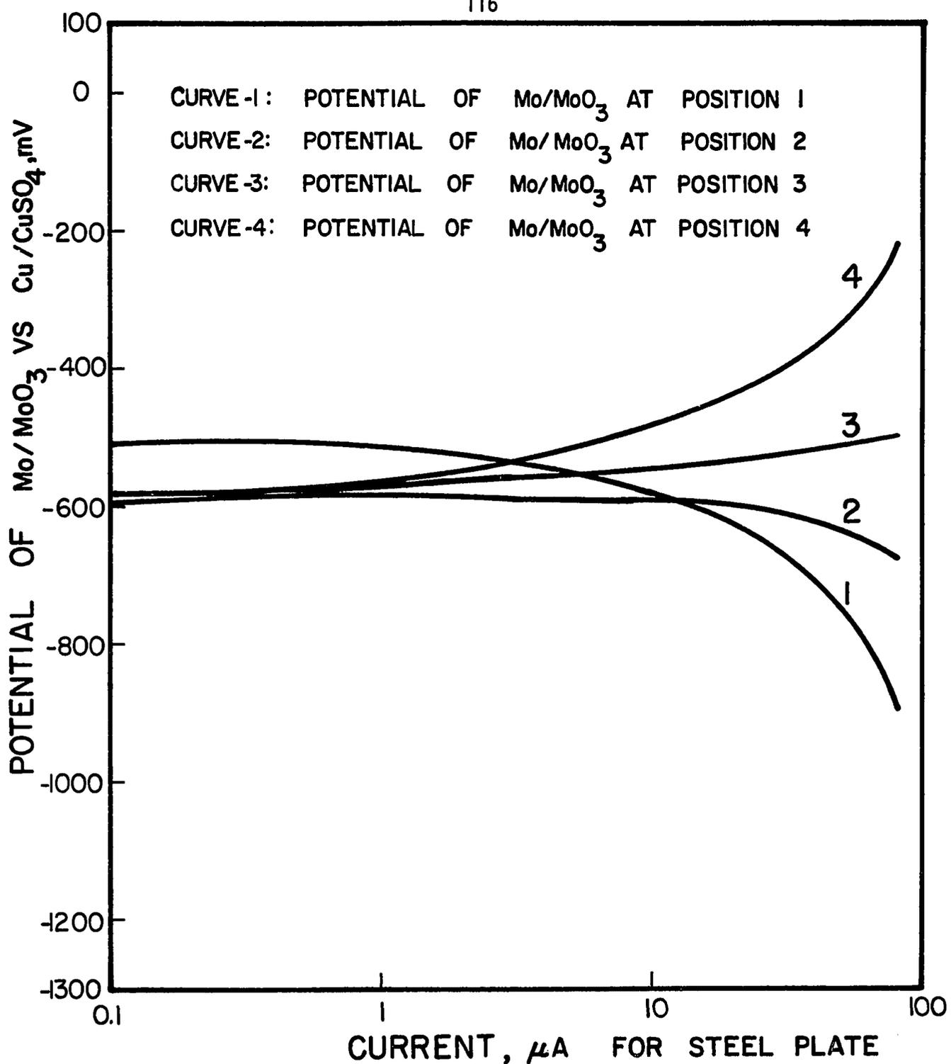
FIG. 56. POTENTIAL SHIFT OF Mo/MoO<sub>3</sub> ELECTRODES VS Cu/CuSO<sub>4</sub> AS A FUNCTION OF CATHODIC CURRENT FOR STEEL PLATE
