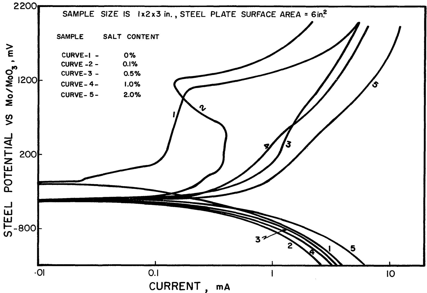
FIG. 19. POTENTIODYNAMIC ANODIC POLARIZATION OF STEEL PLATE IN TYPE I PORTLAND CEMENT CONCRETE CONTAINING VARIOUS PERCENTAGES OF SALT (NaCl). SAMPLES WERE IN DISTILLED WATER FOR 300 DAYS. [SWEEP RATE = 0.28 MV/SEC.]
