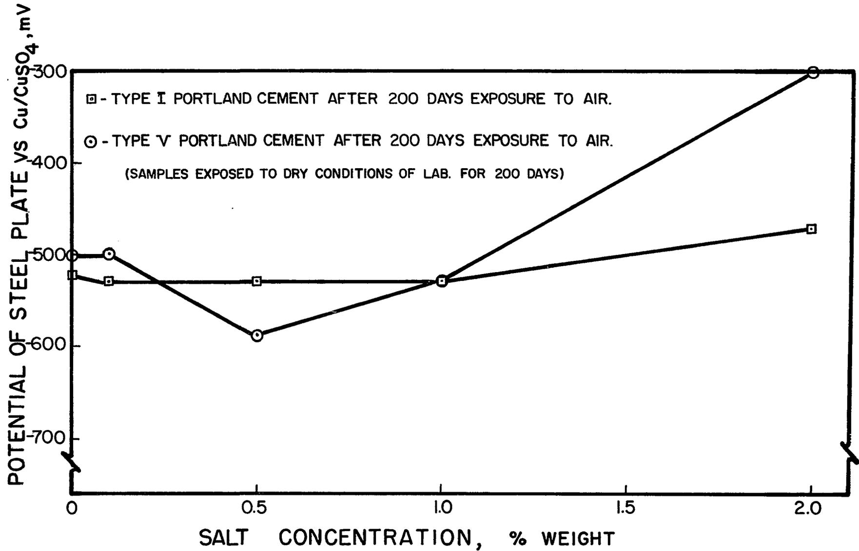
FIG. 15. CORROSION POTENTIAL OF STEEL AS A FUNCTION OF SALT CONTENT IN TYPE I AND V PORTLAND CEMENT CONCRETE.
