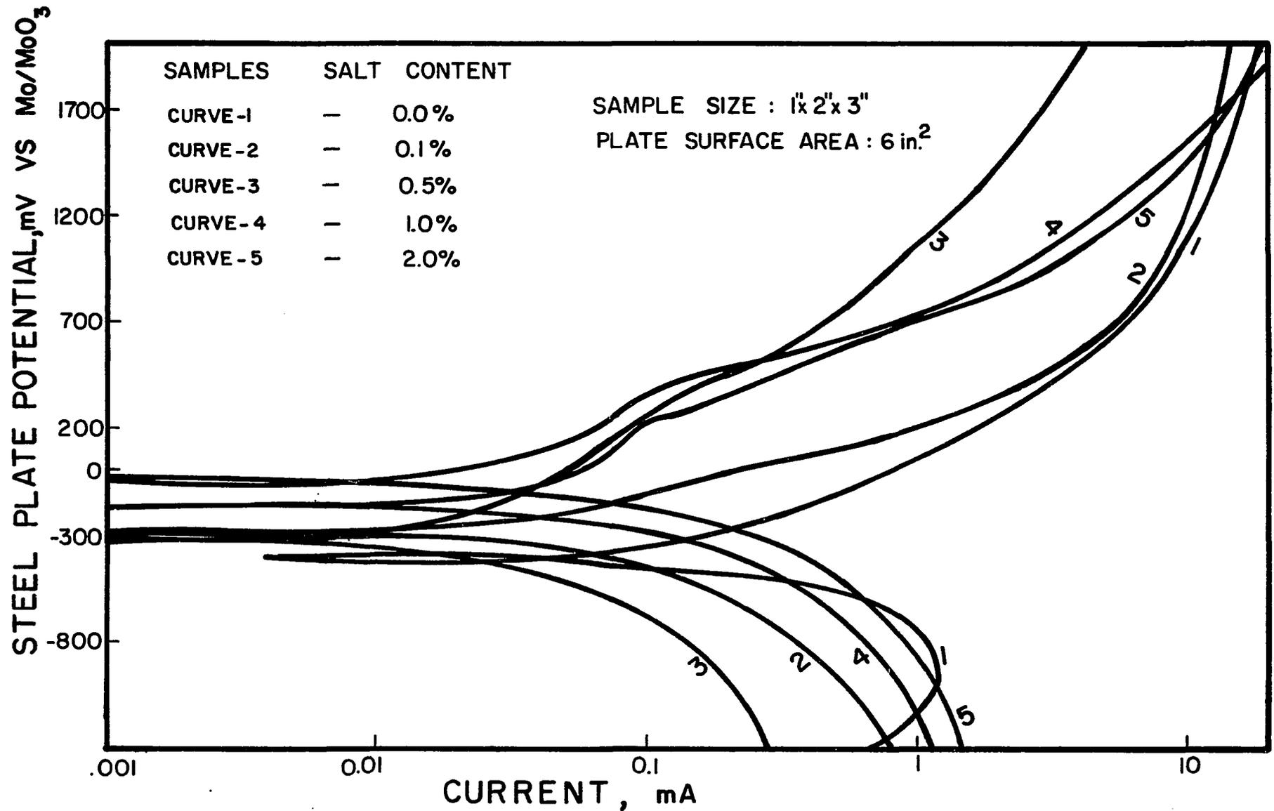
FIG. 14 . POTENTIODYNAMIC ANODIC POLARIZATION OF STEEL PLATE IN TYPE V PORTLAND CEMENT CONCRETE CONTAINING VARIOUS PERCENTAGES OF SALT (NaCl). SAMPLES WERE IN DRY CONDITION OF LABORATORY FOR 300 DAYS. [SWEEP RATE = 0.28 MV/SEC.]
