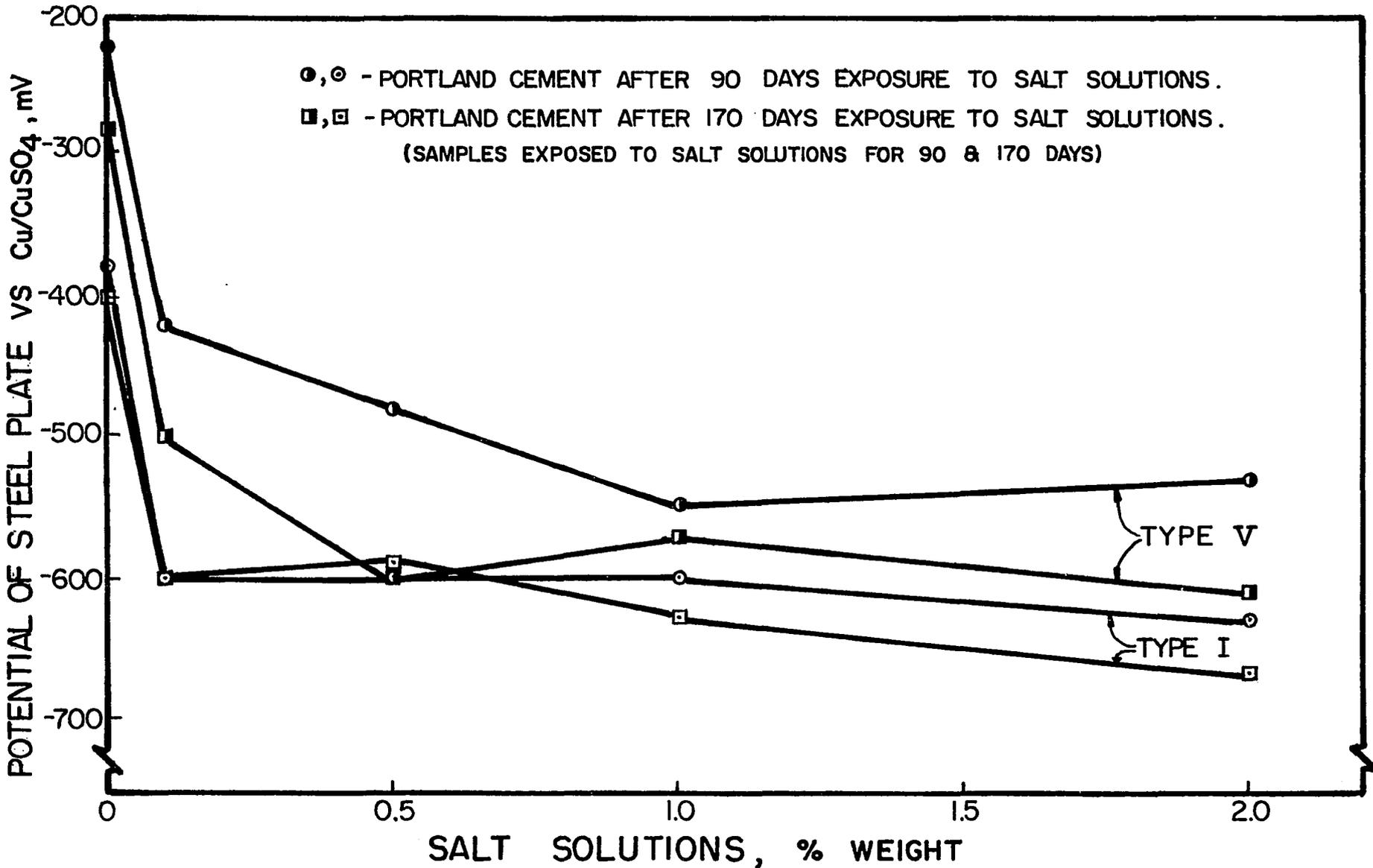
FIG. 32. CORROSION POTENTIAL OF STEEL IN TYPE I AND V PORTLAND CEMENT CONCRETE SAMPLES EXPOSED TO VARIOUS SALT CONCENTRATED SOLUTIONS. SAMPLES WERE EXPOSED TO SALT SOLUTIONS FOR 90 AND 170 DAYS.
