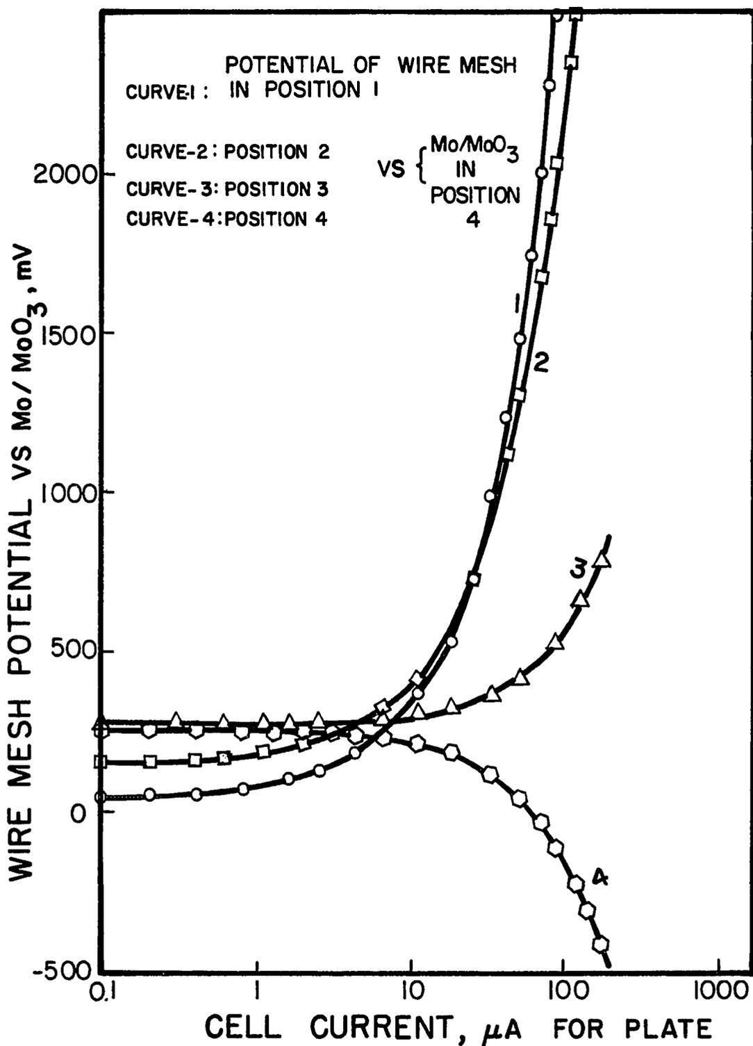
FIG. 54. SHIFT IN WIRE MESH POTENTIAL AS A FUNCTION OF CURRENT REQUIRED FOR ANODIC POLARIZATION OF STEEL PLATE.
