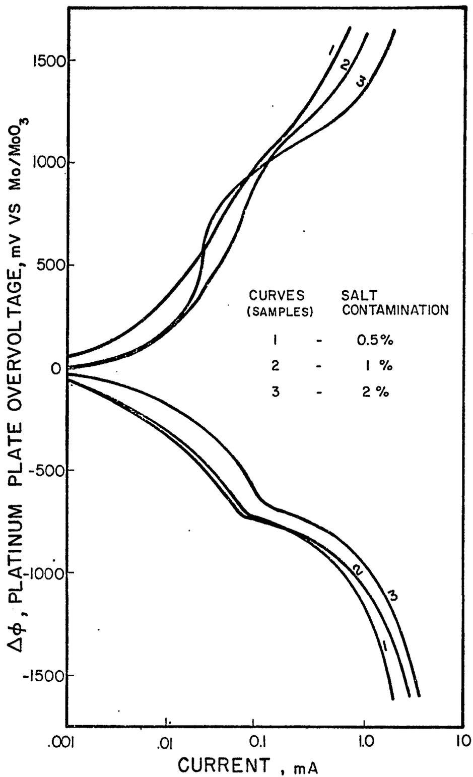
FIG. 22. POTENTIODYNAMIC ANODIC AND CATHODIC POLARIZATION OF PLATINUM PLATE IN TYPE I PORTLAND CEMENT CONTAINING VARIOUS PERCENTAGES OF SALT (NaCl), THE SAMPLES HAVE BEEN SOAKED IN DISTILLED WATER FOR 35 DAYS.
