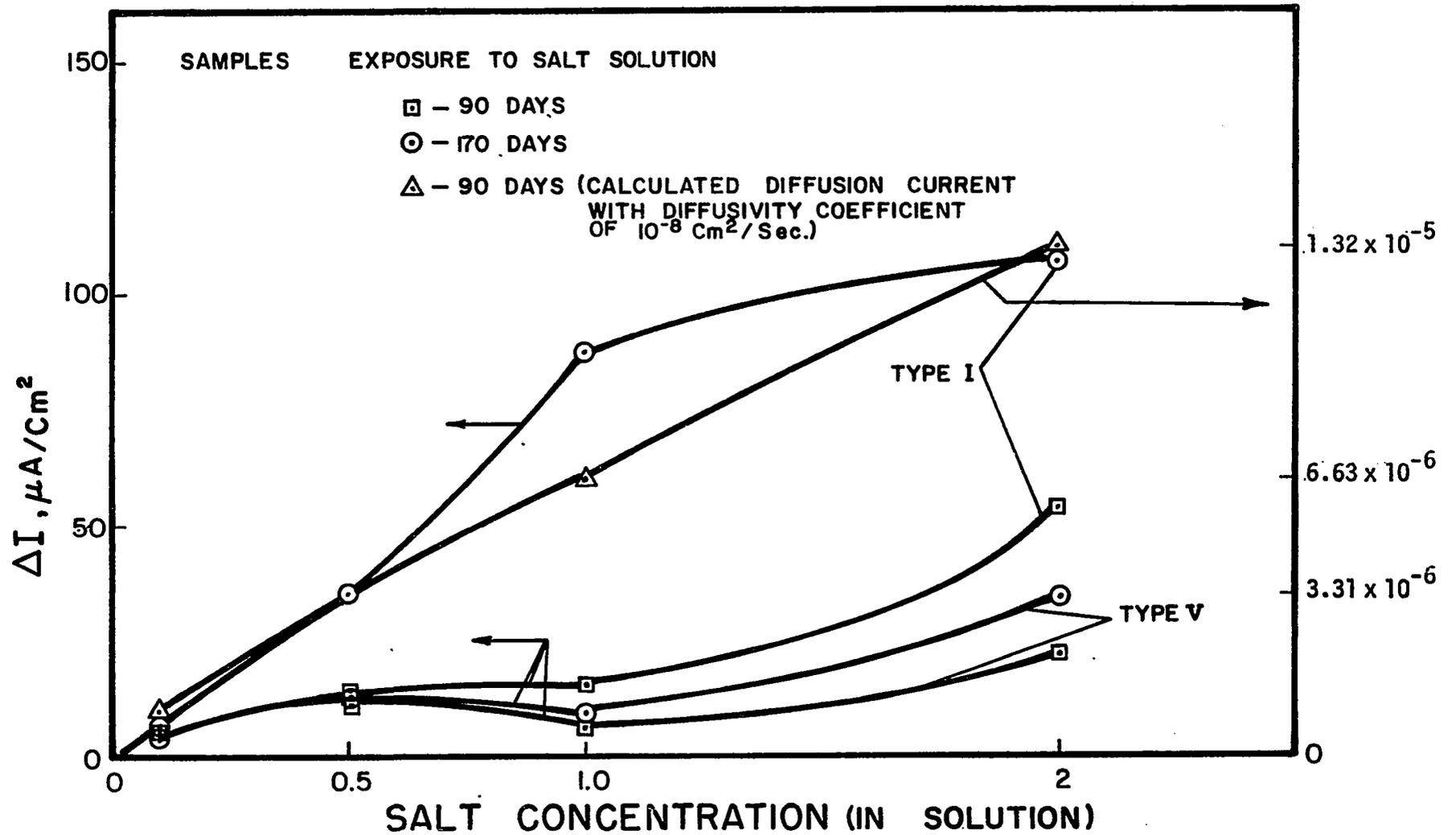
FIG. 31 . DIFFERENTIAL ANODIC CURRENT DENSITY CAUSED BY CHLORIDE IONS AT POTENTIAL OF +800 MV VS Mo/MoO<sub>3</sub> ELECTRODE. THE CURRENT CALCULATED BY THE CHLORIDE DIFFUSION PROCESS IS ALSO SHOWN. THE CONCRETE SAMPLES OF TYPE I AND V PORTLAND CEMENT WERE EXPOSED TO VARIOUS SALT SOLUTIONS FOR A PERIOD OF 90 TO 170 DAYS.
