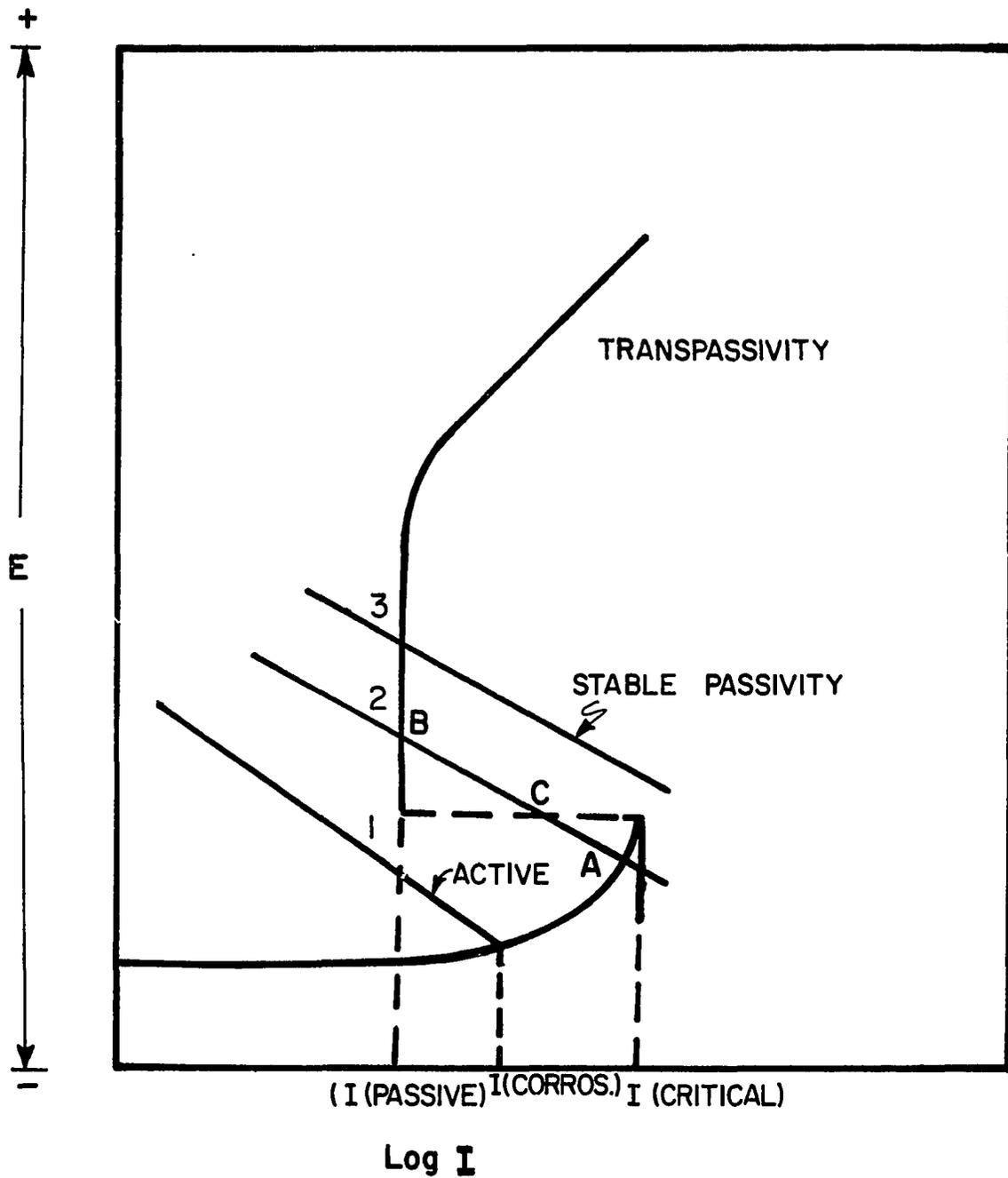
FIG. 1. ANODIC POTENTIOSTATIC POLARIZATION FOR EITHER ACTIVE OR PASSIVE METAL, DEPENDING ON OVERVOLTAGE OF CATHODIC AREAS.
