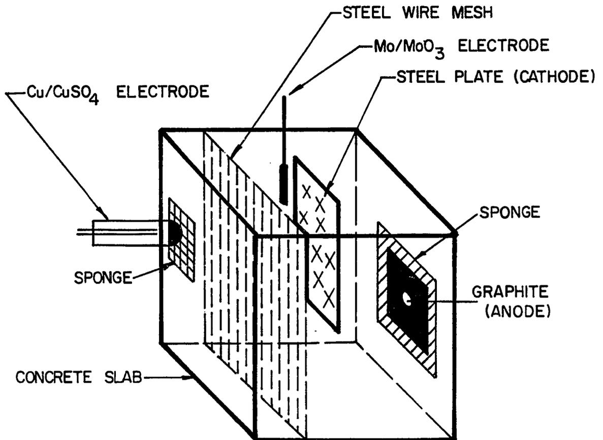
FIG. 46. CELL ASSEMBLY FOR CONCRETE SLAB WITH WIRE MESH OUTSIDE OF ELECTRIC FIELD BETWEEN ANODE AND CATHODE.
