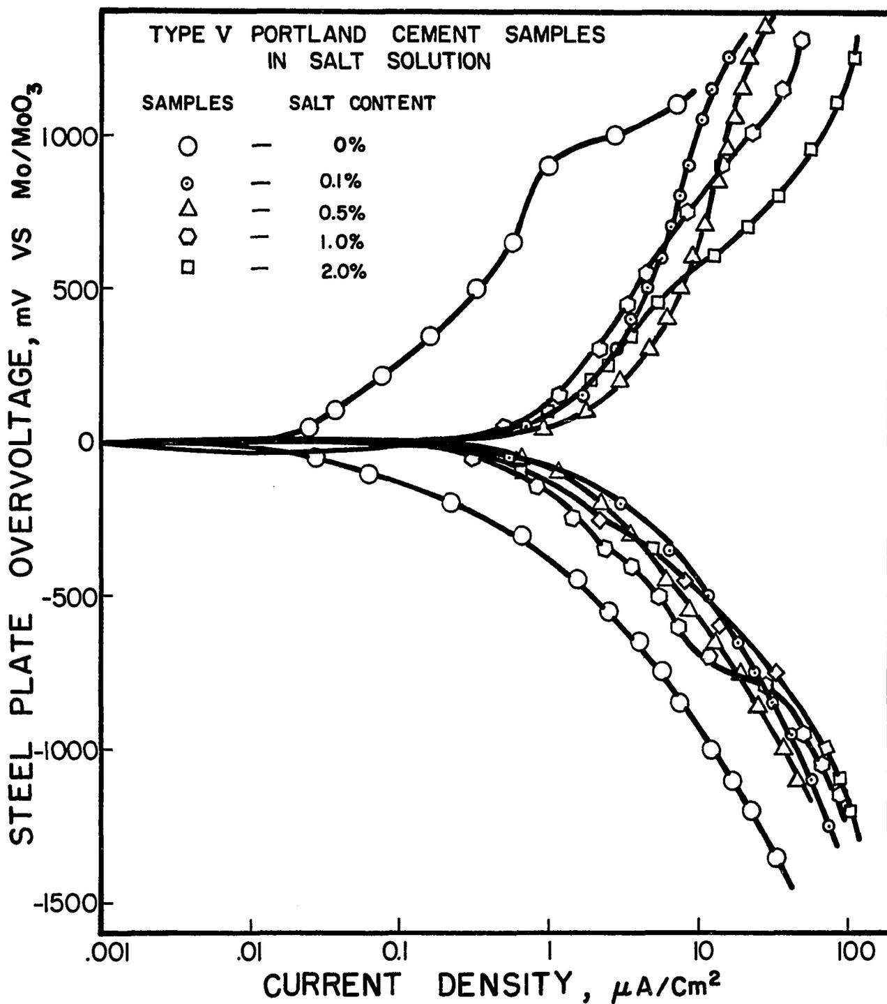
FIG. 28. ANODIC AND CATHODIC POLARIZATION OF STEEL IN TYPE V PORTLAND CEMENT CONCRETE. THE CONCRETE SAMPLES WERE IN VARIOUS SALT CONTAMINATED SOLUTIONS FOR 170 DAYS.
