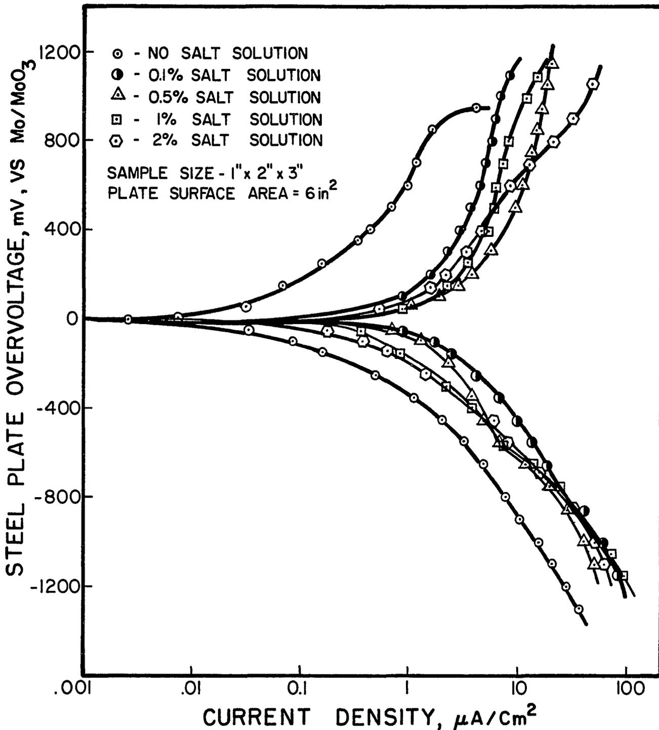
FIG. 25. ANODIC AND CATHODIC POLARIZATION OF STEEL IN TYPE V PORTLAND CEMENT CONCRETE IN VARIOUS SALT CONCENTRATED SOLUTIONS. THE CONCRETE SAMPLES WERE IN SALT SOLUTION FOR 90 DAYS.
