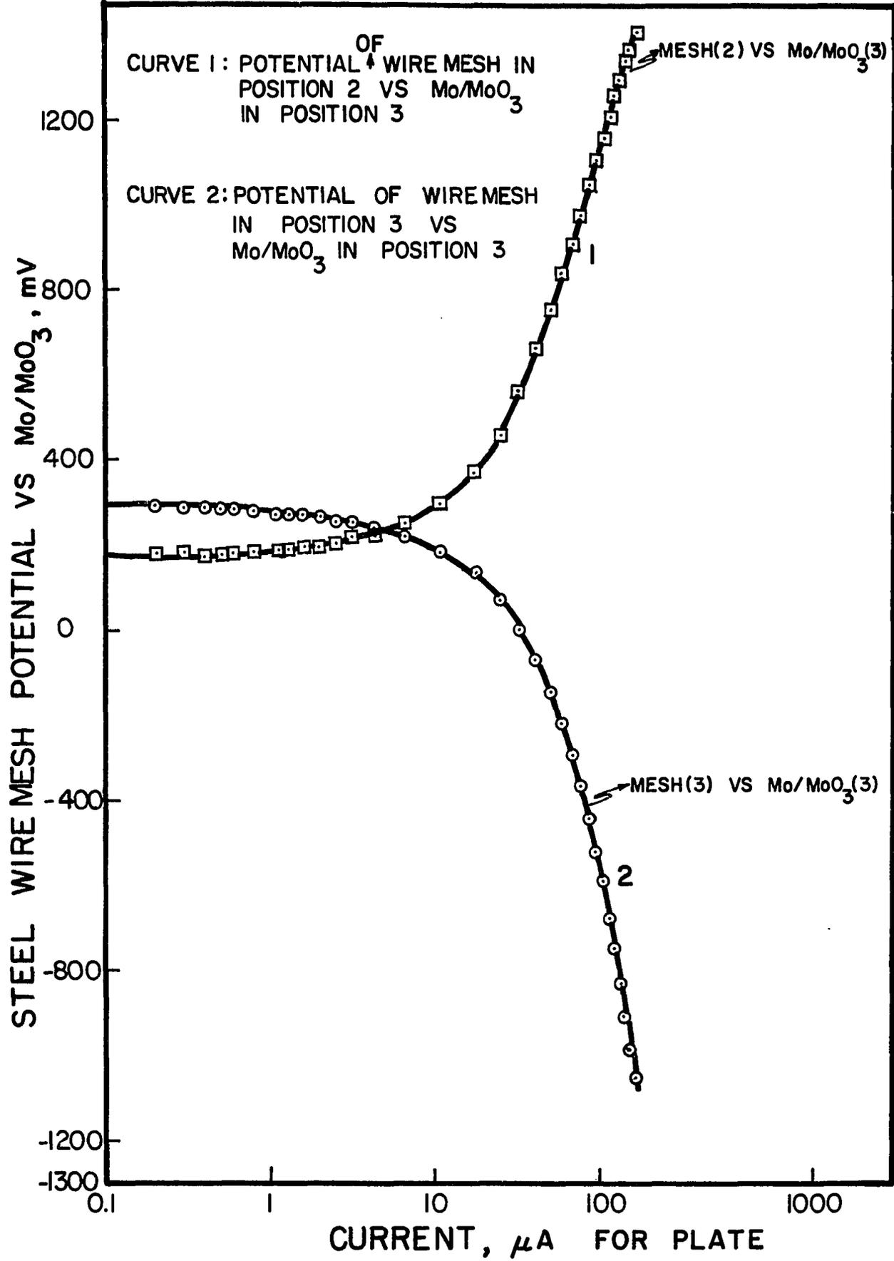
FIG. 55. SHIFT IN WIREMESH POTENTIAL AS A FUNCTION OF CURRENT REQUIRED FOR ANODIC POLARIZATION OF STEEL PLATE
