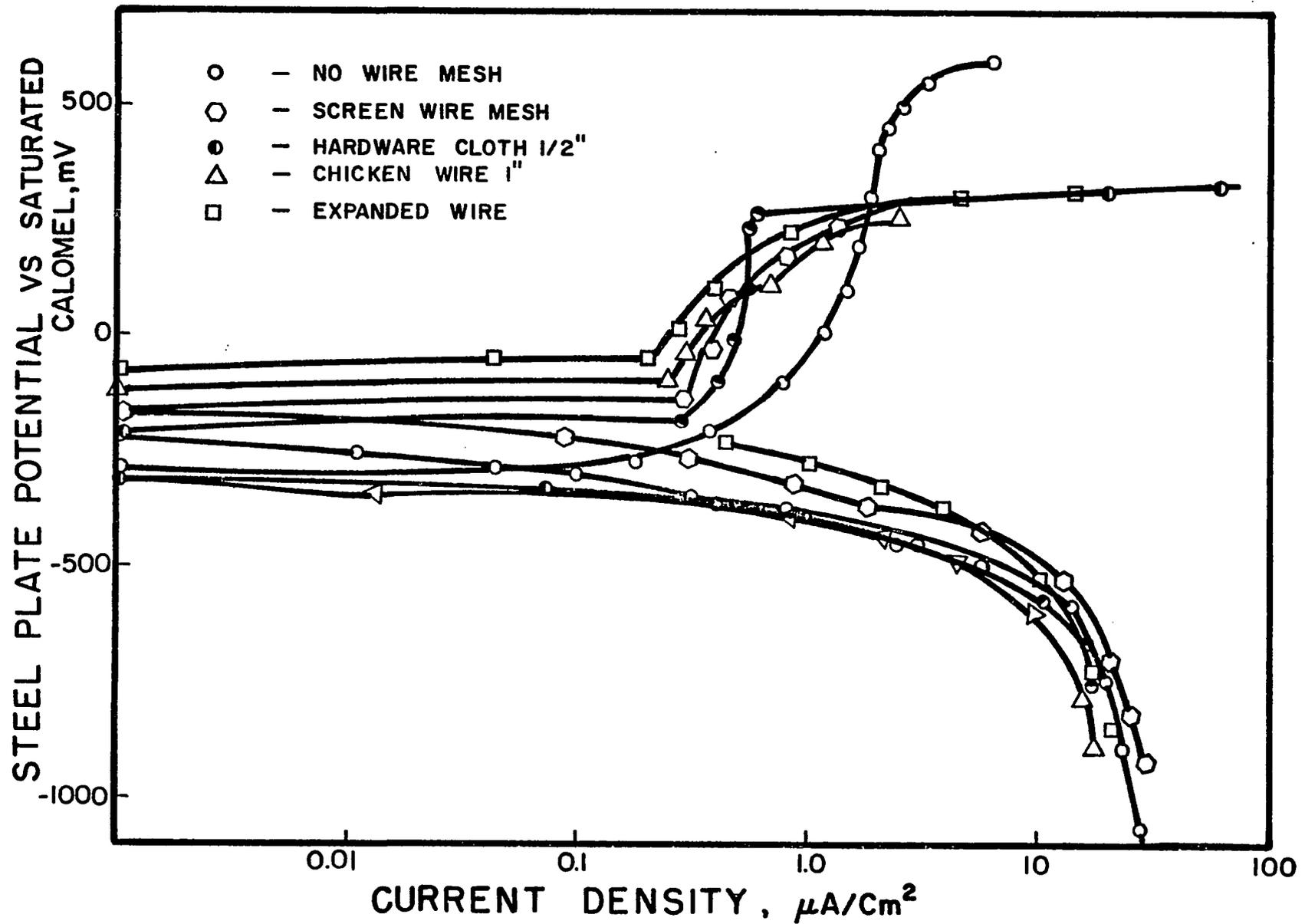
FIG. 36. ANODIC AND CATHODIC POLARIZATION OF STEEL IN SATURATED  $\text{Ca}(\text{OH})_2$  SOLUTION WITH AND WITHOUT WIRE MESH (VARIOUS MESH SIZE) ATTACHED TO TOP AND BOTTOM OF STEEL PLATE, REST ABOUT 1" FROM PLATE.
