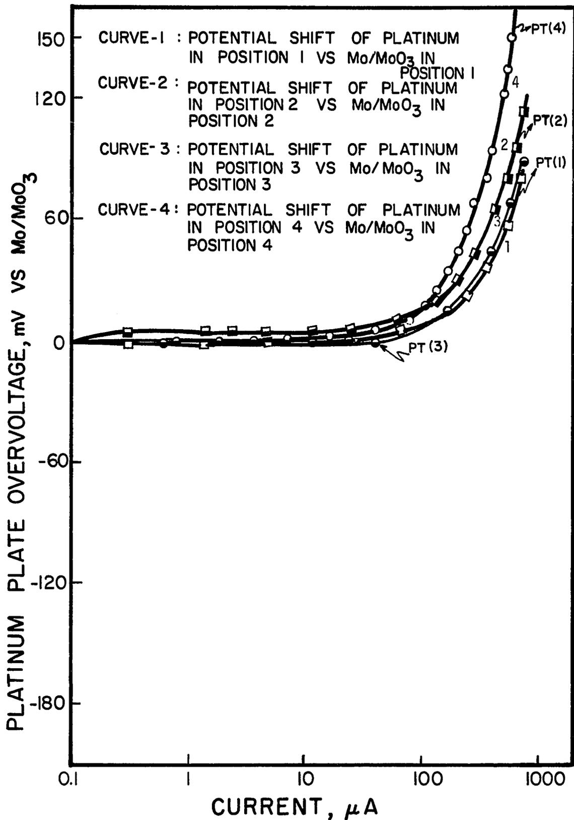
FIG. 58. POTENTIAL SHIFT OF PLATINUM PLATES AS A FUNCTION OF DISTANCE BETWEEN ANODE AND CATHODE AS A RESULT OF ANODIC POLARIZATION IN TYPE I PORTLAND CEMENT CONCRETE.
