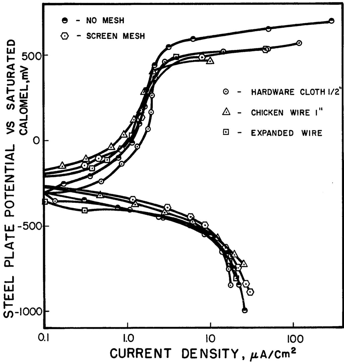
FIG. 37. ANODIC AND CATHODIC POLARIZATION OF STEEL IN SATURATED  $\text{Ca}(\text{OH})_2$  SOLUTION WITH AND WITHOUT WIRE MESH (VARIOUS SIZES) LYING ON STEEL PLATE.
