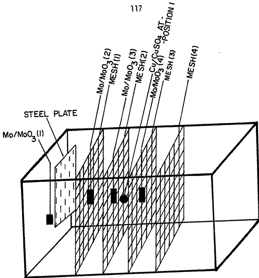
FIG. 57. CONCRETE SAMPLE WITH ONE STEEL PLATE AND FOUR STEEL WIRE MESHES AND FOUR  $\text{Mo/MoO}_3$  ELECTRODES ADJACENT TO PLATE AND WIRE MESHES. WIRE MESHES ARE 4 Cm. APART FROM ONE ANOTHER AND EMBEDDED BETWEEN ANODE AND CATHODE.
