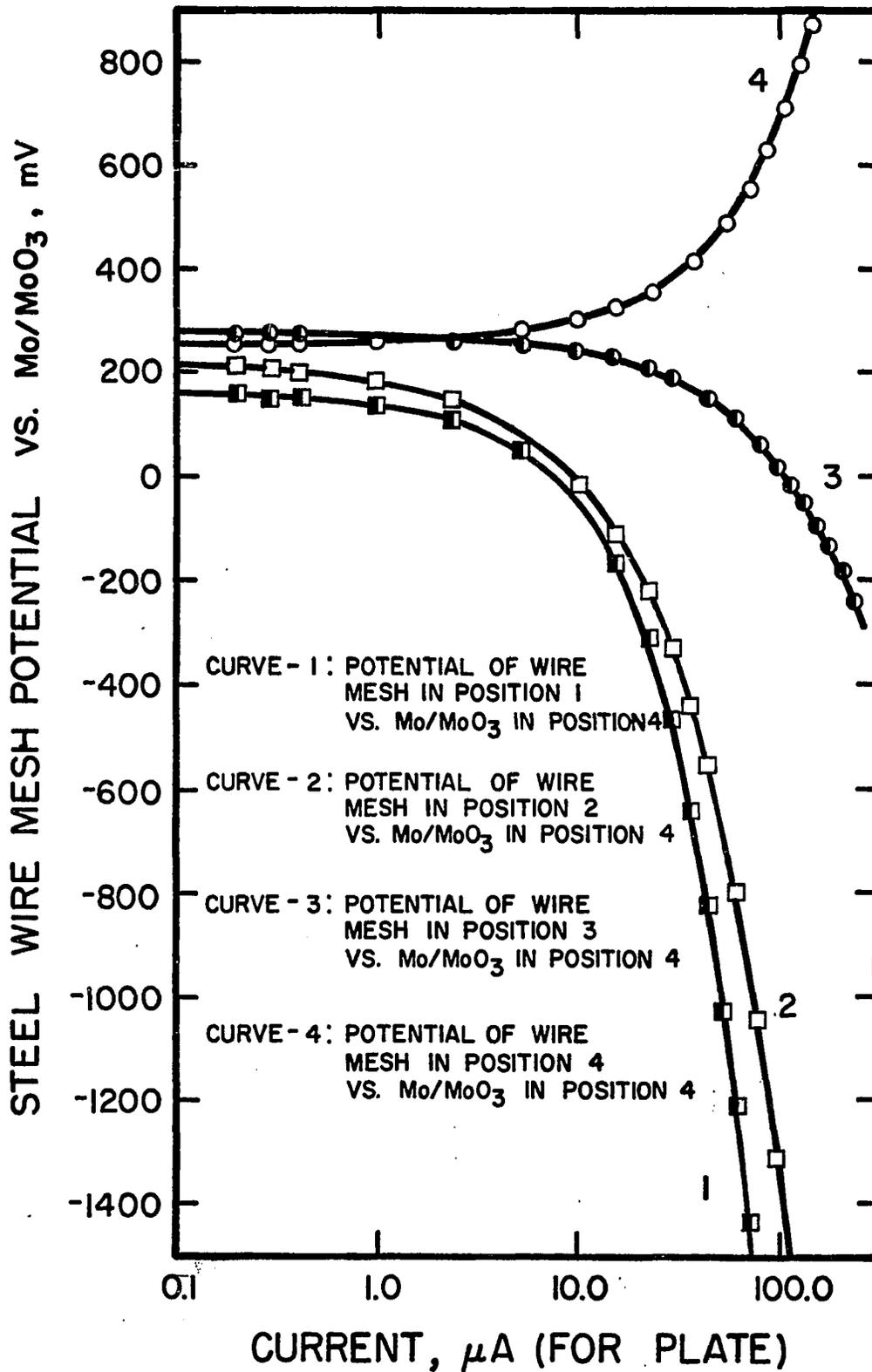
FIG. 50. SHIFT IN STEEL WIRE MESH POTENTIAL AS A FUNCTION OF CURRENT REQUIRED FOR CATHODIC POLARIZATION OF STEEL PLATE.
