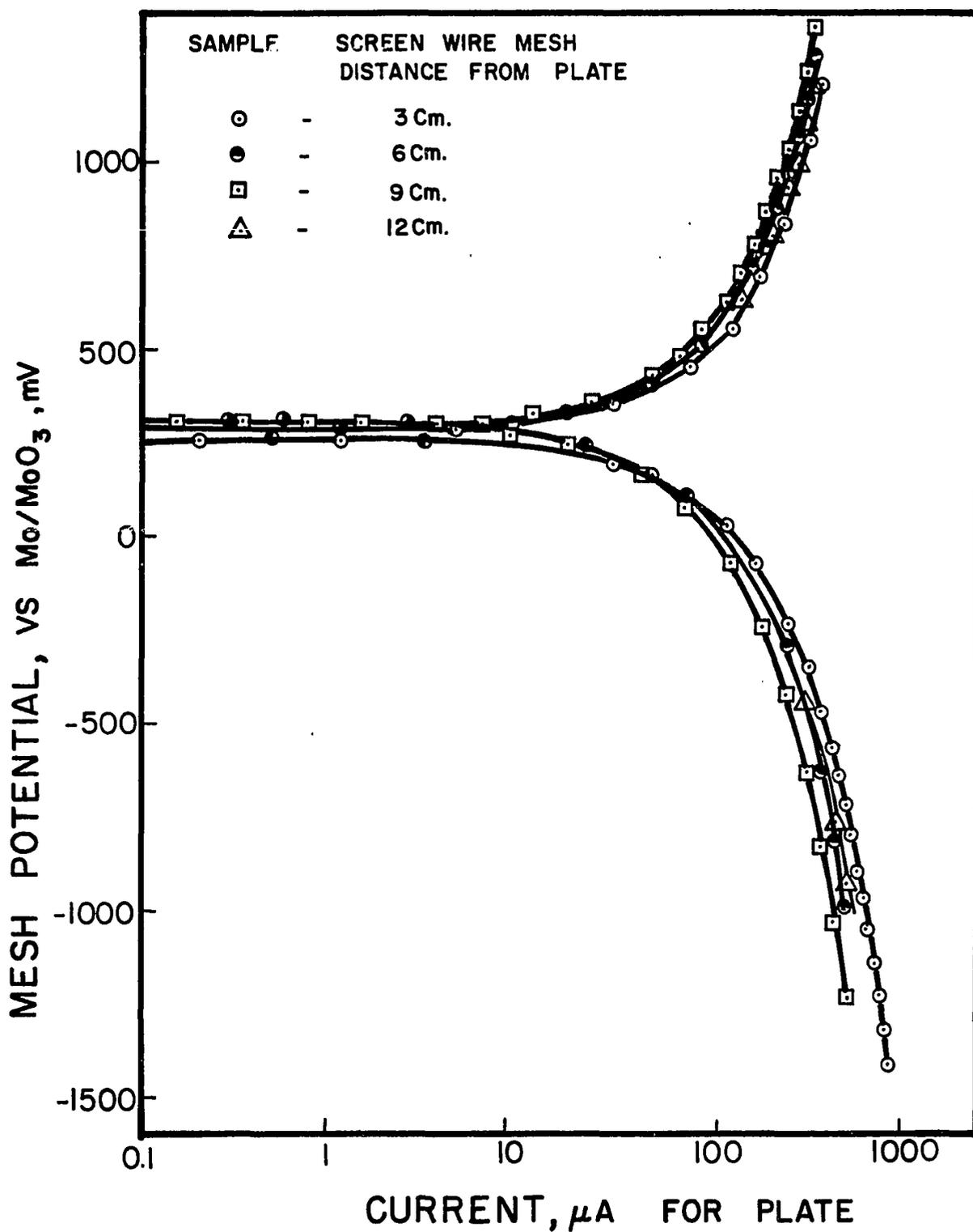
FIG. 47. POTENTIAL VARIATION OF SCREEN WIRE MESH AT VARIOUS DISTANCES FROM THE PLATE AS A RESULT OF ANODIC AND CATHODIC POLARIZATION OF STEEL PLATE IN TYPE I PORTLAND CEMENT CONCRETE.
