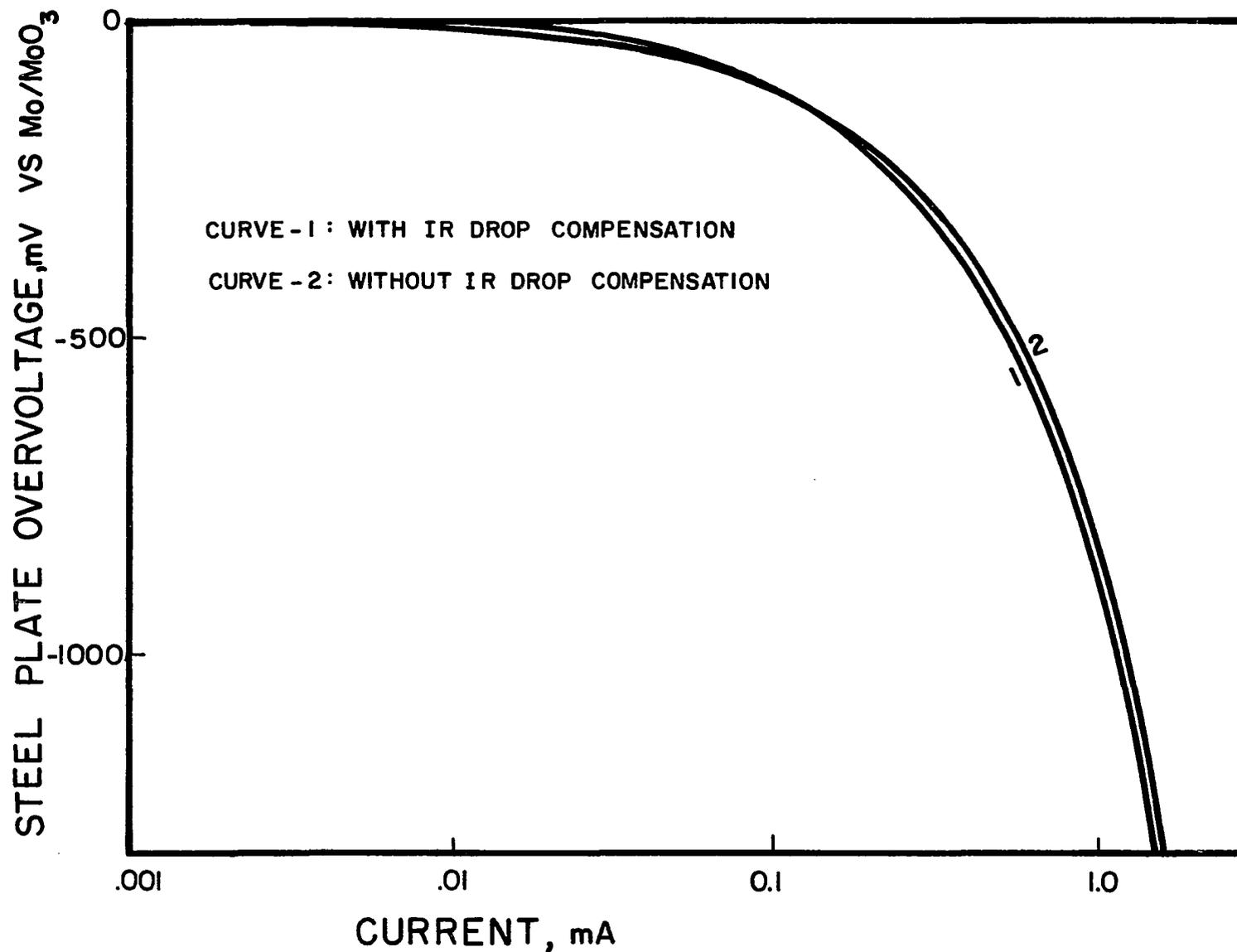
FIG. 33. POTENTIODYNAMIC CATHODIC POLARIZATION OF STEEL PLATE WITH AND WITHOUT IR DROP COMPENSATION COMPARED TO Mo/MoO<sub>3</sub> ELECTRODE IN 2% SALT CONTAMINATED CONCRETE OF TYPE V PORTLAND CEMENT. CONCRETE SAMPLE WAS IN DRY CONDITION OF LABORATORY FOR 300 DAYS.
