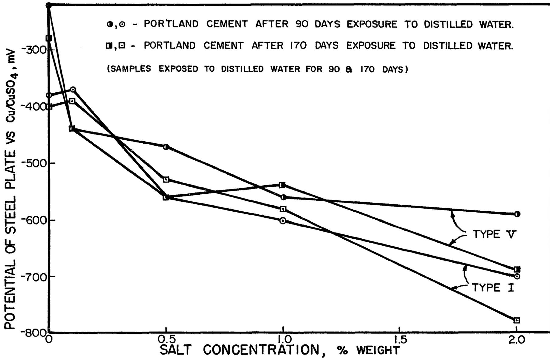
FIG. 23. CORROSION POTENTIAL OF STEEL AS A FUNCTION OF SALT CONTENT IN TYPE I AND V PORTLAND CEMENT CONCRETE.
