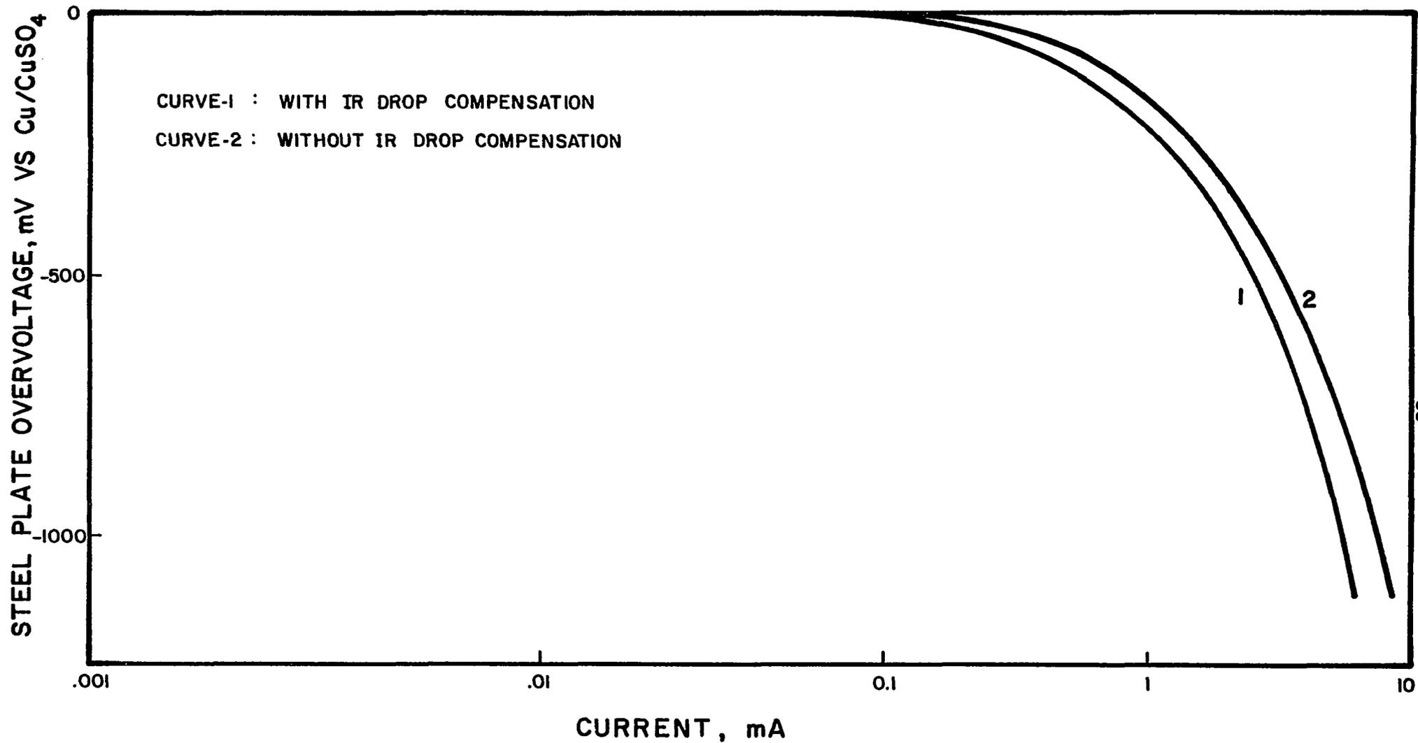
FIG. 34. CATHODIC POLARIZATION OF STEEL PLATE COMPARED TO  $\text{Cu}/\text{CuSO}_4$  ELECTRODE WITH AND WITHOUT IR DROP COMPENSATION IN 2% SALT CONTAMINATED CONCRETE OF TYPE V PORTLAND CEMENT.
