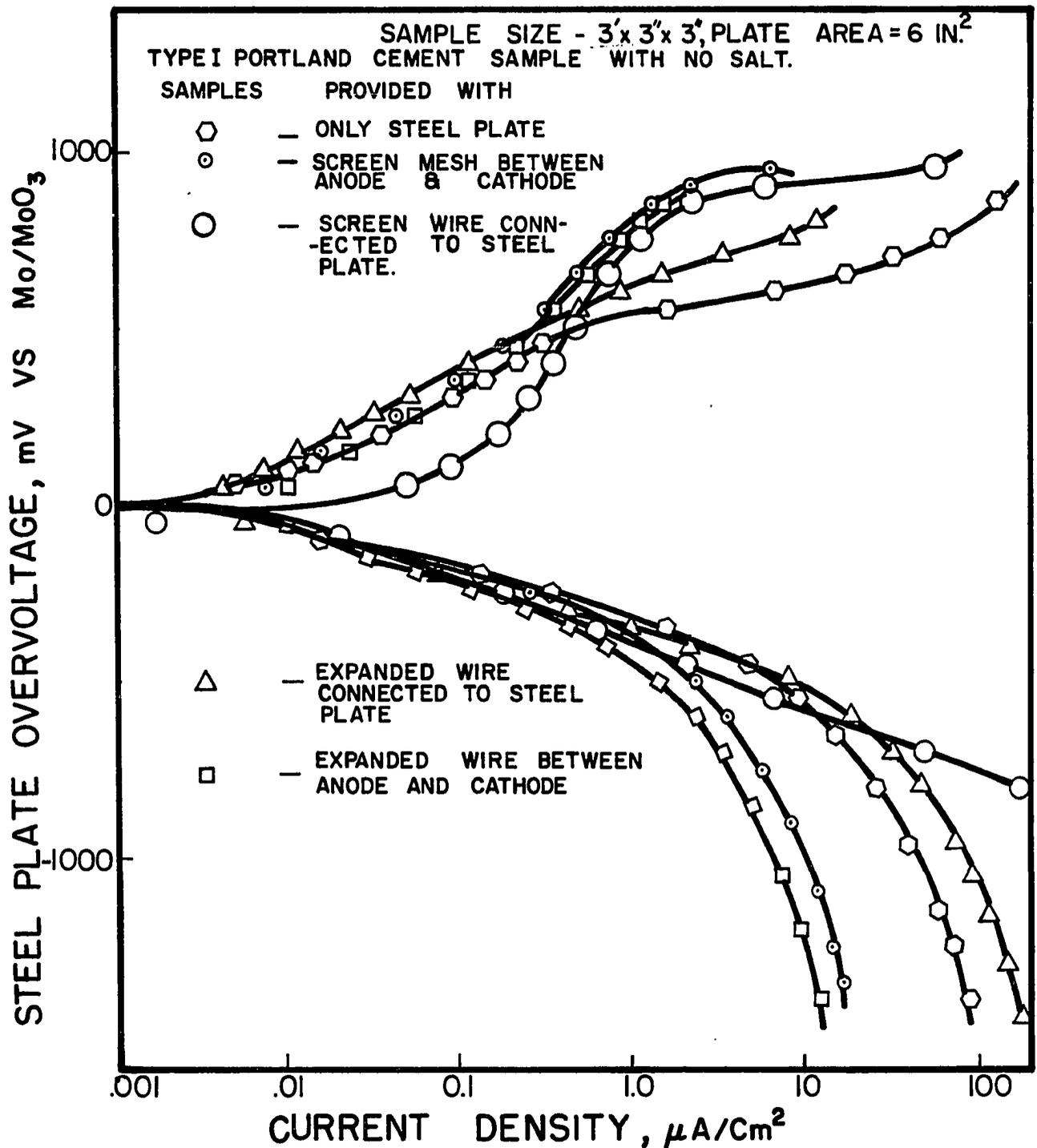
FIG. 41. ANODIC AND CATHODIC POLARIZATION OF STEEL PLATE IN PRESENCE OF WIRE MESH IN TYPE I PORTLAND CEMENT CONCRETE. SAMPLES WERE IN DRY CONDITION OF LABORATORY FOR 20 TO 30 DAYS AFTER CURING.
