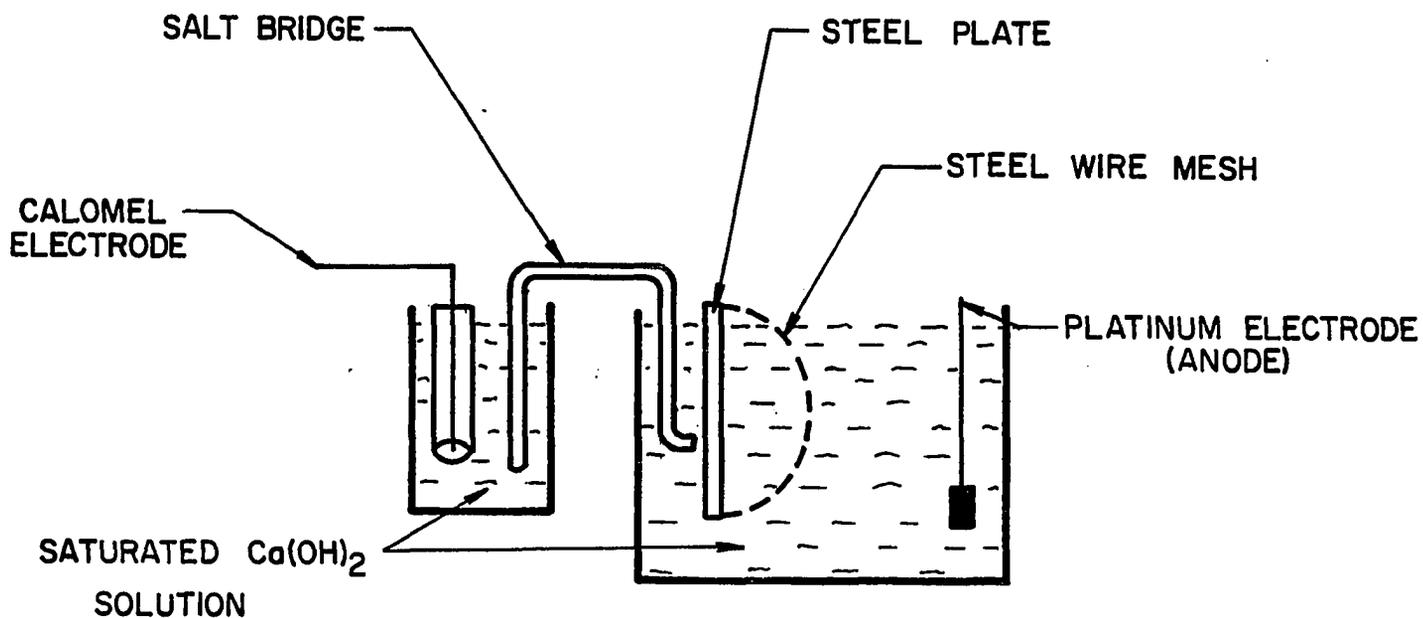
FIG. 9. CELL ASSEMBLY FOR ANODIC AND CATHODIC POLARIZATION OF STEEL PLATE WHEN STEEL WIRE MESH IS ATTACHED TO TOP AND BOTTOM OF STEEL PLATE IN SATURATED  $\text{Ca(OH)}_2$  SOLUTION.
