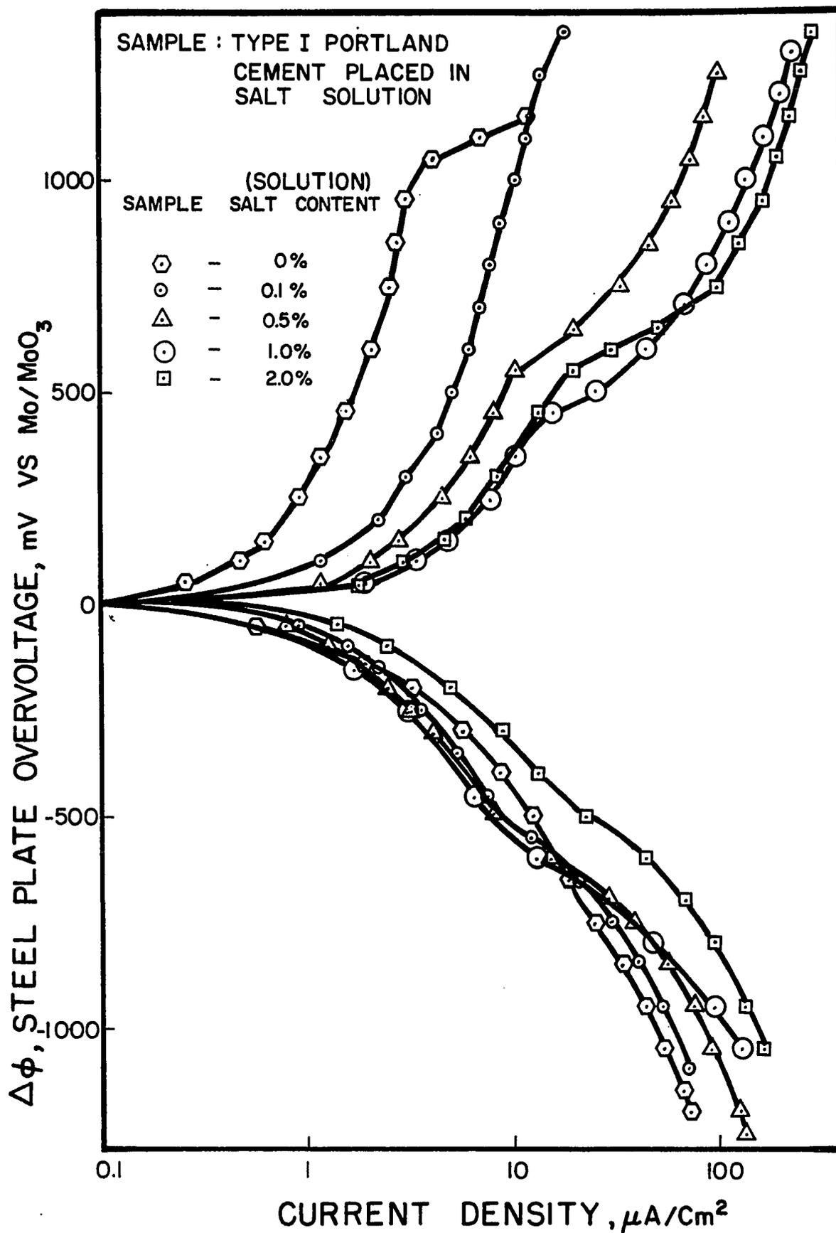
FIG. 26. ANODIC AND CATHODIC POLARIZATION OF STEEL IN TYPE I PORTLAND CEMENT CONCRETE. THE CONCRETE SAMPLES WERE IN VARIOUS SALT CONTAMINATED SOLUTIONS FOR 170 DAYS.
