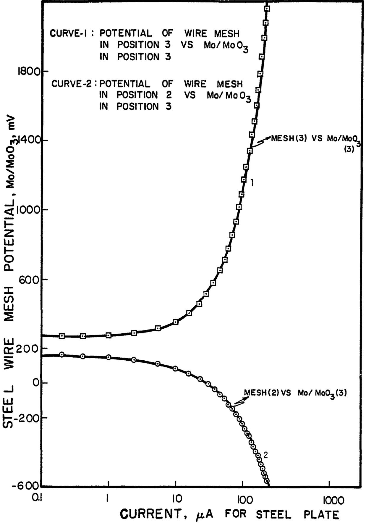
FIG. 51. SHIFT IN WIRE MESH POTENTIAL AS AS A FUNCTION OF CURRENT REQUIRED FOR CATHODIC POLARIZATION OF STEEL PLATE.
