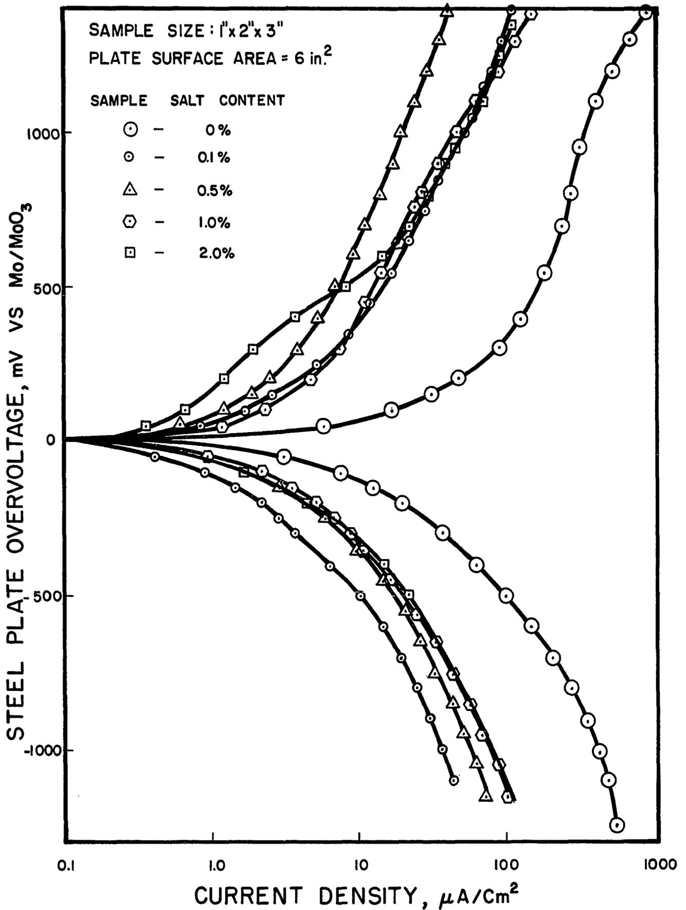
FIG. 11. ANODIC AND CATHODIC POLARIZATION OF STEEL IN TYPE I PORTLAND CEMENT CONCRETE WITH VARIOUS SALT CONTENTS. THE CONCRETE SAMPLES WERE IN DRY CONDITION OF LABORATORY FOR 200 DAYS.
