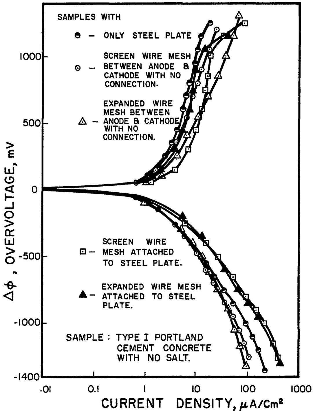
FIG. 42. ANODIC AND CATHODIC POLARIZATION OF STEEL PLATE IN PRESENCE OF WIRE MESH IN TYPE I PORTLAND CEMENT CONCRETE. SAMPLES WERE EXPOSED TO DISTILLED WATER FOR 4 MONTHS.
