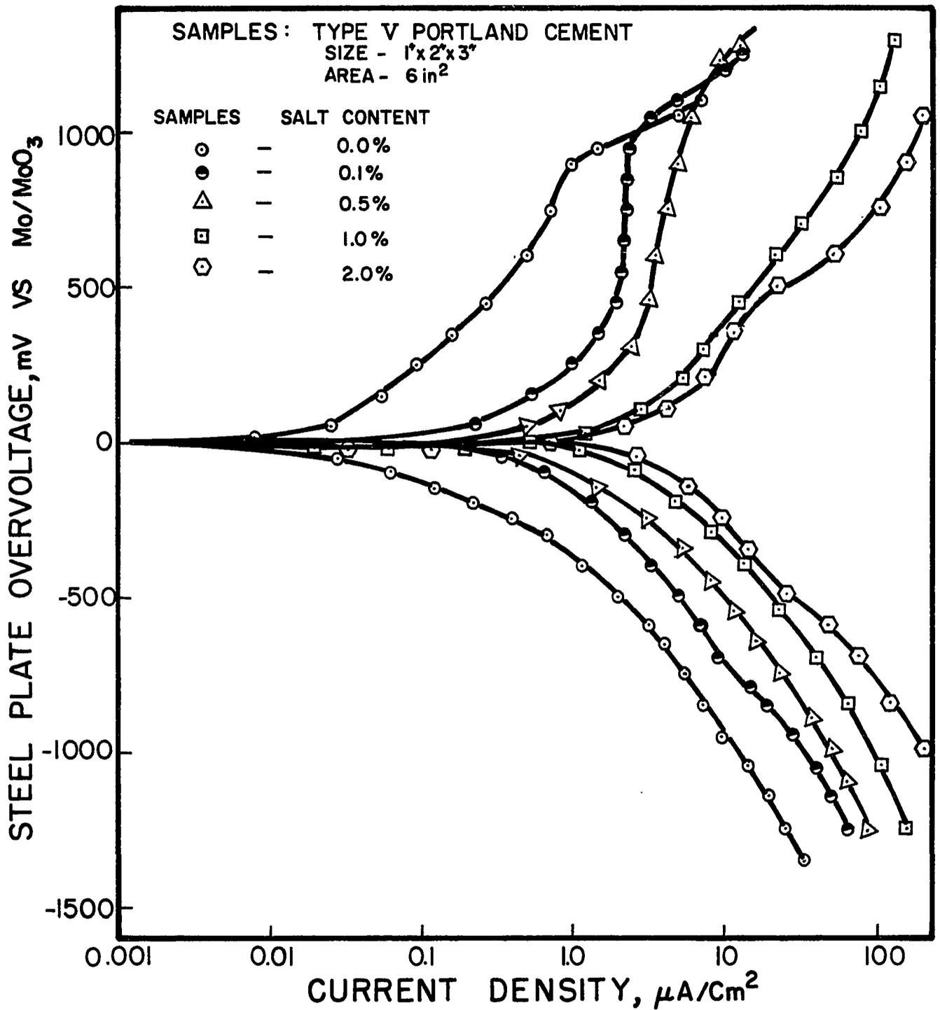
FIG. 20. ANODIC AND CATHODIC POLARIZATION OF STEEL IN TYPE V PORTLAND CEMENT WITH VARIOUS SALT CONTENTS. THE CONCRETE SAMPLES WERE IN WATER FOR 170 DAYS.
