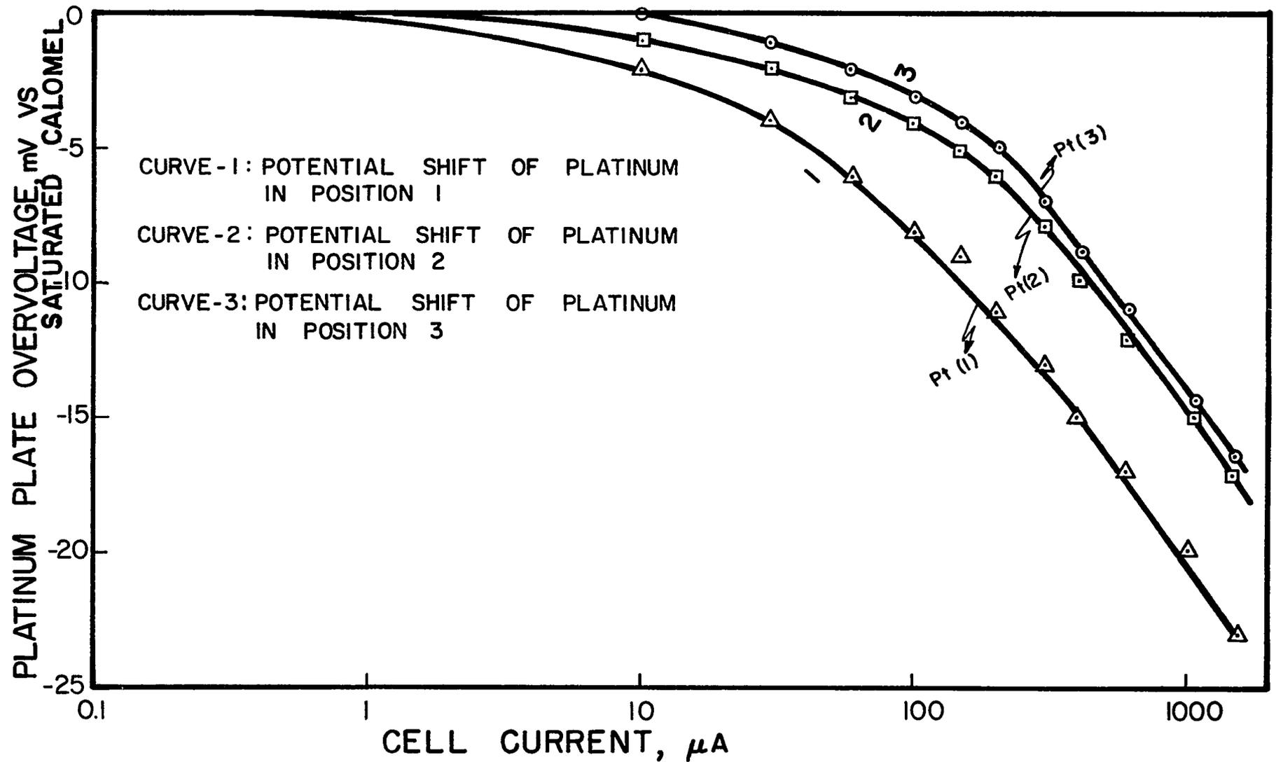
FIG. 39. POTENTIAL SHIFT OF PLATINUM ELECTRODES AS A RESULT OF CATHODIC POLARIZATION OF CATHODE IN 3% SALT SOLUTION.
