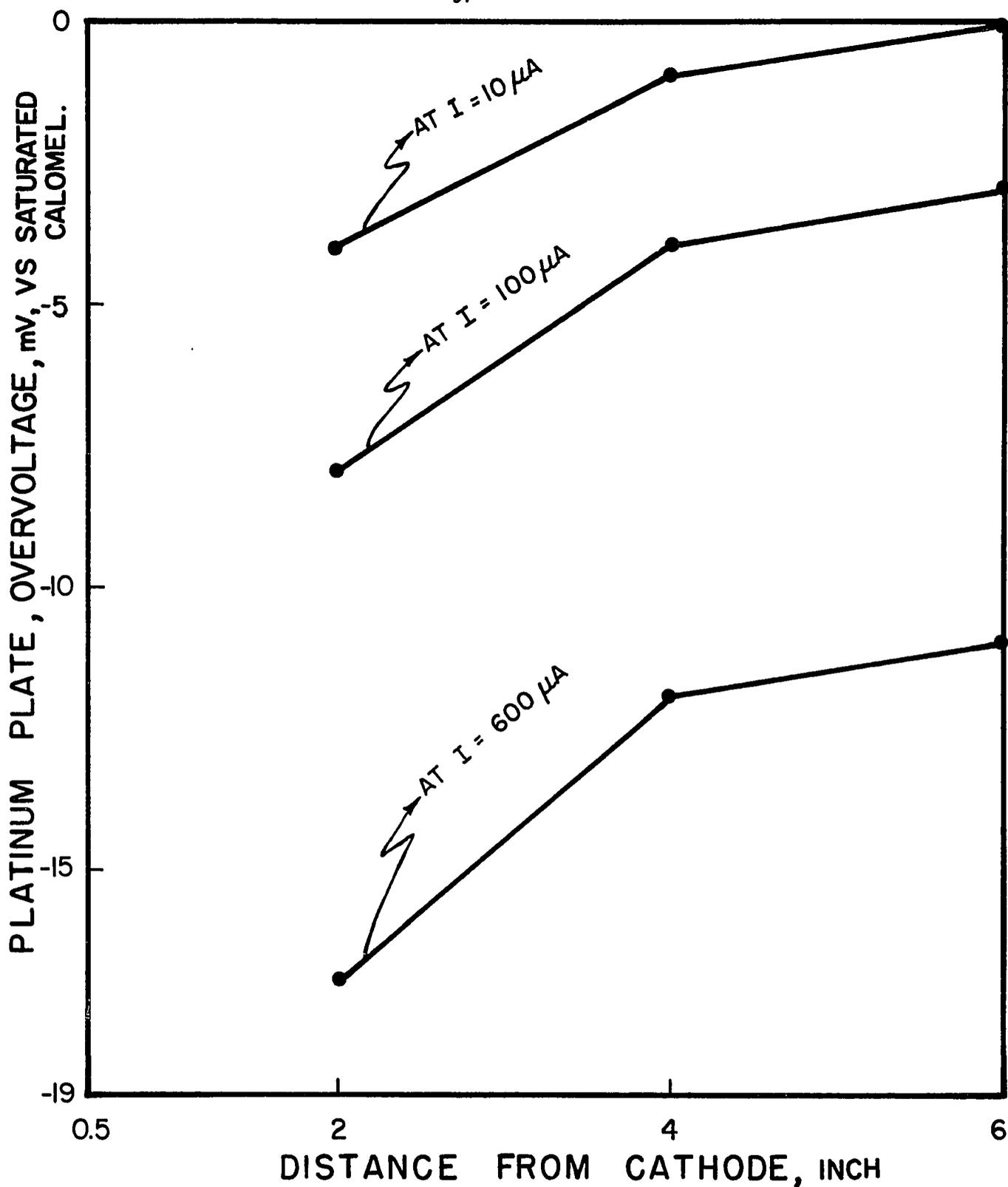
FIG. 40. POTENTIAL SHIFT OF PLATINUM PLATE BETWEEN ANODE AND CATHODE AS A FUNCTION OF DISTANCE AT THREE LEVELS OF CATHODIC CURRENT IN 3% SALT SOLUTION.
