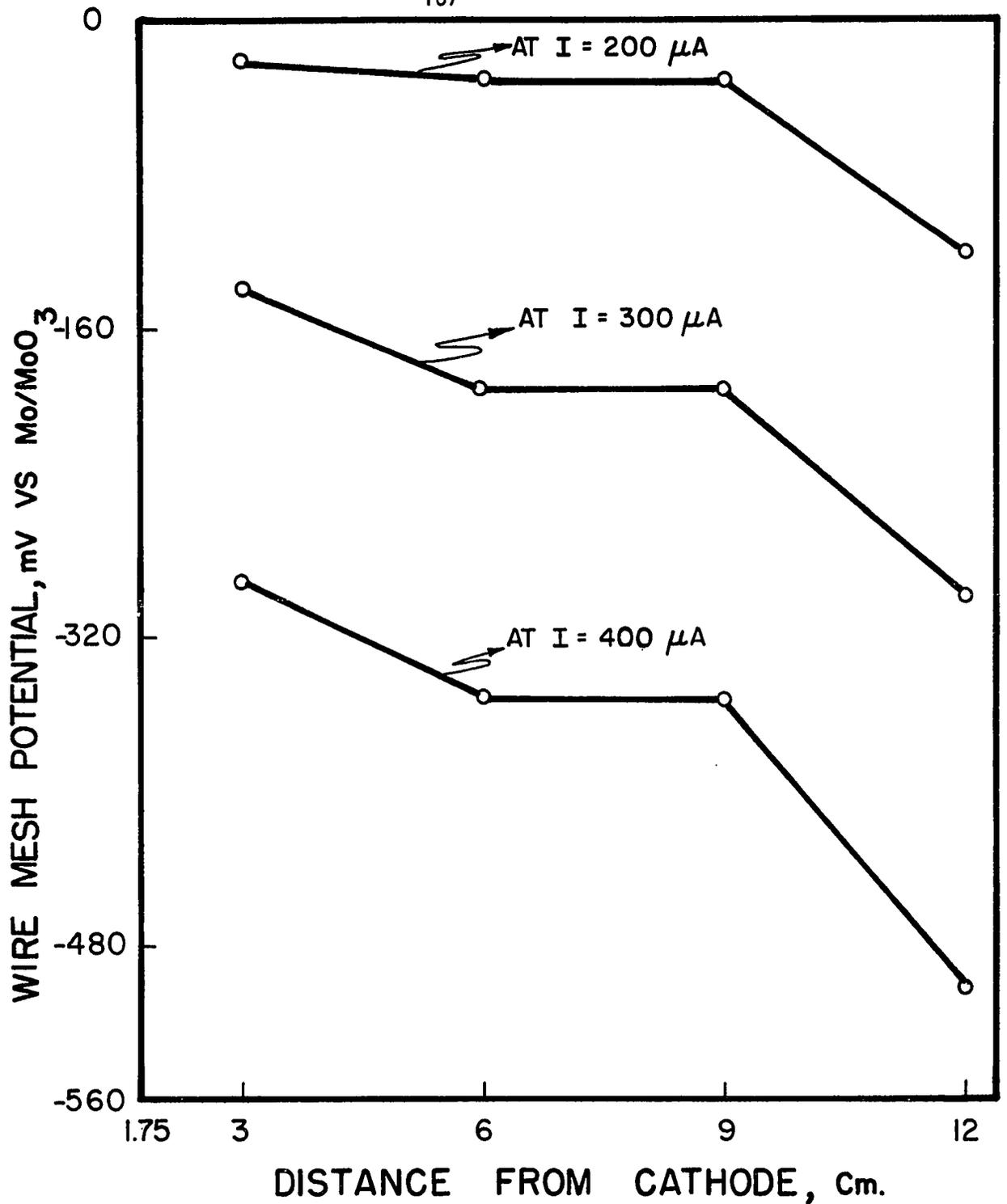
FIG. 48. POTENTIAL SHIFT OF STEEL WIRE MESH AS A FUNCTION OF DISTANCE AT THREE LEVELS OF CATHODE CURRENT FOR POLARIZATION OF STEEL PLATE IN TYPE I PORTLAND CEMENT CONCRETE.
