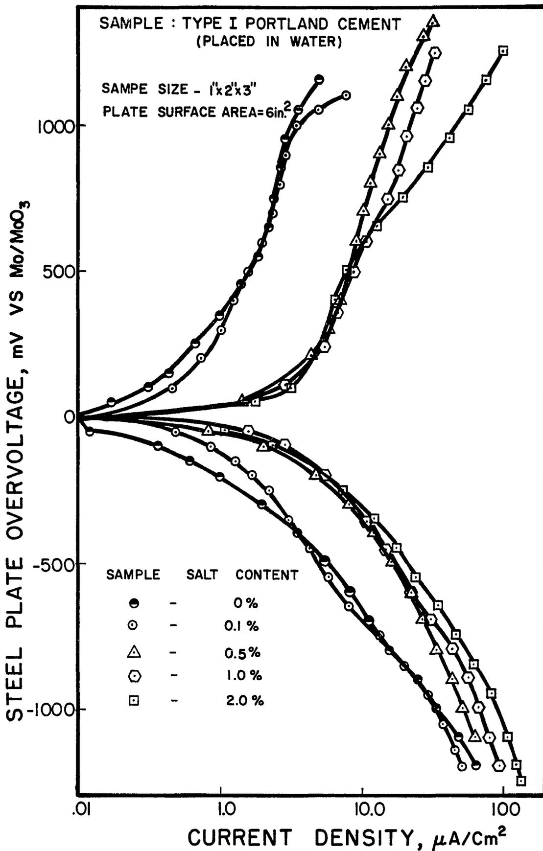
FIG. 16. ANODIC AND CATHODIC POLARIZATION OF STEEL IN TYPE I PORTLAND CEMENT CONCRETE WITH VARIOUS SALT CONTENTS. THE SAMPLES WERE IN WATER FOR 90 DAYS.
