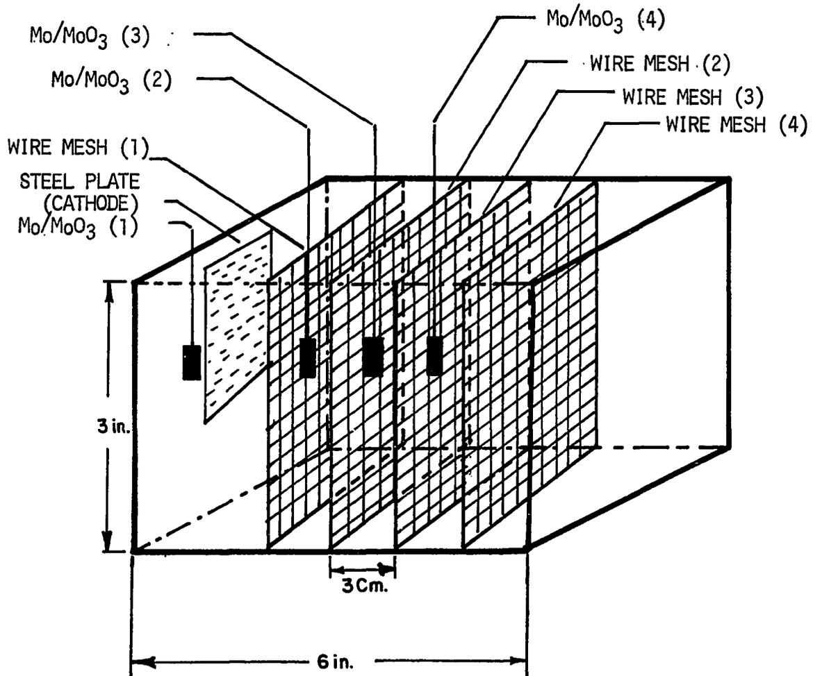
FIG. 5 . CONCRETE SAMPLE WITH ONE STEEL PLATE AND FOUR STEEL WIRE MESHES AT THE DISTANCES 4 CM APART EMBEDDED IN CONCRETE BETWEEN ANODE AND CATHODE.
