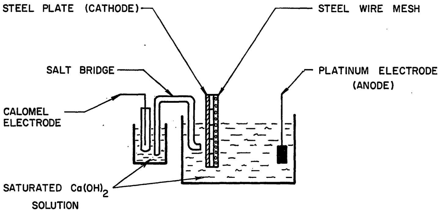
FIG. 8. CELL ASSEMBLY FOR ANODIC AND CATHODIC POLARIZATION OF STEEL PLATE WHEN WIRE MESH IS LYING ON STEEL PLATE IN SATURATED  $\text{Ca(OH)}_2$  SOLUTION.
