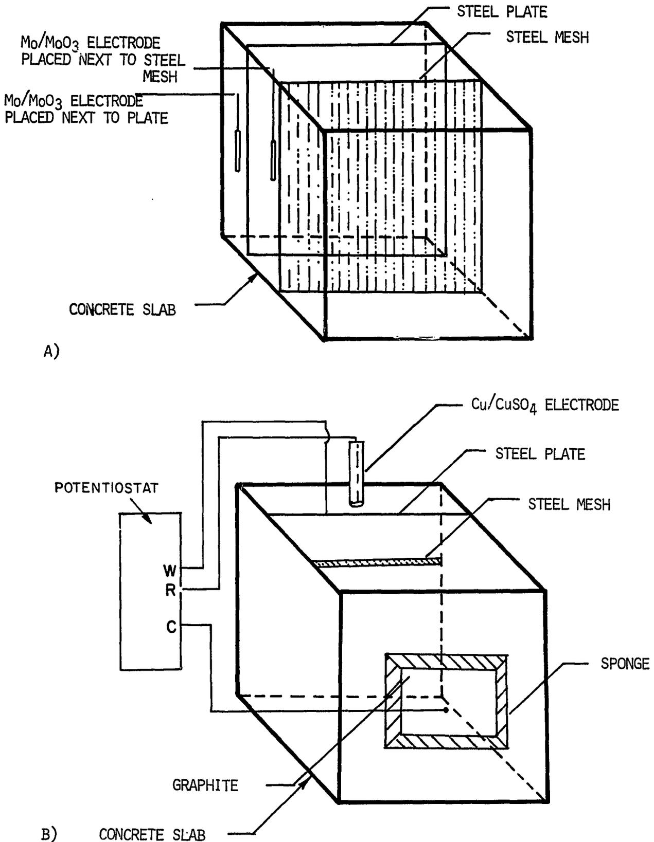
FIG. 3 . SCHEMATIC DIAGRAM OF CONCRETE SLABS FOR MESH SHIELDING STUDIES
