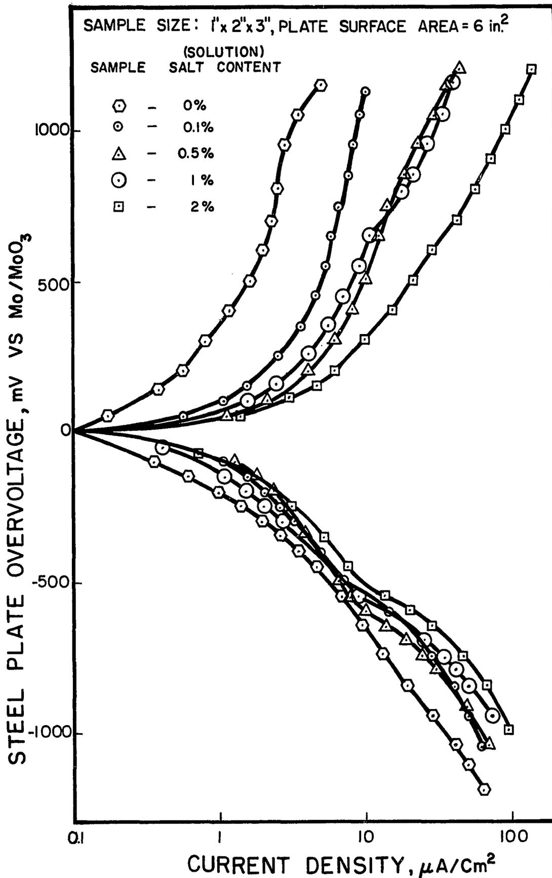
FIG. 24. ANODIC AND CATHODIC POLARIZATION OF STEEL PLATE IN CONCRETE SAMPLE OF TYPE I PORTLAND CEMENT. SAMPLES WERE IN VARIOUS SALT CONTAMINATED SOLUTIONS FOR 90 DAYS.
