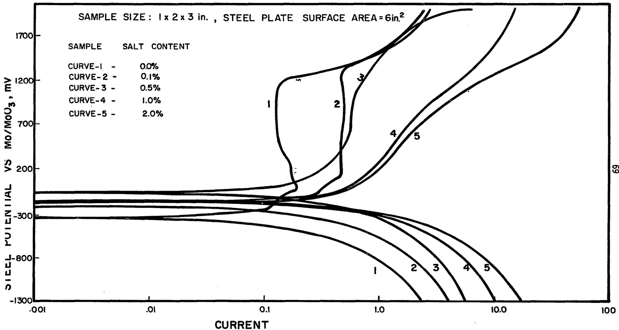
FIG. 21 . POTENTIODYNAMIC ANODIC POLARIZATION OF STEEL PLATE IN TYPE V PORTLAND CEMENT CONCRETE CONTAINING VARIOUS PERCENTAGES OF SALT (NaCl). SAMPLES WERE IN DISTILLED WATER FOR 300 DAYS. [SWEEP RATE = 0.28 MV/SEC.]
