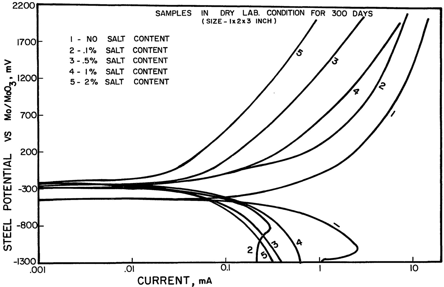
FIG. 12. POTENTIODYNAMIC ANODIC POLARIZATION OF STEEL PLATE IN TYPE I PORTLAND CEMENT CONCRETE CONTAINING VARIOUS PERCENTAGES OF SALT (NaCl) (SWEEP RATE 0.28 mV/S)
