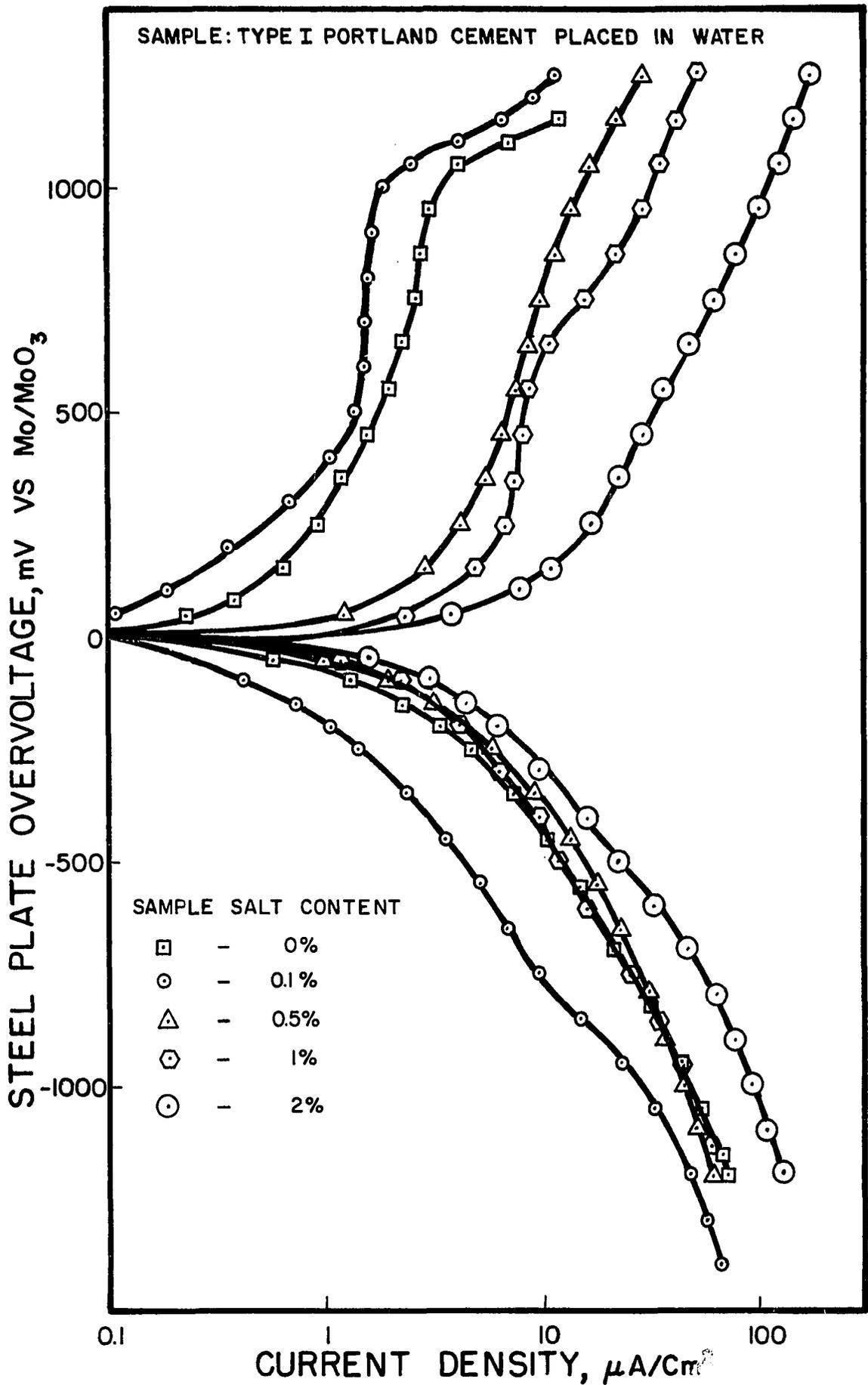
FIG. 18. ANODIC AND CATHODIC POLARIZATION OF STEEL IN TYPE I PORTLAND CEMENT CONCRETE WITH VARIOUS SALT CONTENTS. THE CONCRETE SAMPLES WERE IN WATER FOR 170 DAYS.
