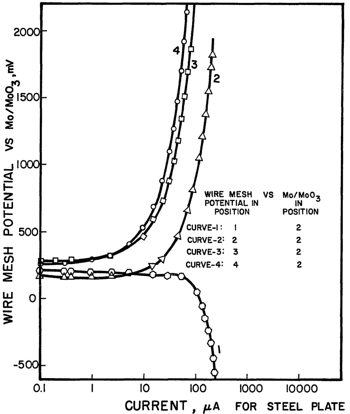
FIG. 52. SHIFT IN STEEL WIRE MESH POTENTIAL AS A FUNCTION OF CURRENT REQUIRED FOR CATHODIC POLARIZATION OF STEEL PLATE.
