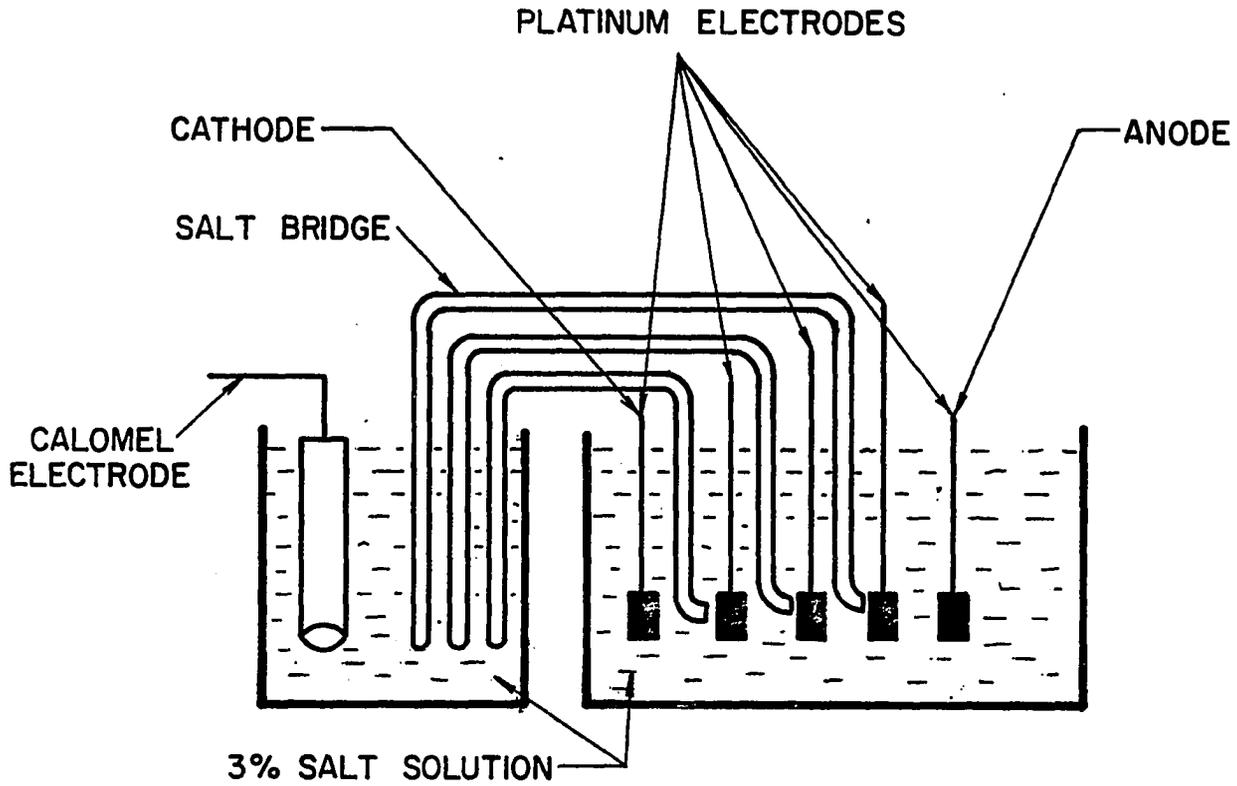
FIG. 10. CELL ASSEMBLY FOR ANODIC AND CATHODIC POLARIZATION OF PLATINUM ELECTRODE AND ITS EFFECT ON THREE OTHER PLATINUM ELECTRODES PLACED BETWEEN ANODE AND CATHODE IN 3% SALT SOLUTION.
