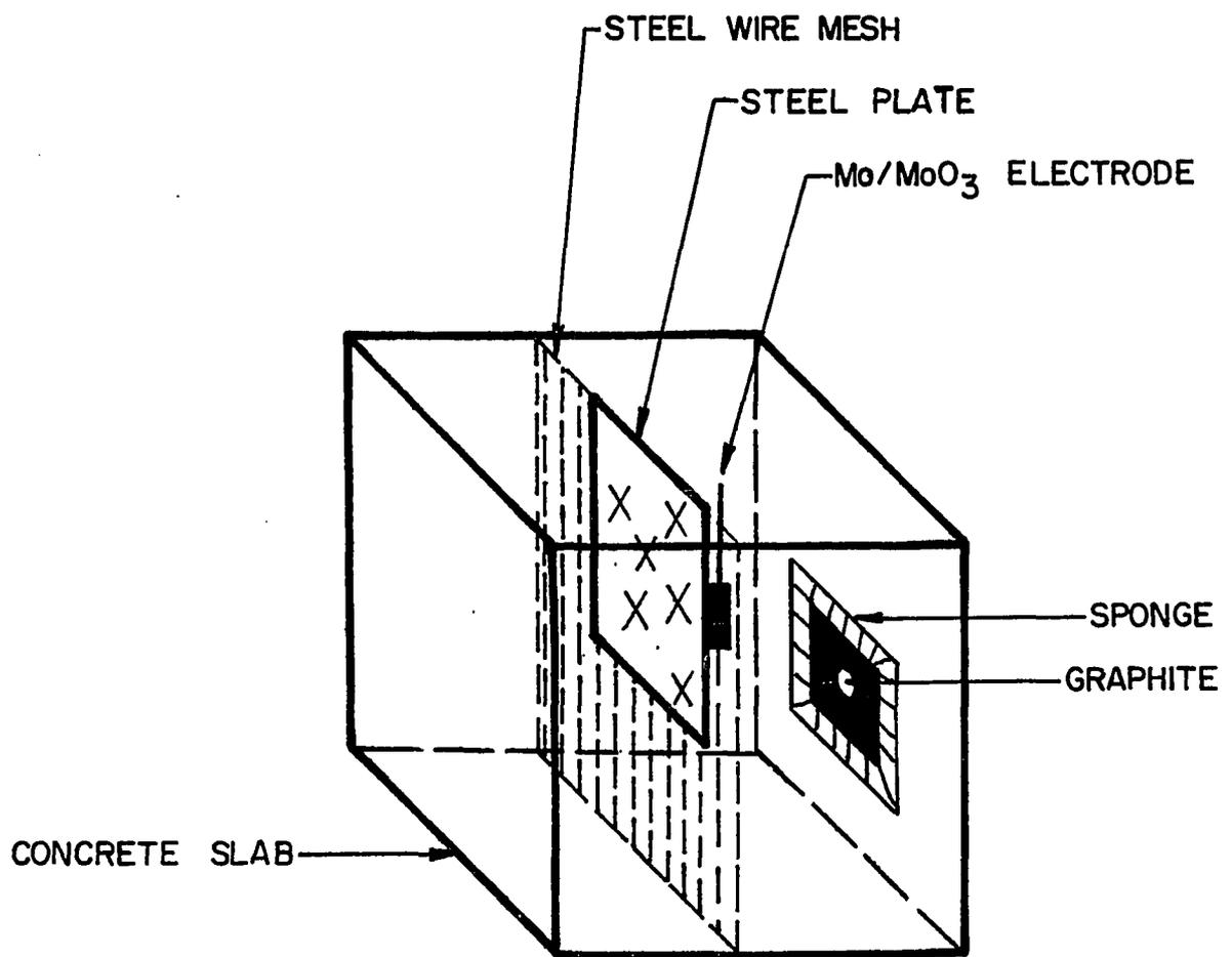
FIG. 4. CELL ASSEMBLY FOR CONCRETE SLAB
