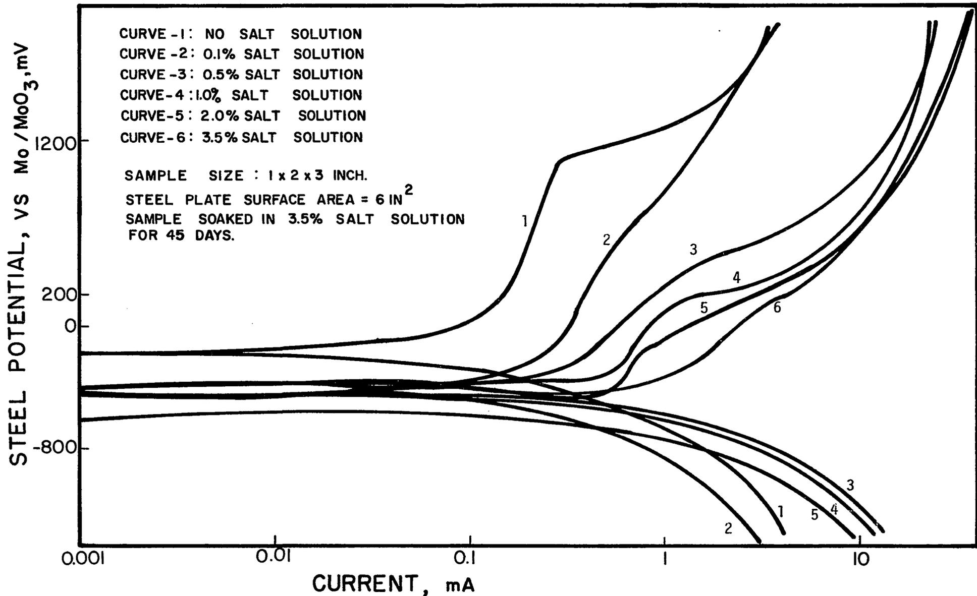
FIG. 27. POTENTIO — DYNAMIC ANODIC POLARIZATION OF STEEL PLATE IN TYPE I PORTLAND CEMENT CONCRETE PLACED IN VARIOUS SALT CONCENTRATED SOLUTIONS FOR 300 DAYS. ( SWEEP RATE - 0.28 mV/S )
