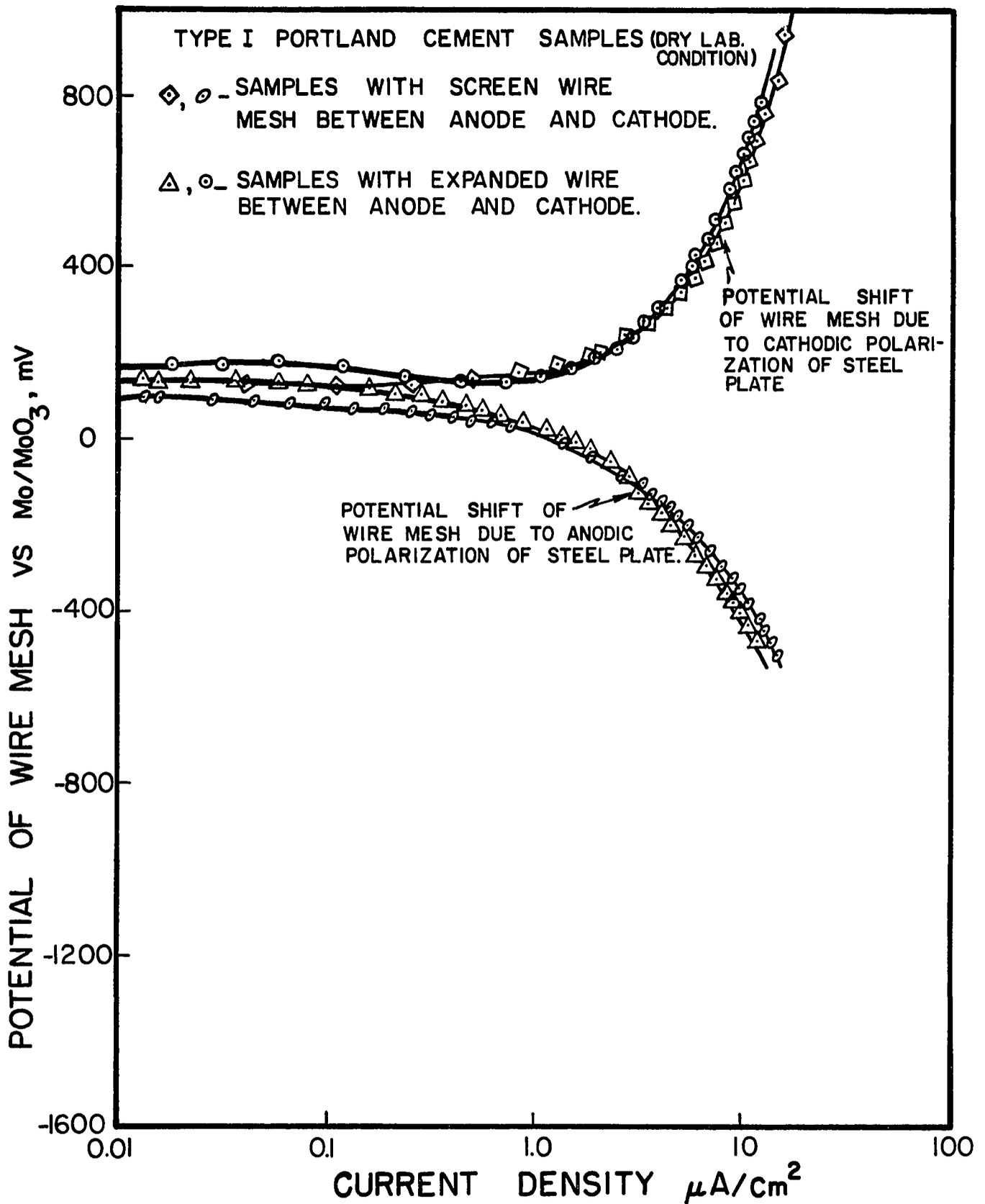
FIG. 44. POTENTIAL SHIFT OF WIRE MESH IN TYPE I PORTLAND CEMENT CONCRETE DURING ANODIC AND CATHODIC POLARIZATION OF STEEL PLATE.
