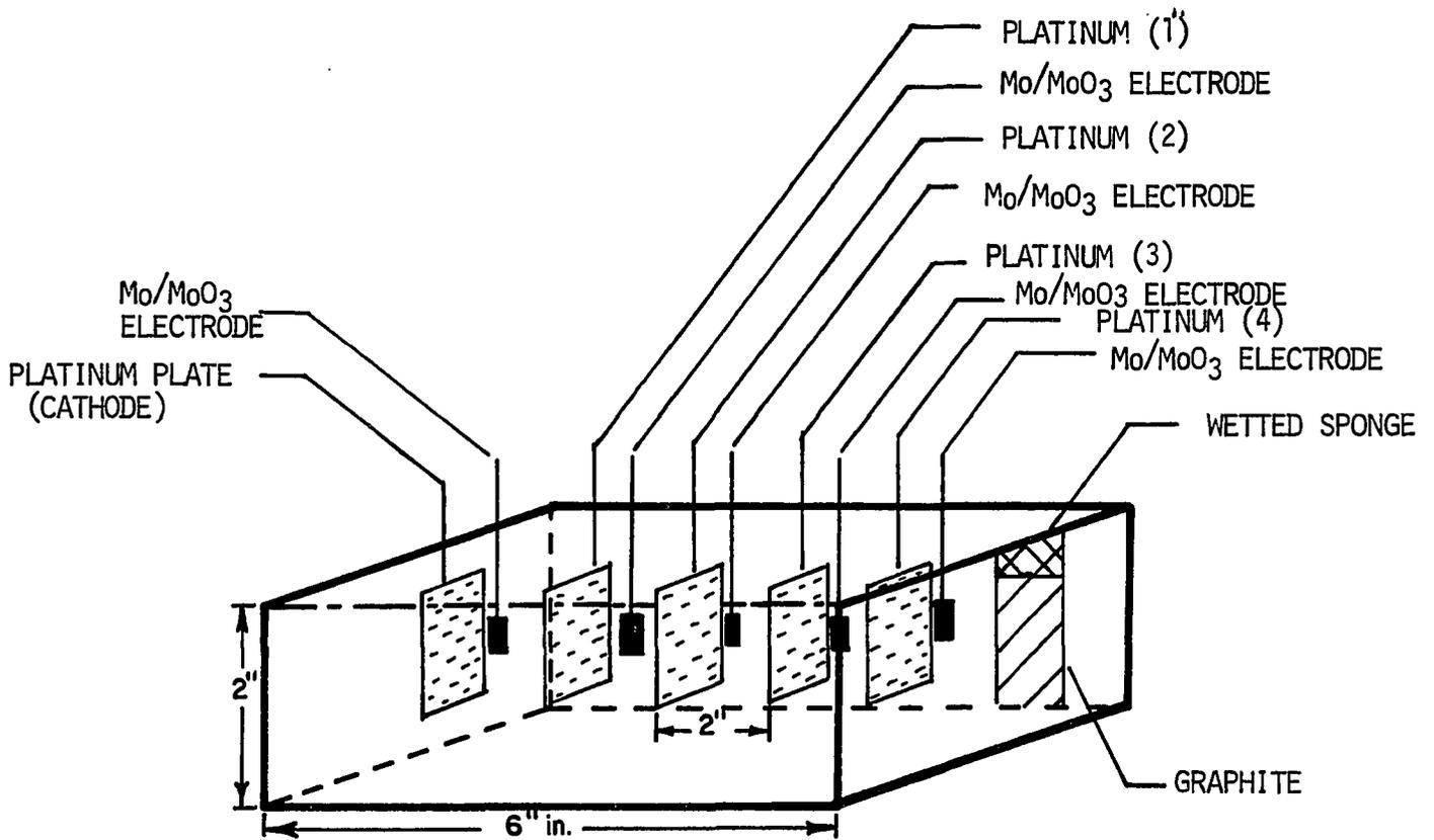
FIG. 6 . CONCRETE SAMPLE WITH FIVE PLATINUM PLATES AND FIVE Mo/MoO<sub>3</sub> ELECTRODES ADJACENT TO PLATES. PLATINUM PLATES ARE AT THE DISTANCE OF 2 INCHES APART FROM ONE ANOTHER.
