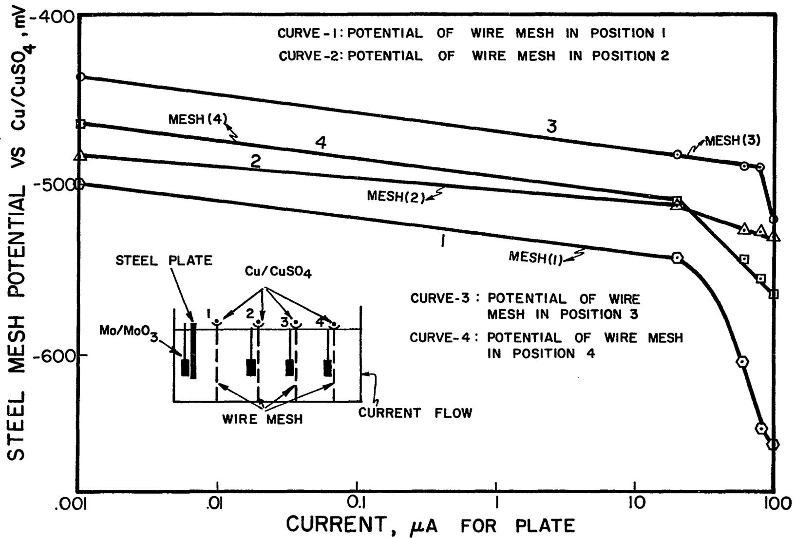
FIG. 49. POTENTIAL SHIFT OF WIRE MESH COMPARED TO  $\text{Cu}/\text{CuSO}_4$  AS A RESULT OF CATHODIC POLARIZATION OF STEEL PLATE.
