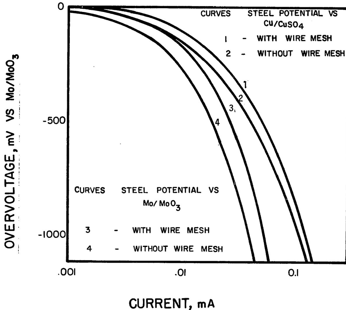
FIG. 43. POTENTIODYNAMIC CATHODIC POLARIZATION OF STEEL PLATE IN CONCRETE WITH RESPECT TO EXTERNAL (Cu/CuSO<sub>4</sub>) AND EMBEDDED (Mo/MoO<sub>3</sub>) REFERENCE ELECTRODES WITH AND WITHOUT PRESENCE OF WIRE MESH. SAMPLES WERE IN DRY CONDITION OF LABORATORY FOR 120 DAYS. [SWEEP RATE = 1 MV/SEC.]
