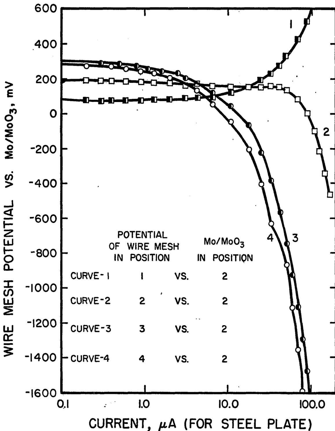
FIG. 53. SHIFT IN WIRE MESH POTENTIAL AS A FUNCTION OF CURRENT REQUIRED FOR ANODIC POLARIZATION OF STEEL PLATE.
