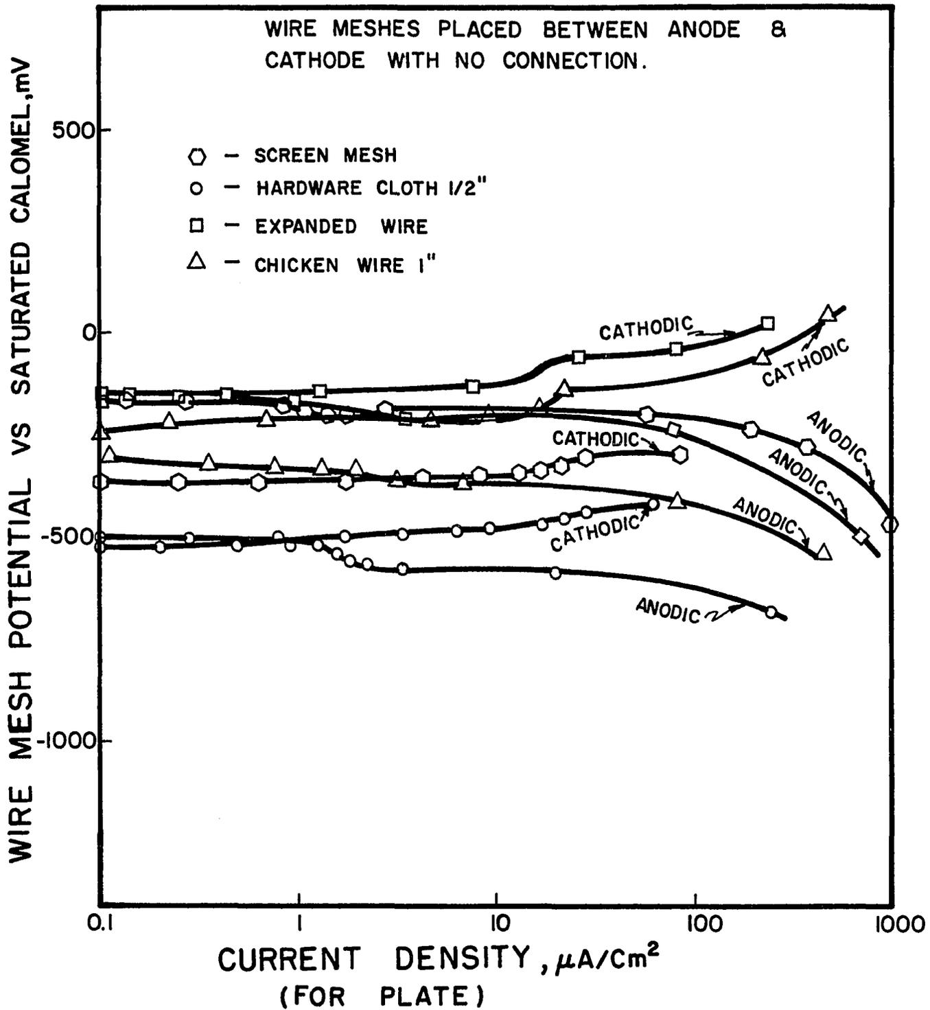
FIG. 38. POTENTIAL VARIATION OF WIRE MESH IN SATURATED  $\text{Ca}(\text{OH})_2$  DURING ANODIC AND CATHODIC POLARIZATION OF STEEL PLATE.
