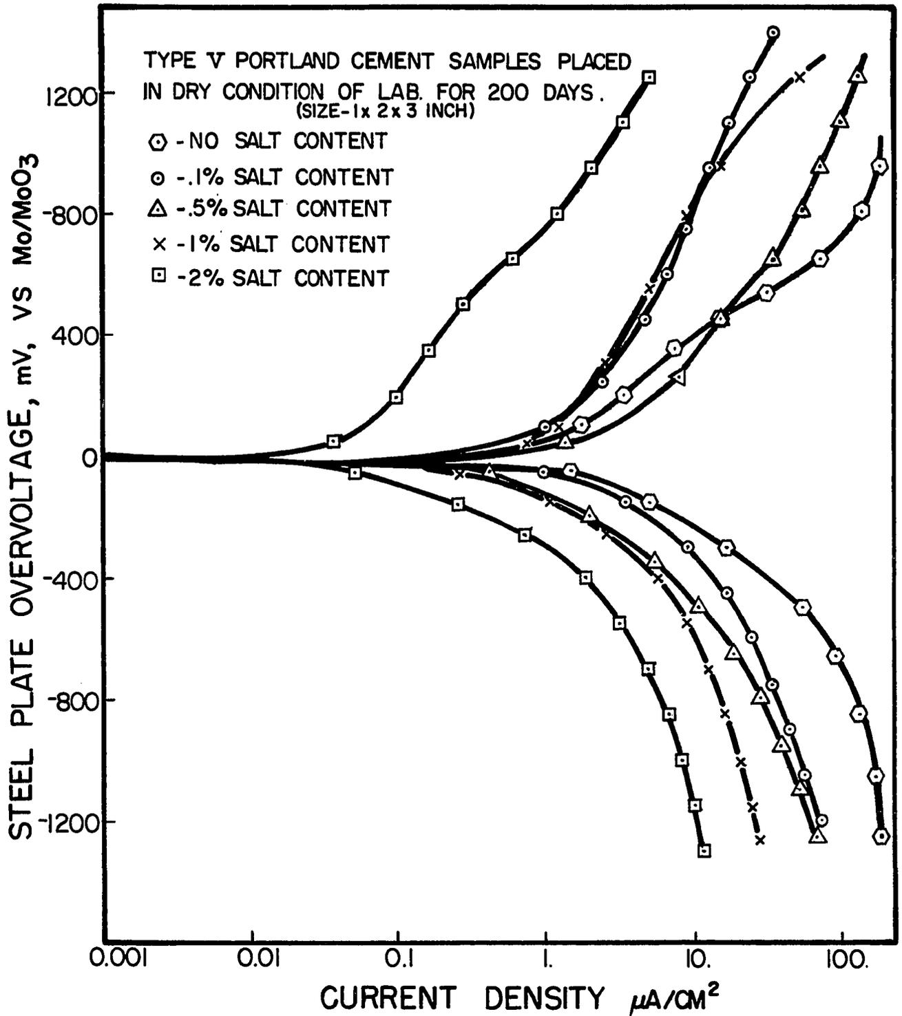
FIG. 13. ANODIC AND CATHODIC POLARIZATION OF STEEL PLATE IN TYPE V PORTLAND CEMENT CONCRETE. THE CONCRETE SAMPLES WERE IN DRY CONDITION OF LABORATORY FOR 200 DAYS.
