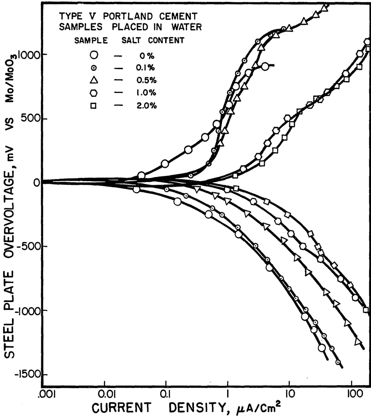
FIG. 17. ANODIC AND CATHODIC POLARIZATION OF STEEL IN TYPE V PORTLAND CEMENT CONCRETE WITH VARIOUS SALT CONTENTS. THE CONCRETE SAMPLES WERE IN WATER FOR 90 DAYS.
