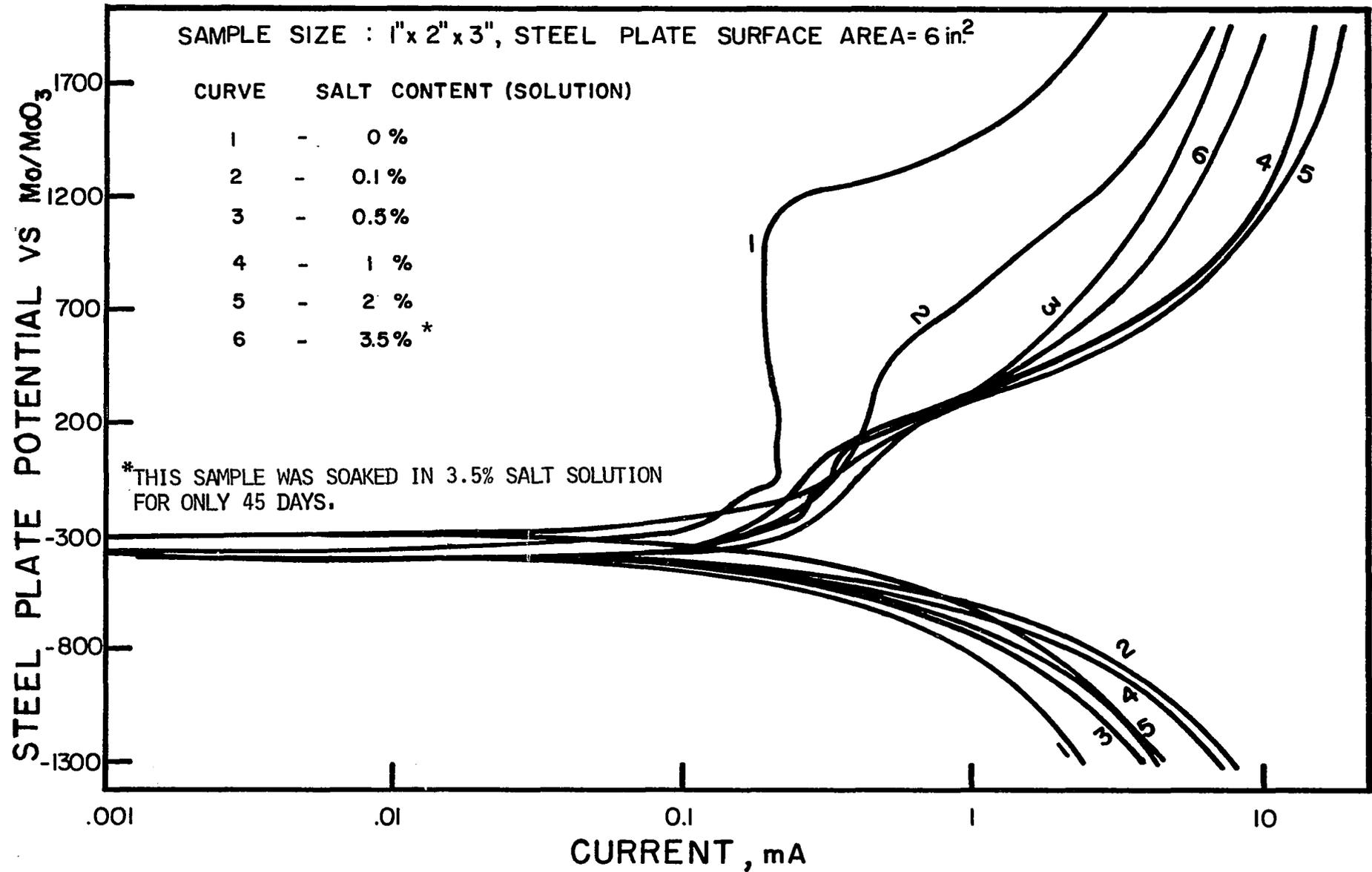
FIG. 29. POTENTIODYNAMIC ANODIC POLARIZATION OF STEEL PLATE IN TYPE V PORTLAND CEMENT CONCRETE PLACED IN VARIOUS SALT CONCENTRATED SOLUTIONS FOR 300 DAYS. [SWEEP RATE = 0.28 MV/SEC.]
