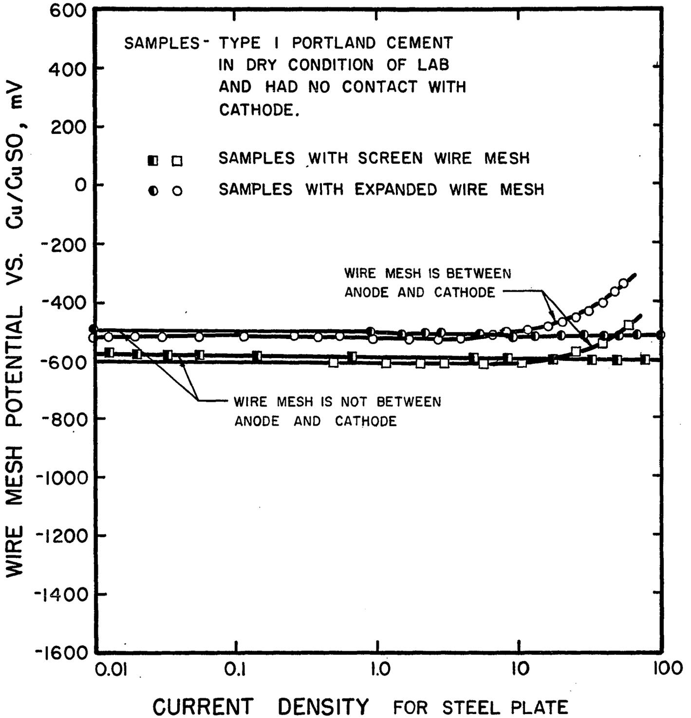
FIG. 45. POTENTIAL SHIFT OF WIRE MESH IN TYPE I PORTLAND CEMENT CONCRETE DURING CATHODIC POLARIZATION OF STEEL PLATE.
