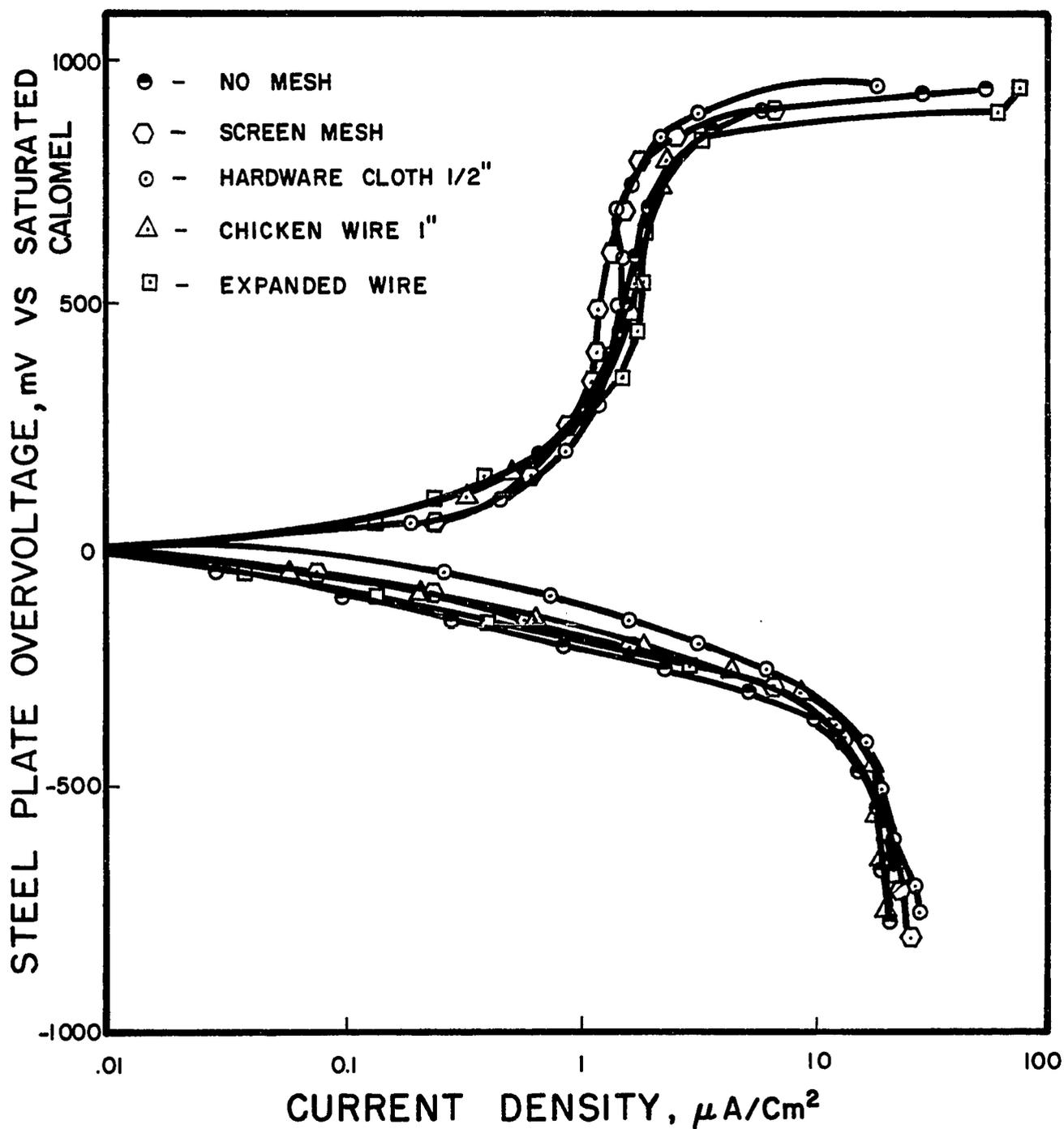
FIG. 35. ANODIC AND CATHODIC POLARIZATION OF STEEL IN SATURATED  $\text{Ca}(\text{OH})_2$  SOLUTION WITH AND WITHOUT PRESENCE OF WIRE MESH (VARIOUS SIZES). WIRE MESH WAS PLACED BETWEEN ANODE AND CATHODE WITH NO CONTACT.
