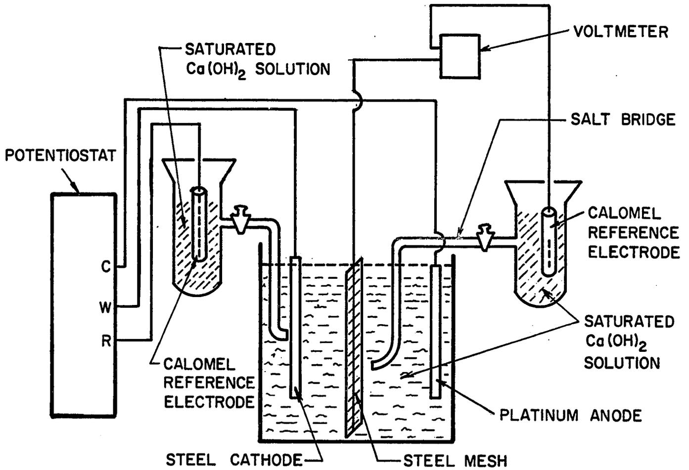
FIG. 7. EXPERIMENTAL SCHEMATIC FOR STEEL MESH STUDY.
