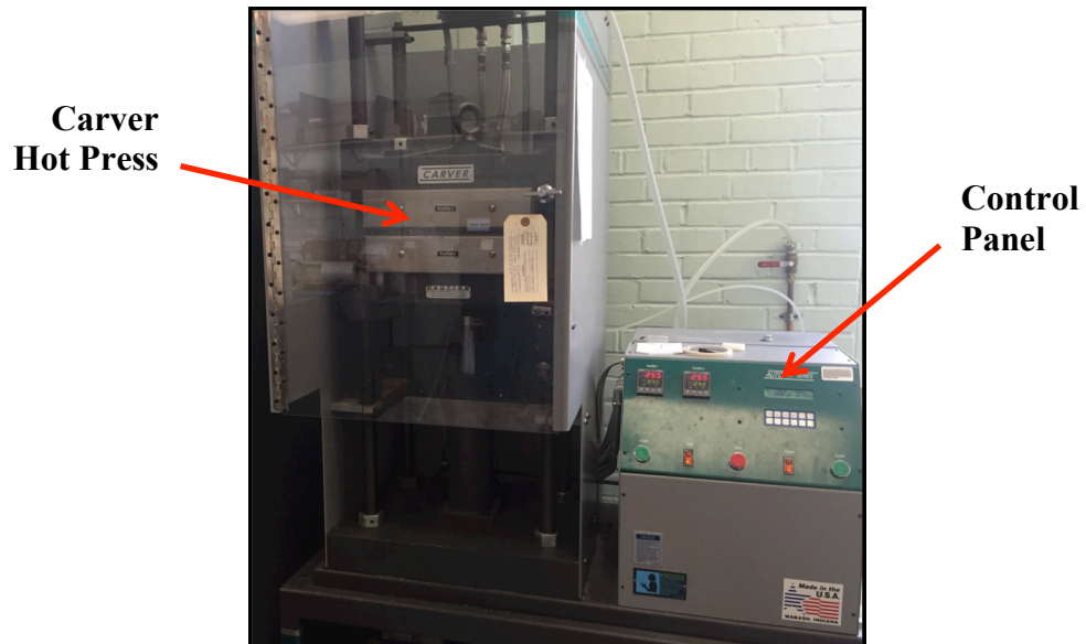
Figure 2.4 Carver hot press used for fabricating laminates from conditioned preregs
