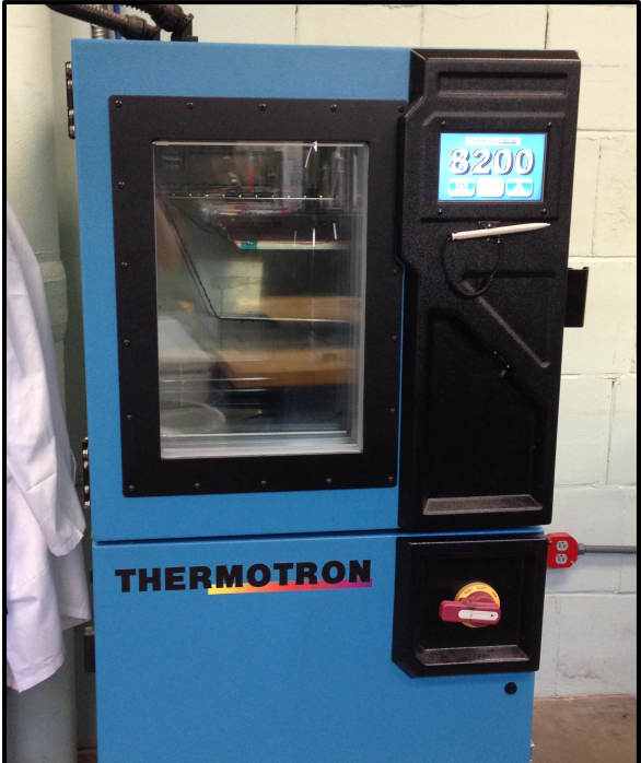
Figure 2.2 Thermotron 8200 environmental chamber used for conditioning prepreg sheets at varying relative humidity levels
