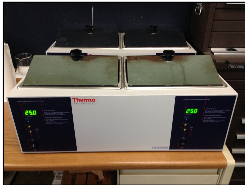
Figure 5.1 Thermo Scientific constant temperature water bath used for hydraulic fluid absorption of composite laminates
