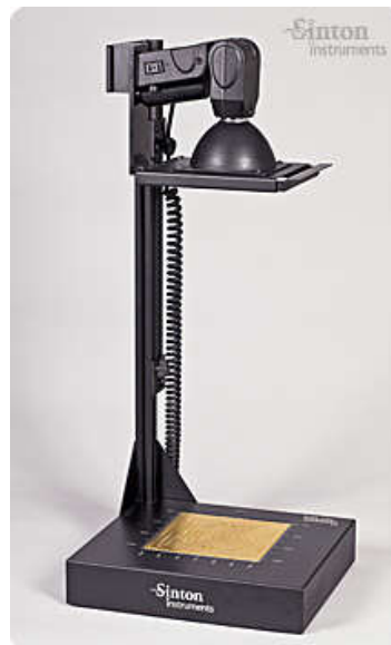
Figure 7-9: A commercial Suns- V_{oc} apparatus manufactured by Sinton instruments. Image from: http://sintoninstruments.com
