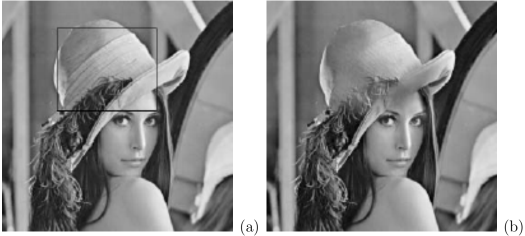
Figure 2.17: From [84], example of modulation domain filtering on amplitude modulation functions. (a) Original Lena texture image. (b) Amplitude modulation attenuation within the black rectangle of (a) to remove the bands of Lena 's hat.
