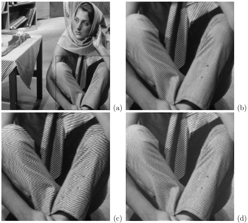
Figure 4.18: Rotation of specific texture in image. (a) Original Barbara image. Image processing is applied to the region within the black rectangle. (b) Region of interest from (a). (c) Previous result from [74]. (d) Rotated texture, using phase growing reconstruction.
