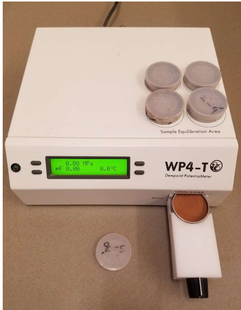
Figure 3.4: Decagon dewpoint potentiometer and soil sample cups
