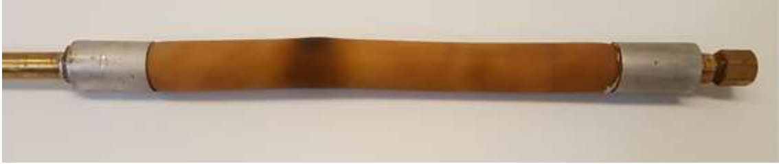
Figure 4.2: Miniature pressuremeter shown in uninflated condition
