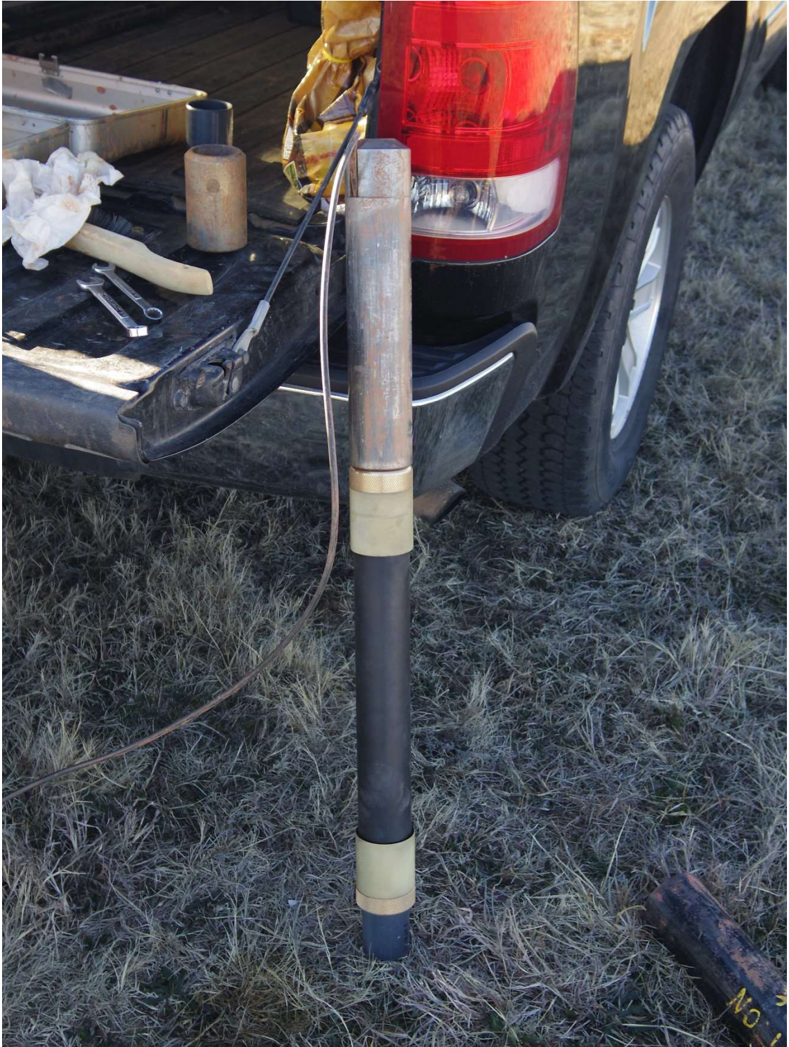
Figure 3.5: Roctest Texam NX long probe pressuremeter used for all PMT.
