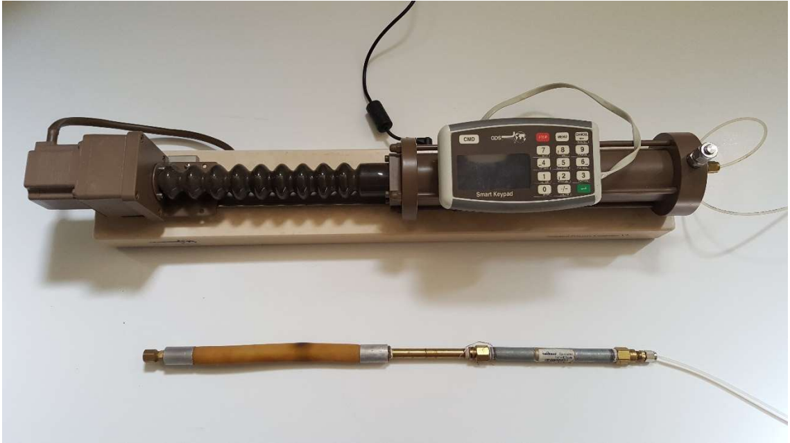
Figure 4.5: Pressure controller and miniature pressuremeter used in model footing tests
