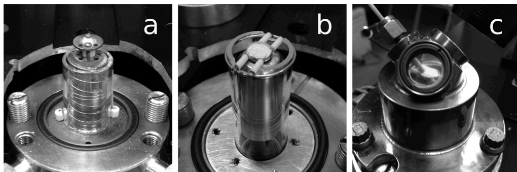
Figure 5.13 (a) Steel and (b) quartz sample holder support systems and (c) thermocouple for the quartz tube sample support system.
