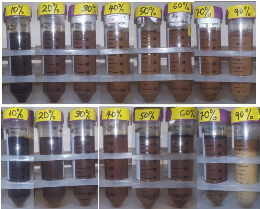
Figure 4.14: Emulsion pictures at different water fraction immediately after preparation(upper) and 48 hours after (lower)
