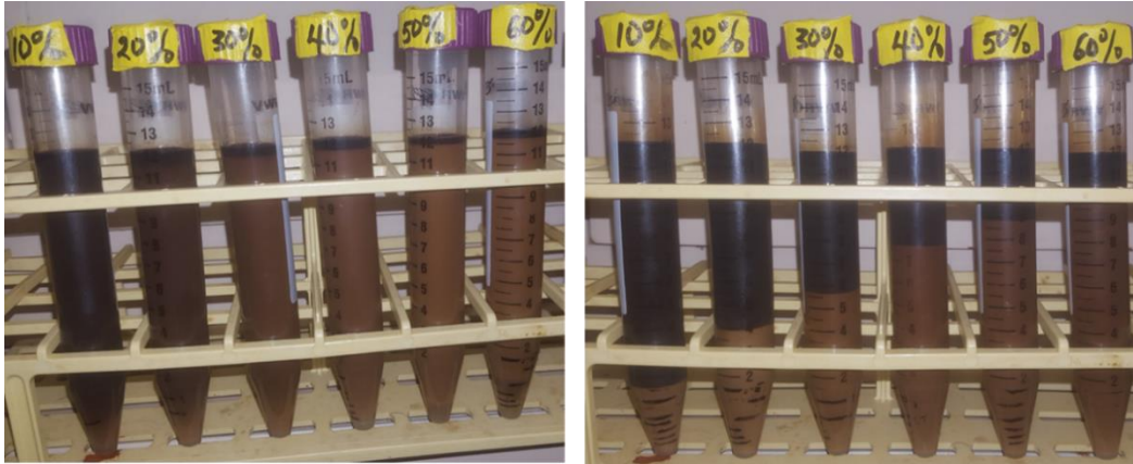
Figure 4.22: Pictures of texas crude oil emulsion after 45minutes in a centrifuge. On the left is 0.5%vol span85 and on the right is 5%vol span85 concentration
