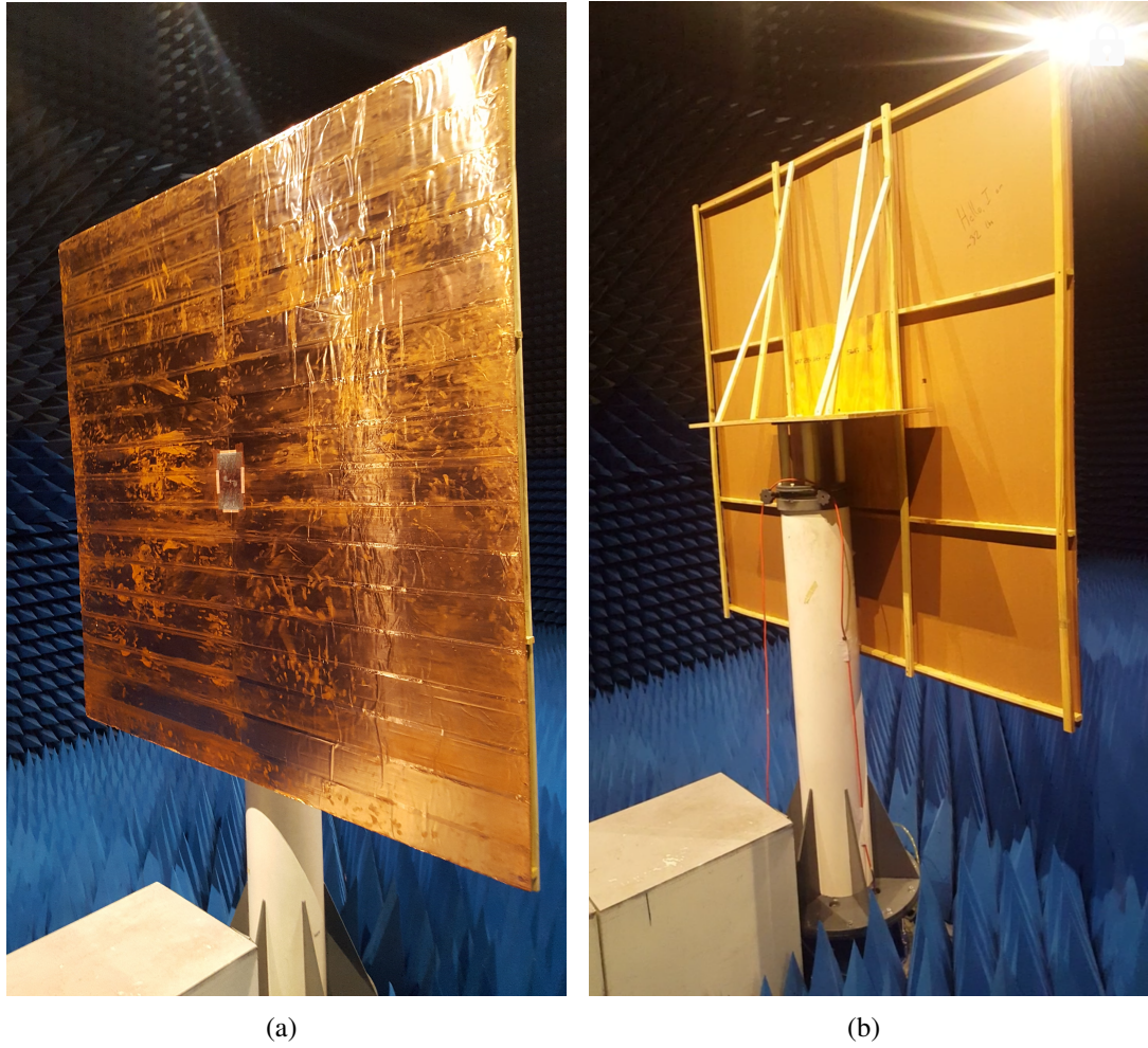
Figure 5.8: The 8'x8' ground plane mounted in the anechoic chamber.
