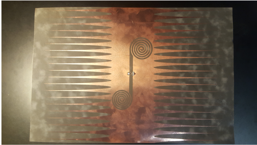
Figure 5.3: Fabricated conductor-backed slot antenna containing the curved serration edge treatment.
