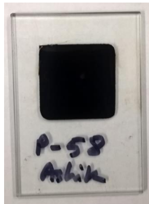
Figure 3.7 Asphalt binder sample for XRD test
