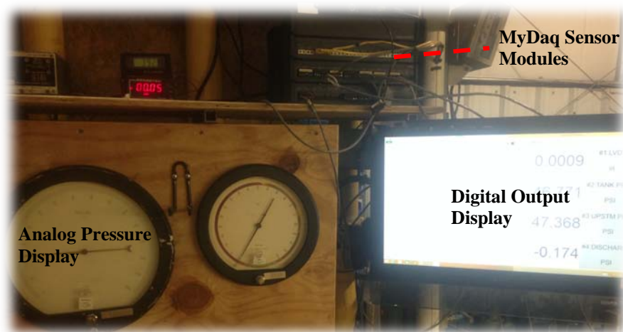
Figure 21: Data Acquisition System
