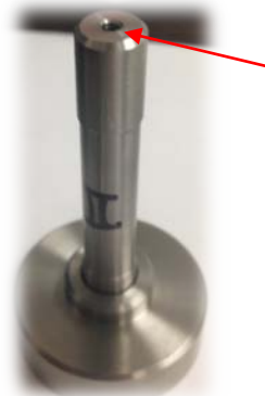
Figure 20: Disk Stem with LVDT Attachment
