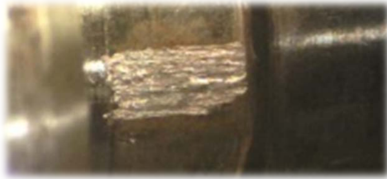
Figure 37: Galling of Component
