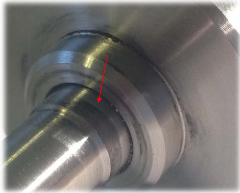
Figure 28: Low Severity Wear on Disk
