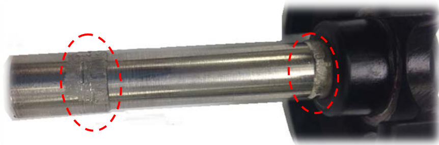
Figure 1: Galling on the piston portion of the PRV component as a result of chatter.
