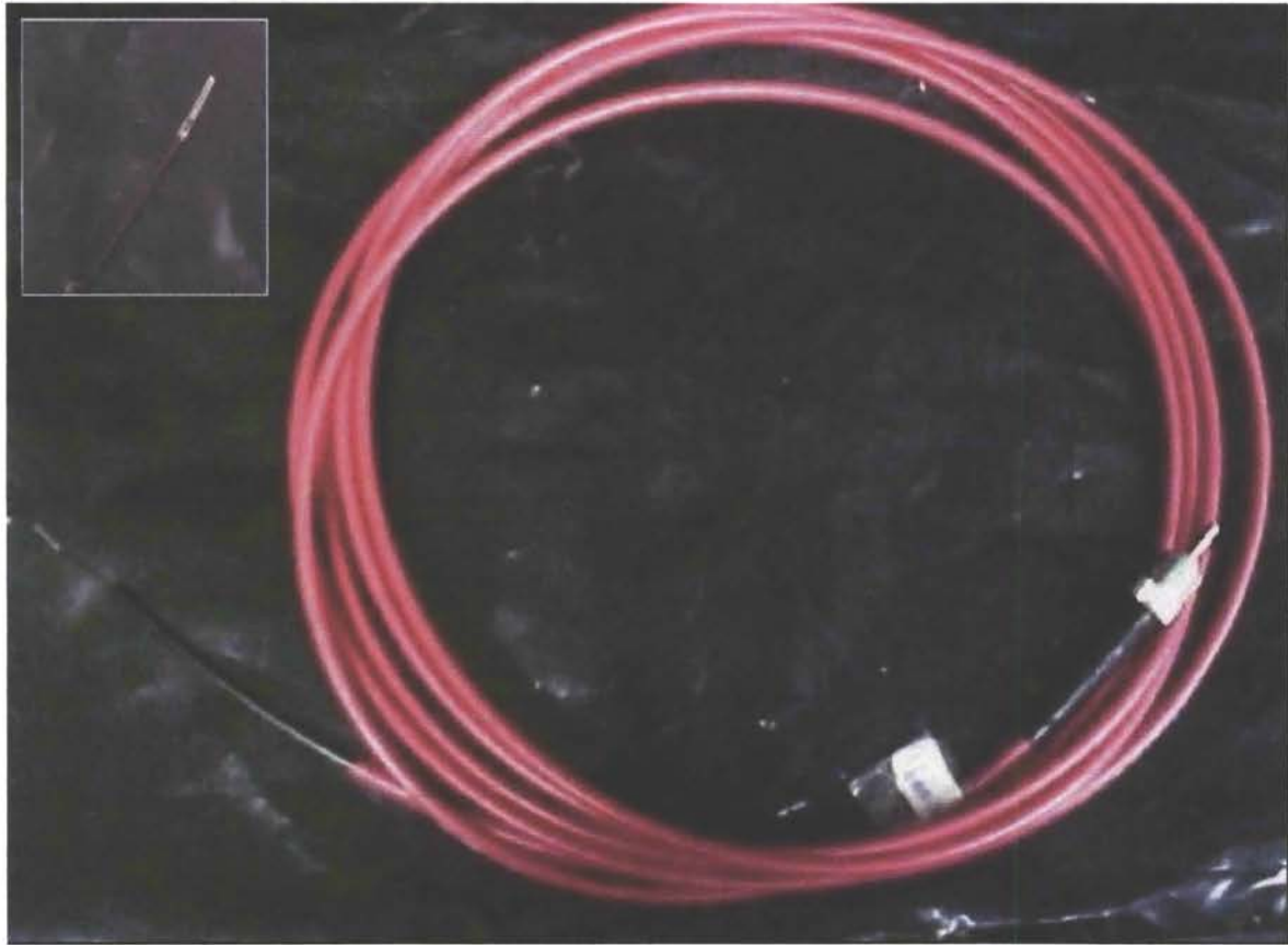
Figure 5-3: A single-fiber \text{Al}_2\text{O}_3 -based dosimeter. Pictured is a 6 mm long, 550 micron diameter piece of fiber 31 attached to a 3m fused silica fiber optic cable. A close up of the tip of the dosimeter is shown in the inset.
