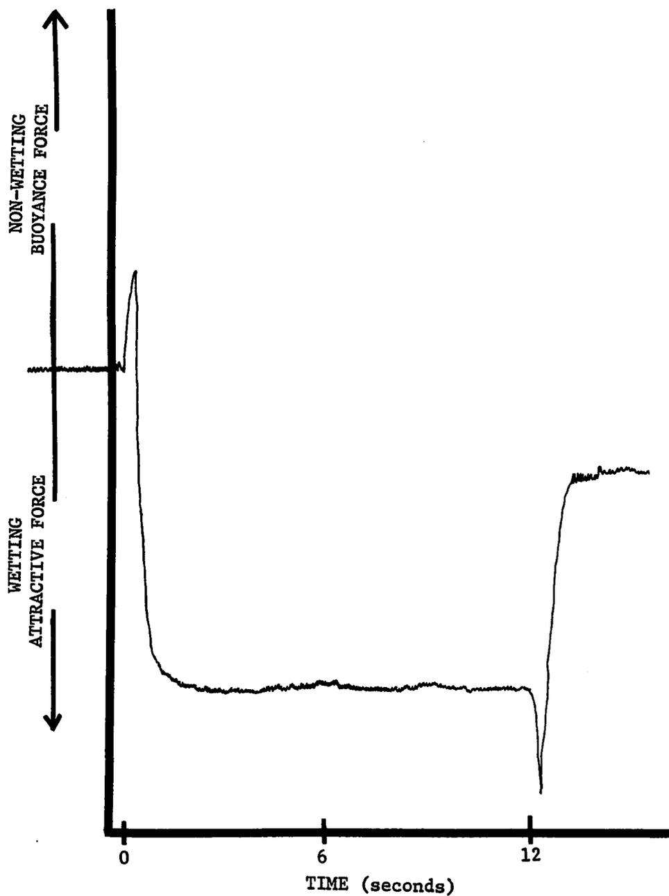
Figure B-11. A typical wetting curve. The curve is for Be-Cu soldered with 60/40 solder at 420°F (216°C).
