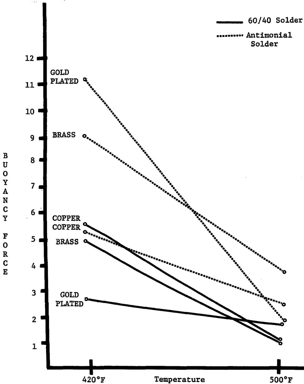
Figure B-5. Buoyancy Force vs Temperature Plot for Copper, Brass, and Gold Plated Substrates
