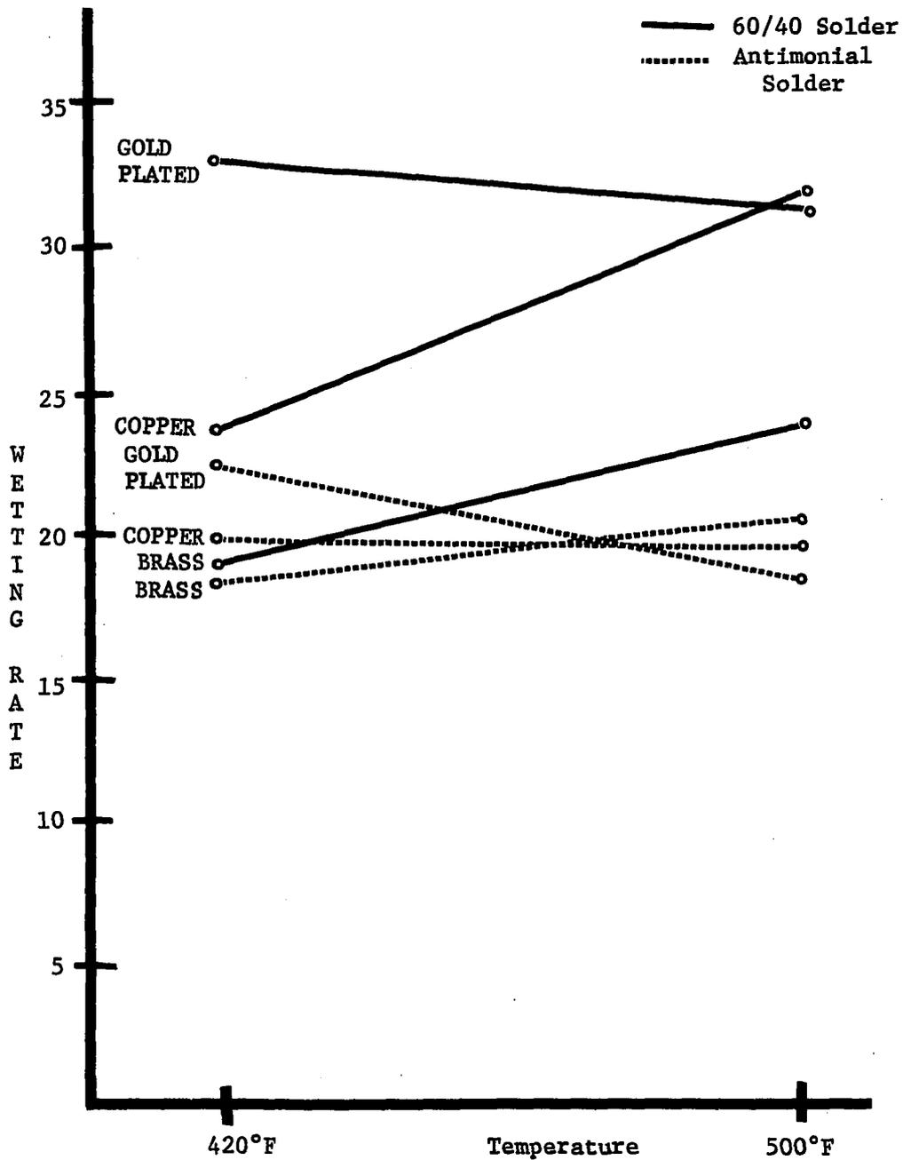
Figure B-9. Wetting Rate vs Temperature Plot for Copper, Brass, and Gold Plated Substrates
