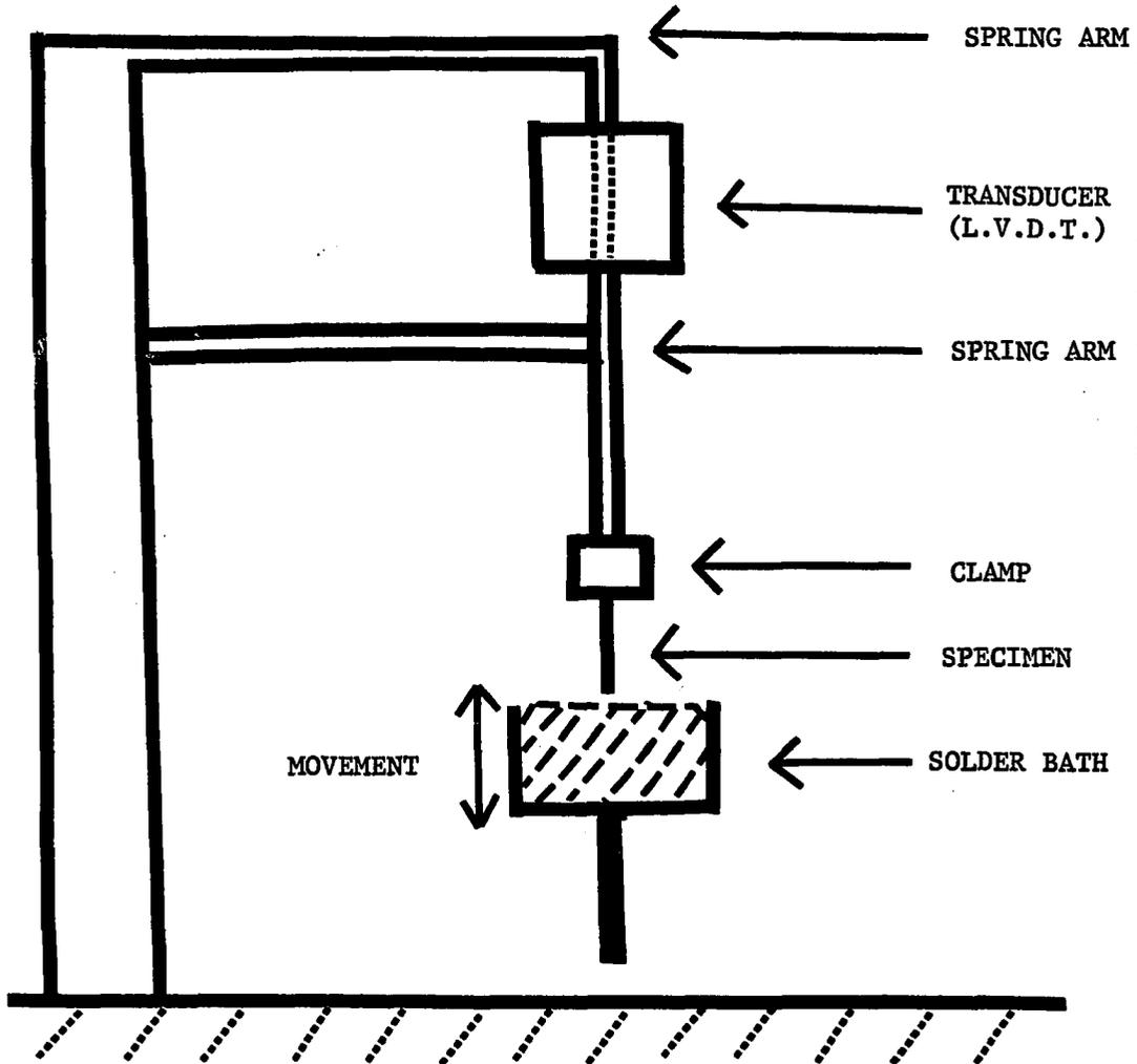
Figure B-1. The principle of operation of the G.E.C. Meniscograph
