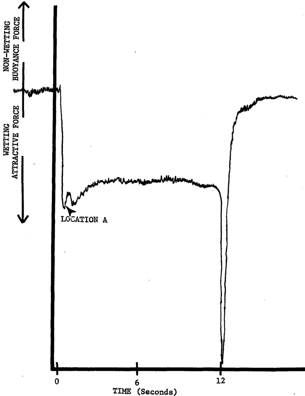
Figure B-12. Wetting curve for a gold plated terminal soldered with 60/40 solder at 500°F (260°C). Abnormal fluctuations at Location A suggest the formation of gold-tin intermetallic compounds.
