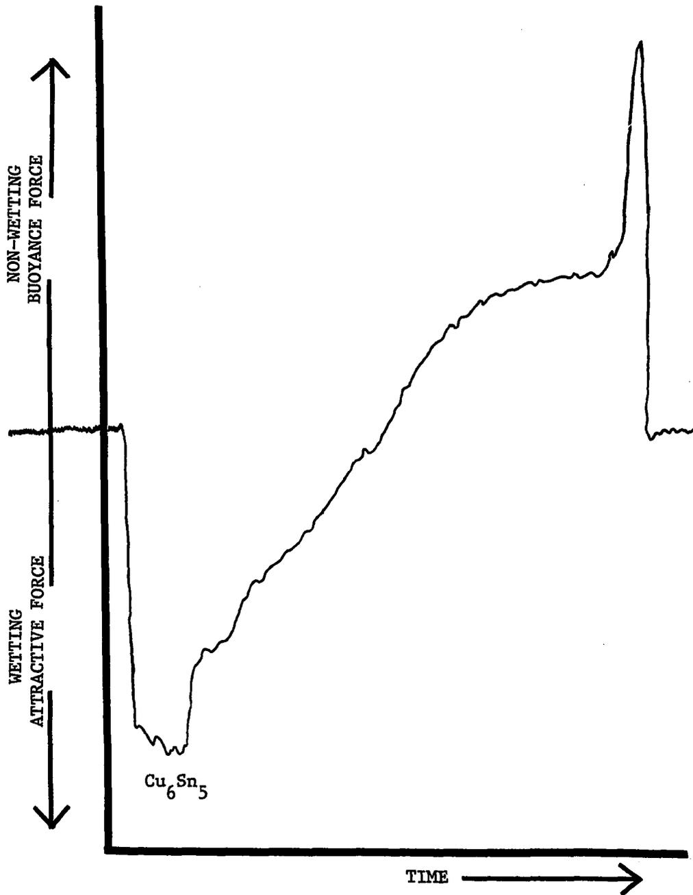
Figure B-14. The wetting curve from a study by MacKay demonstrating the wetting of  $\text{Cu}_6\text{Sn}_5$  at  $235^\circ\text{C}$ .
