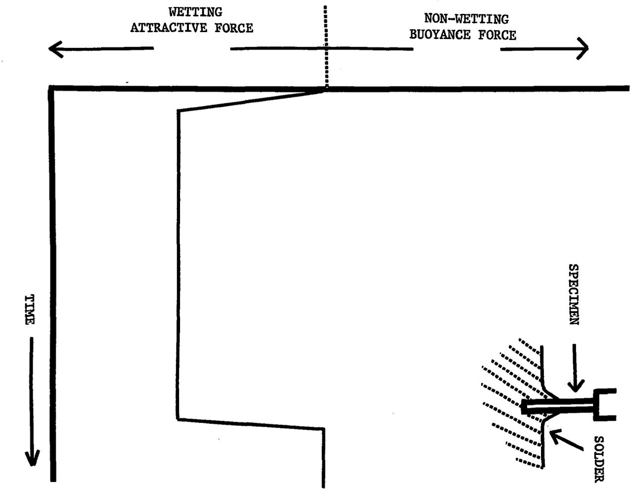
Figure B-2. Time-wetting curve for "infinite wetting"
