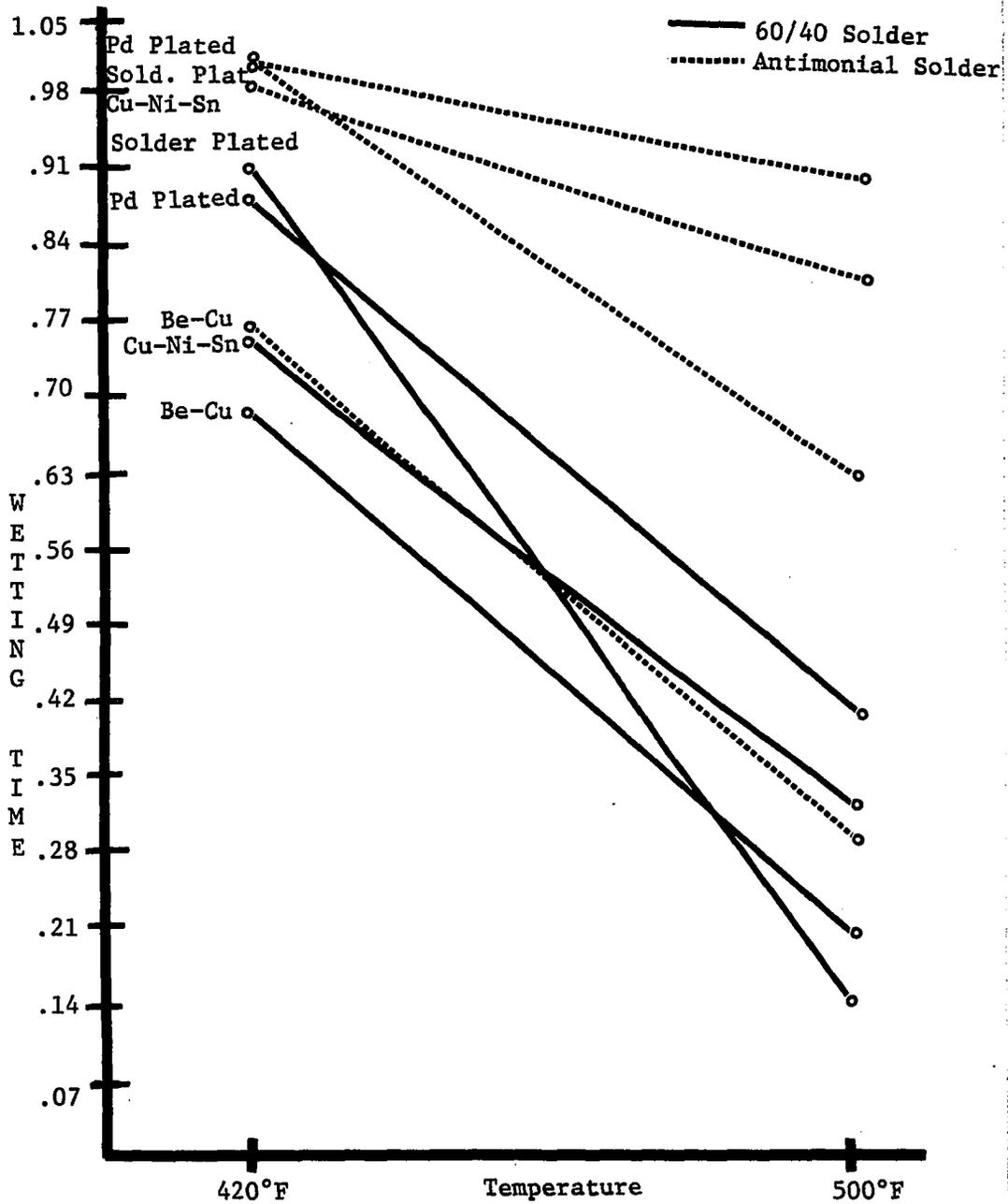
Figure B-8. Wetting Time vs Temperature Plot for Cu-Ni-Sn, Be-Cu, Pd Plated, and Solder Plated Substrates
