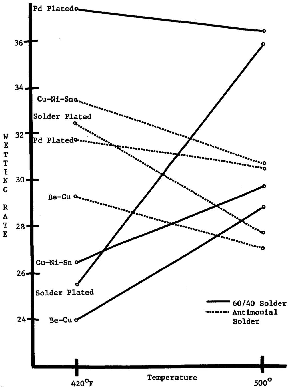
Figure B-10. Wetting Rate vs Temperature Plot for Be-Cu, Cu-Ni-Sn, Pd Plated, and Solder Plated Substrates
