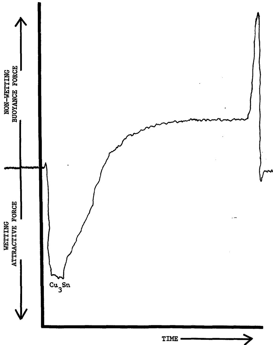
Figure B-13. The wetting curve from a study by MacKay demonstrating the wetting of  $\text{Cu}_3\text{Sn}$  at  $255^\circ\text{C}$ .
