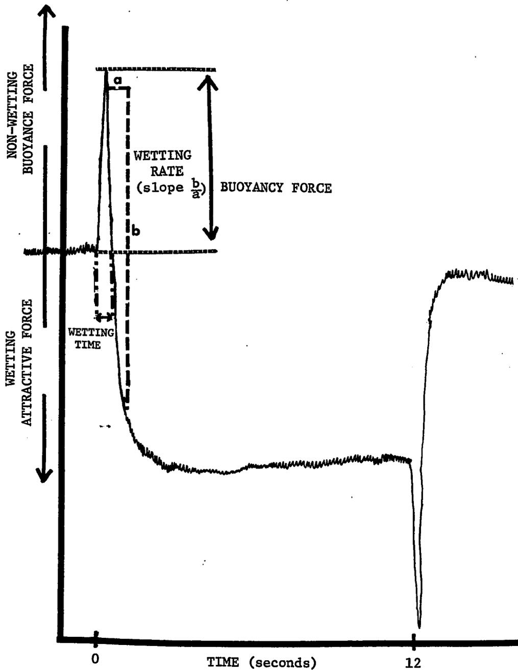
Figure B-4. A typical wetting curve generated by the soldering systems under investigation. The buoyancy force, wetting time, and wetting rate (slope  $b/a$ ) were used to evaluate the wetting characteristics of the soldering systems.
