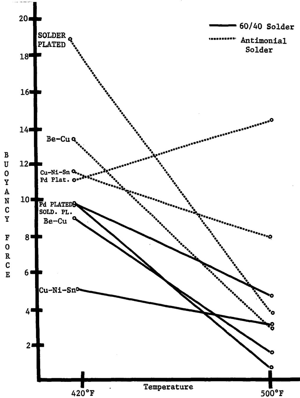
Figure B-6. Buoyancy Force vs Temperature Plot for Cu-Ni-Sn, Be-Cu, Pd Plated, and Solder Plated Substrates
