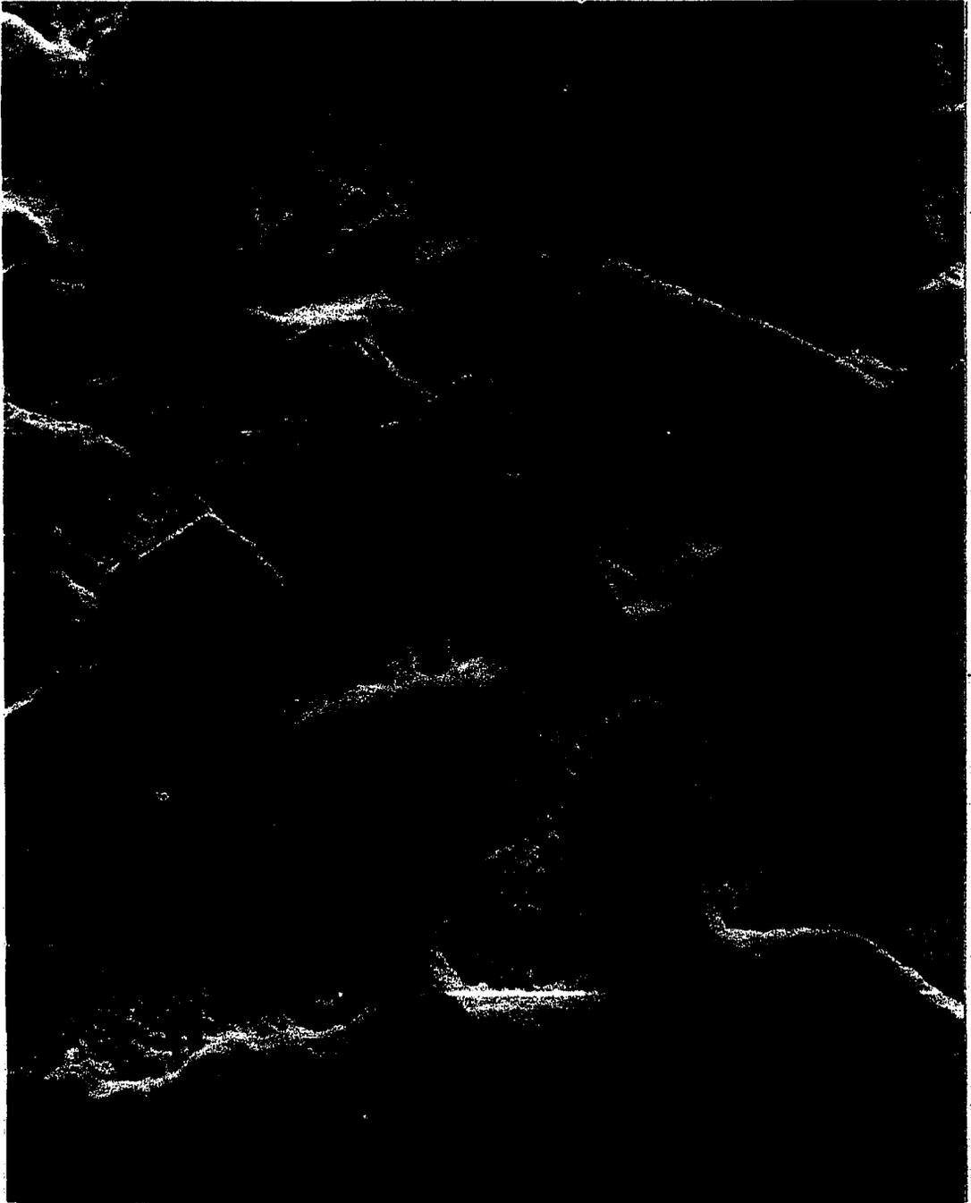
Figure 49. 4200X - Peroxide and Nital Etch
