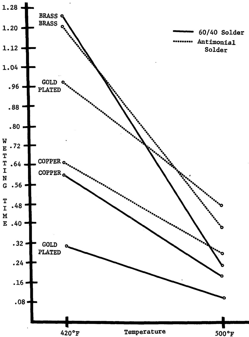
Figure B-7. Wetting Time vs Temperature Plot for Copper, Brass, and Gold Plated Substrates
