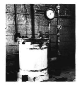
and maintained for the desired length of time. After this time, the steam was shut off and the pieces allowed to cool to room temperature before removal from the autoclave.
