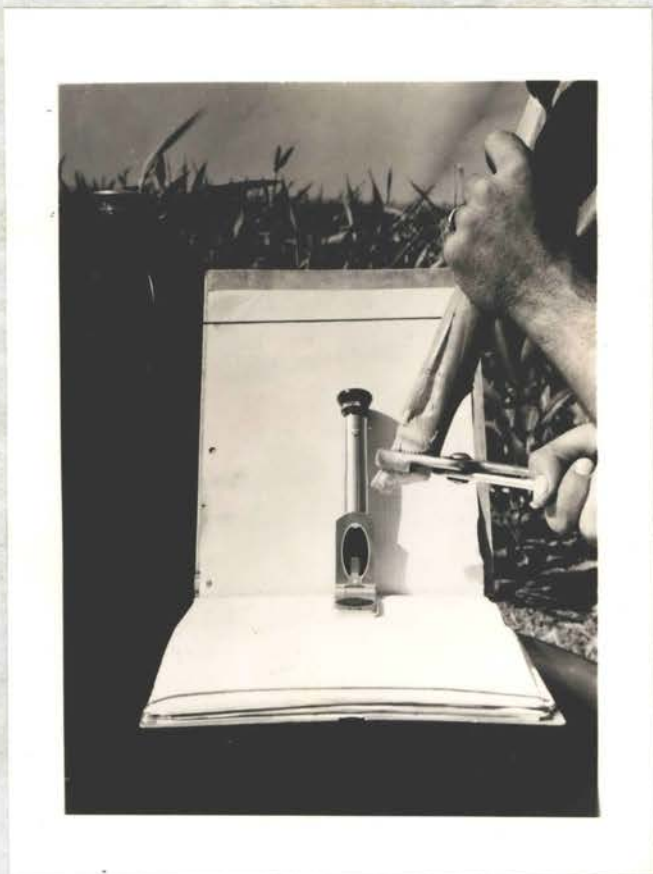
Figure 1. The process of making a reading with the refractometer
