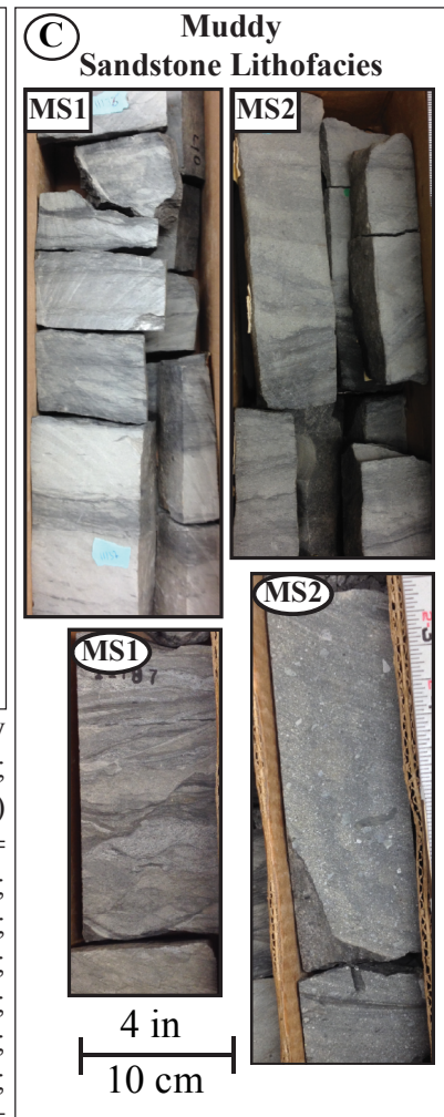
Figure 7. A) Sandstone, B) conglomerate, and C) muddy sandstone lithofacies. Circle: Core from GHK 1-27 Niece; Rectangle: Core from GHK 1-34 Finnell. S1) Parallel-stratified sandstone, measured depth (md) = 11104 ft; S2) Cross-stratified sandstone, md = 11100.5 ft; S3) Structureless sandstone, md = 11195 ft, md = 11762 ft; S4) Granule-pebble-bearing sandstone, md = 11105.5 ft; S5) Bioturbated sandstone, md = 11117 ft, md = 11692 ft; C1) Orthoconglomerate, md = 11092 ft, md = 11712.5 ft; C2) Paraconglomerate, md = 11099 ft, md = 11708 ft; MS1) Bioturbated muddy sandstone, md = 11136 ft, md = 11787 ft; MS2) Slumped muddy sandstone, md = 11086 ft, md = 11719 ft.
