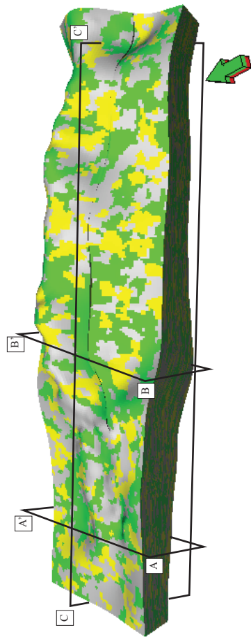
Figure 16. 3-D lithology model with cross-sectional views. Note the greater amount of conglomerate on the northwest side of the study area, and increase in the amount of sandstone toward southeast side. Flooding mudstones can be recognized with their long lateral continuity. Toward northeast (away from source site) the amount of conglomerate decreases while the amount of sandstone increases.
