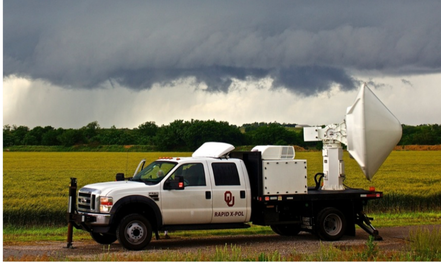
Figure 3.2: The Mobile Rapid-Scan, X-band, Polarimetric (RaXPOL) Doppler radar system. Photo taken by Kyle J. Thiem.
