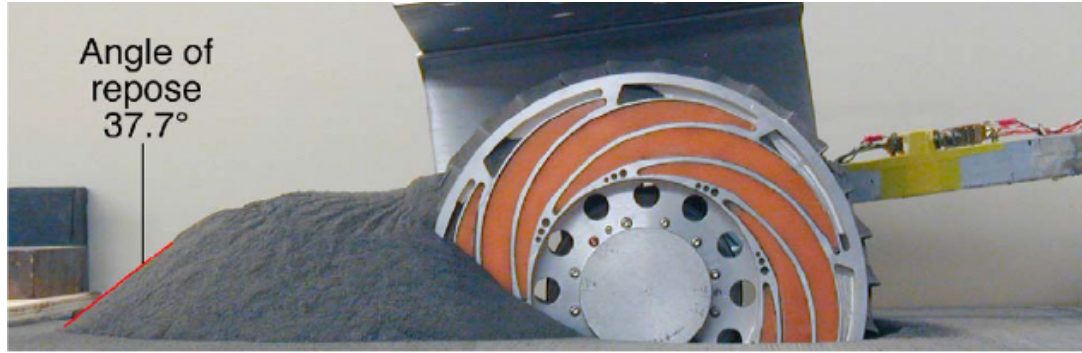
Figure 3.1: Experimental fixture demonstrating repose angle on cohesiveless tailings of JSC-1A lunar regolith [21]
