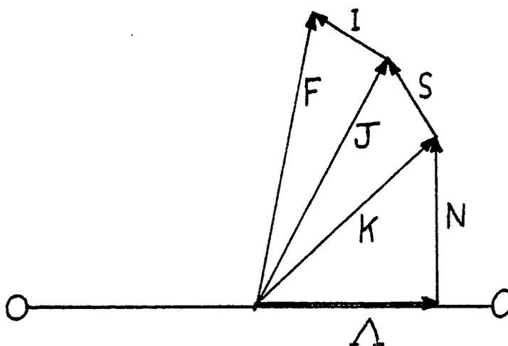
Fig. 4. Schematic diagram of Hund's Case (b) Coupling.
