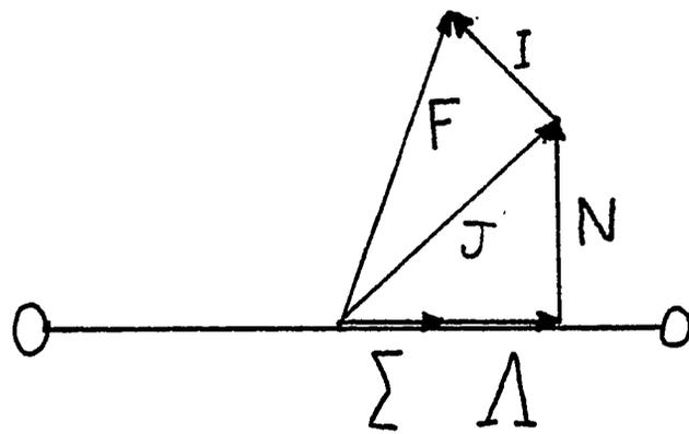
Fig. 5. Schematic diagram of Hund's Case (a) Coupling.
