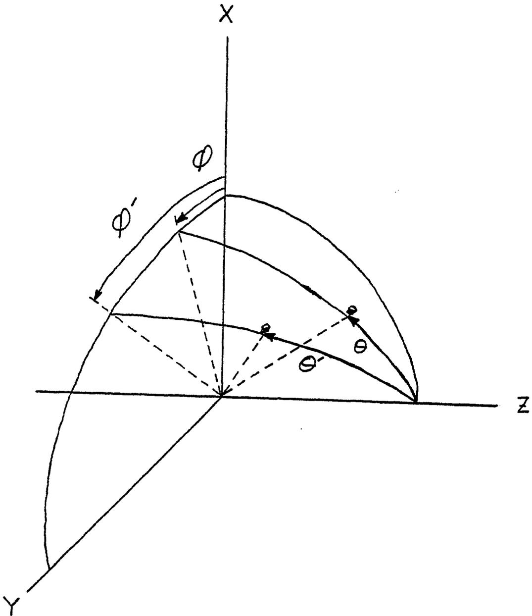
Fig. 1. Coordinate system used in MJ and in the present work. The primed coordinates refer to the photon detector and the unprimed coordinates refer to the electron detector. The electron beam is incident from the  $-Z$  direction.
