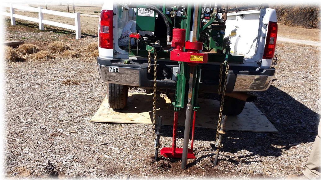
Figure 3.1 – Giddings soil core apparatus mounted on the bed of truck at the Botanic Garden in Stillwater, Oklahoma.
