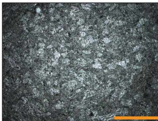
Figure 24. Fine grained grainstone facies (FGGS), in plane-polarized light (PPL) (left), and cross-polarized light (XPL) (right). Grains consist of unidentifiable skeletal fragments <1.25 mm in diameter. The orange scale bar in the lower right of each image is 1mm in length.
