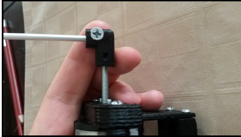
Figure 7.19: Slide the Elbow Onto the Encoder Screw
