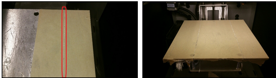
(a) Leave Gap Between Tape Strands (b) Cover the Whole Printer Surface With Tape
