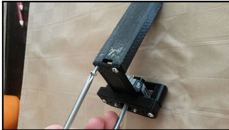
Figure 7.15: Mount Encoder Assembly to Beam
