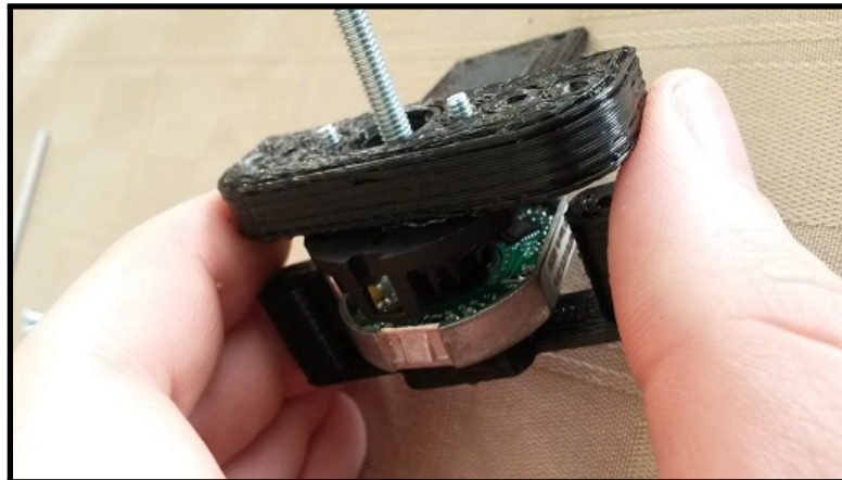
Figure 7.10: Slide the Encoder Mount Assembly Down (Do Not Clip)
