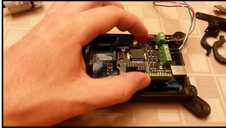
Figure 5.7: Plug Motor Shield Back Into Arduino
