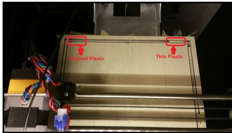
Figure 4.19: Desired vs. Thin Plastic On Plate
