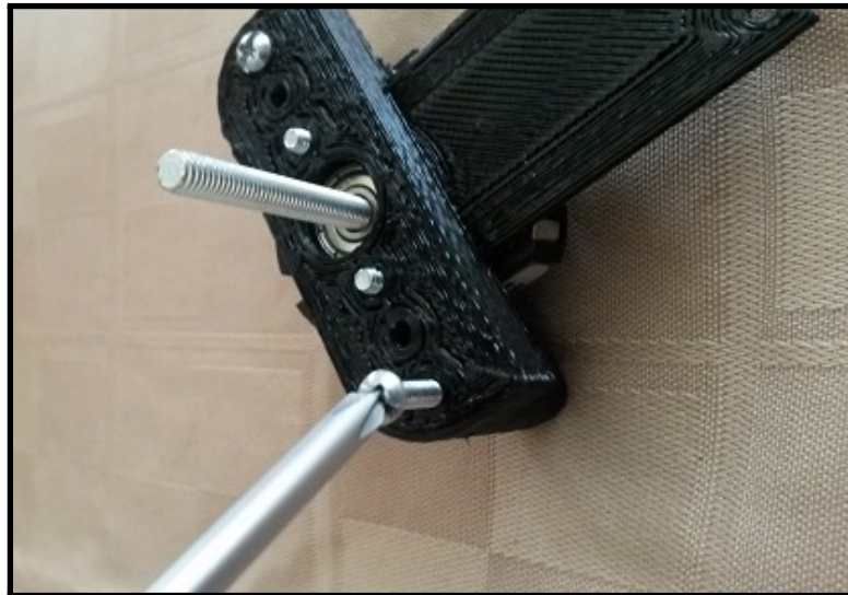
Figure 7.12: Mount the Encoder Mount to the Bearing Holder
