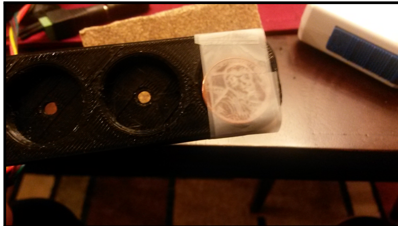
Figure 5.15: Pennies Inserted Into Mass (Suspended with Scotch Tape)
