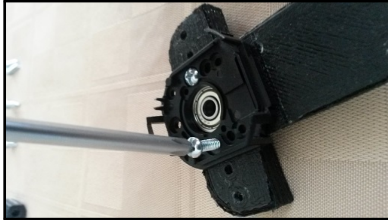
Figure 7.4: Mount Black Backing of the CUI Encoder Kit to the Encoder Mount
