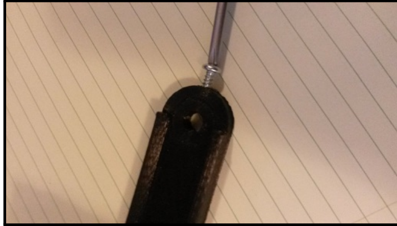
Figure 7.25: Screw Self-Drilling Screw Into the Back of the Beam
