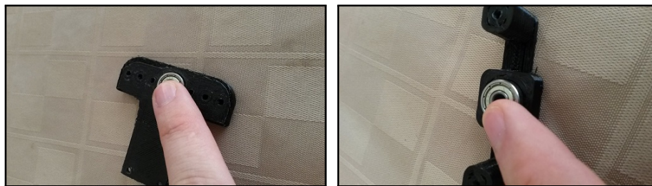
(a) Press Bearing Into 3D Printed Encoder Mount (b) Press Bearing Into 3D Printed Bearing Holder
