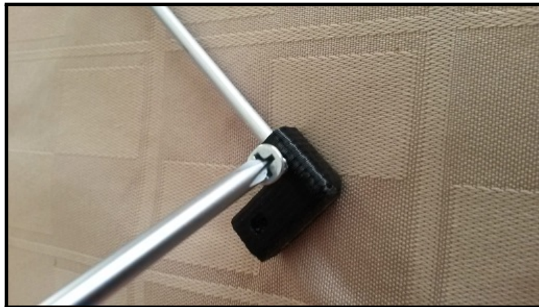
Figure 7.18: Hardware Used to Attach the Pendulum to the Encoder Screw
