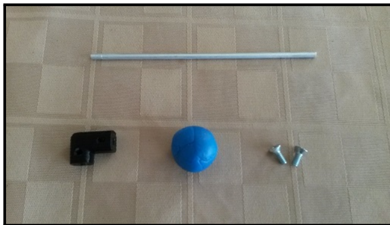
Figure 7.16: Hardware Used to Attach the Pendulum to the Encoder Screw
