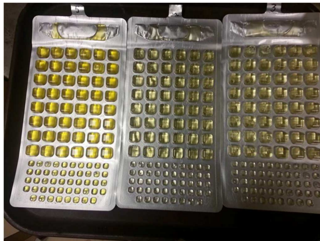
Figure 5. Example of chromogenic result for the presence of Coliform bacteria in a sample of the wastewater. Note the color difference in the sample on the left, which showed a chromogenic indication (dark yellow in color) compared to the right, where the result was negative for each of the wells.
