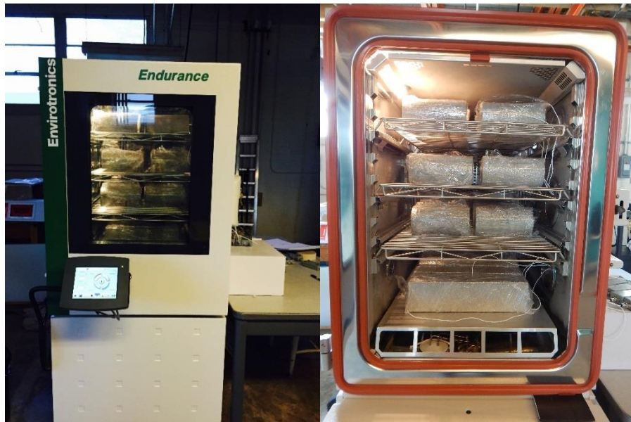
Figure 6: Samples placed in environmental chamber for exposure regimen
