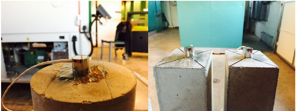
Figure 8: Sensor glued to the specimen
