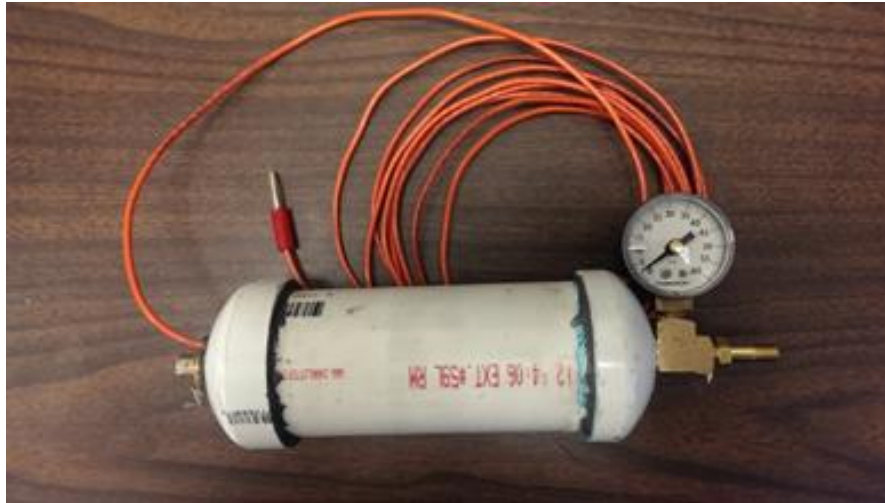
Figure 3.8 – The pressurized solid core PVC detector (SPVC-P).
