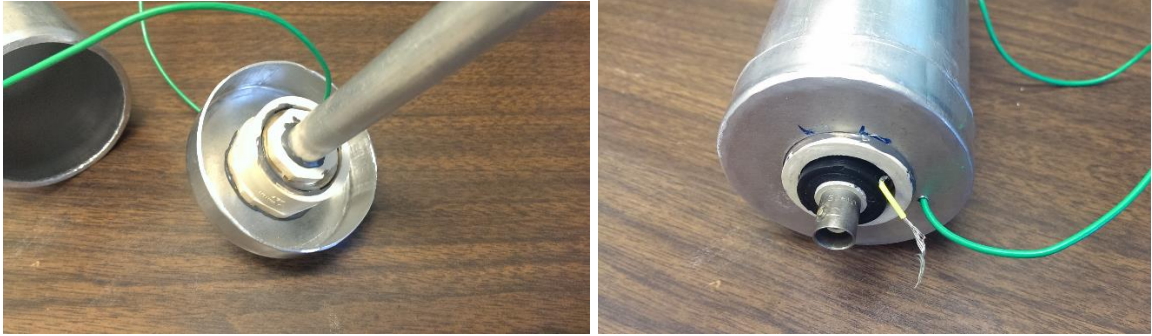
Figure 3.12 – (Left) The insulated electrode assembly used in the aluminum ion chamber. (Right) Exterior of the electrode assembly.
