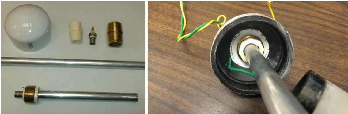
Figure 3.3 – (Left) Hardware used to construct the basic electrode assembly of the SPVC-B ion chamber. (Right) The finished electrode assembly seated in the graphite coated PVC endcap.
