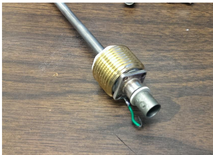
Figure 3.7 – The HV connector and the BNC connector were used to construct a solid base for the SPVC-SE electrode.
