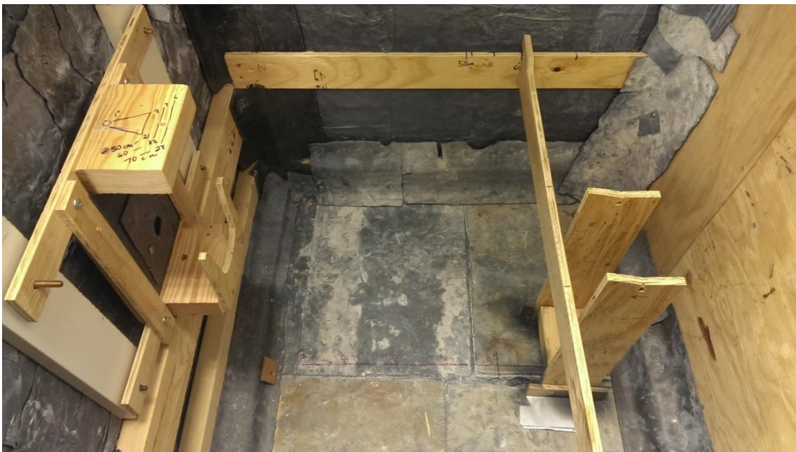
Figure 3.1- Interior testing space of the El Vacatron x-ray system. To the left is the x-ray beam collimator and to the right is the ion chamber positioning stand and cross bar.
