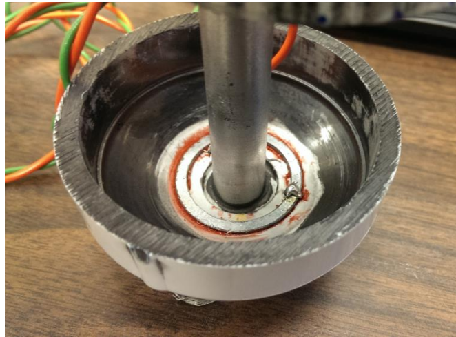
Figure 3.9 – Shows the superficial guard ring of the CPVC-R detector, used in place of the brass cylinder guard ring.
