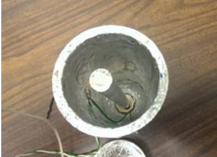
Figure 3.10 – The cellular core PVC detector lined with aluminum foil (CPVC-AI).
