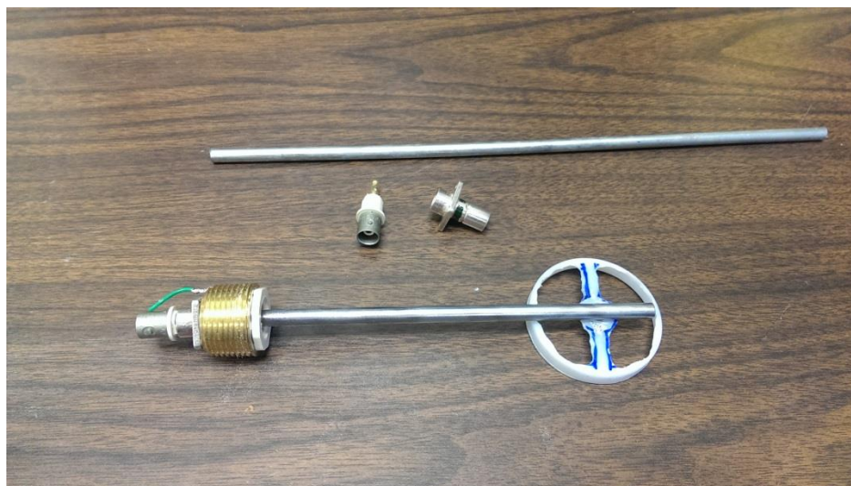
Figure 3.6 – Some of the electrode assembly components and the finished product of the SPVC-SE ion chamber.
