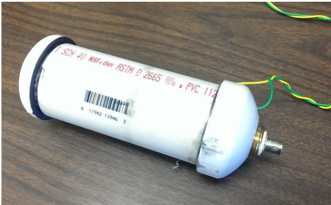
Figure 3.4 - The solid core PVC basic ion chamber (SPVC-B). The interior wall was coated with graphite to make it conductive.
