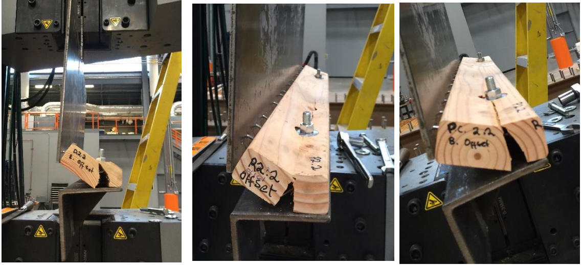
Figure 4-6 Fracture of SAMPLE#3 Specimens along bottom face.
