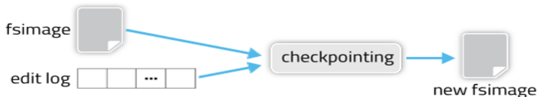
Fig. 2.1 Checkpoint creates a new fsimage from an old fsimage and edit log
