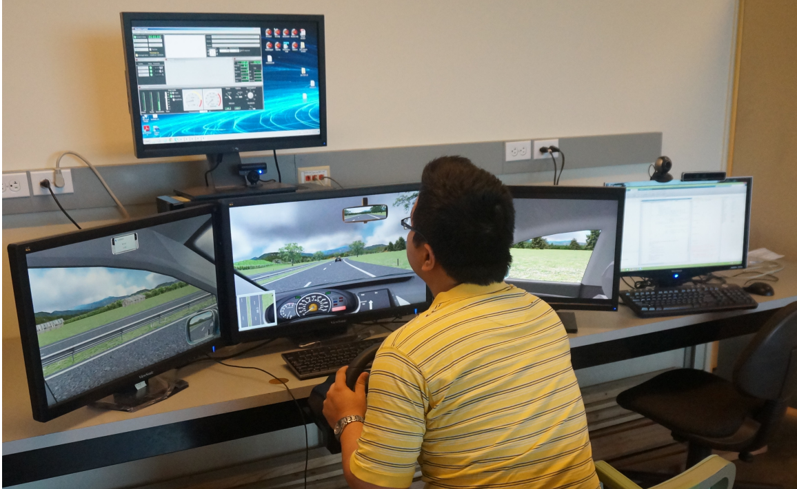
Figure 4.4: Carnetsoft's simulator utilizes 3 monitors for realistic panoramic view from the cabin and 1 monitor for setup and simulation parameters while the steering wheel set Logitech G27 controls the human-driven vehicle. The autonomous vehicle is controlled by a separate computer using Ethernet connection and can be seen from the side only.
