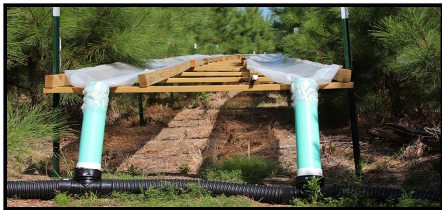
FIGURE 5. Images of the \frac{1}{3} throughfall excluders showing drainage design which directs precipitation away from the measurement plots in McCurtain County, Oklahoma. [Source: Photos courtesy of Duncan Wilson, 2012]
