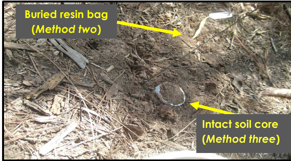
FIGURE 8. Photo showing placement of Method two and Method three within a measurement plot of a loblolly pine plantation, McCurtain County, Oklahoma.
