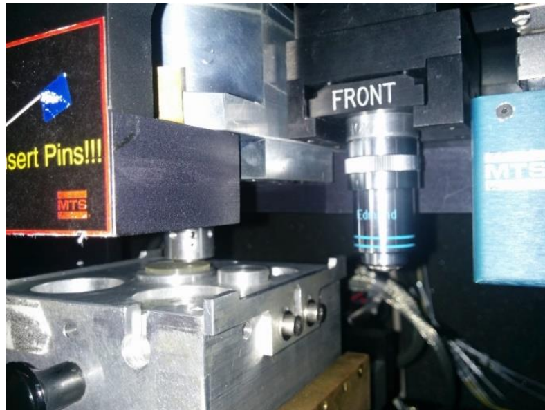
FIGURE 2.5 Sample and testing apparatus of Nano indenter system
