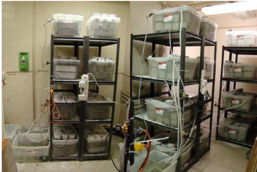
Figure 3.2: Specimens cured in sodium sulfate solutions in controlled conditions.
