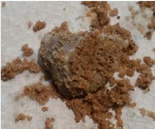
Fig. 9-22 shows wet sand attached to coarse aggregate.
