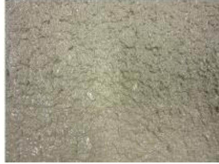
Fig. 9-4 shows impacts of excessive coarse sand amounts.
