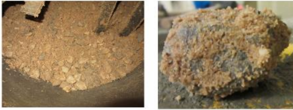
Fig. 9-9 shows wet sand being attached to coarse aggregate.
