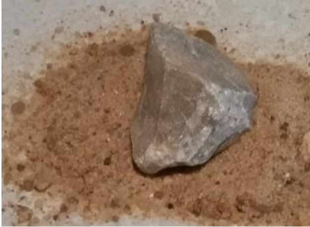
Fig. 9-21 shows dry sand not attaching to coarse aggregate.
