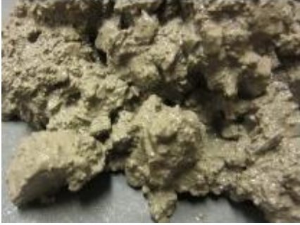
Fig. 9-4 shows impacts of excessive coarse sand amounts.
