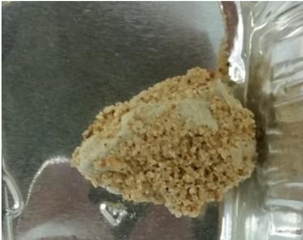
Fig. 9-23 shows dried fine aggregate still attached to coarse aggregate.
