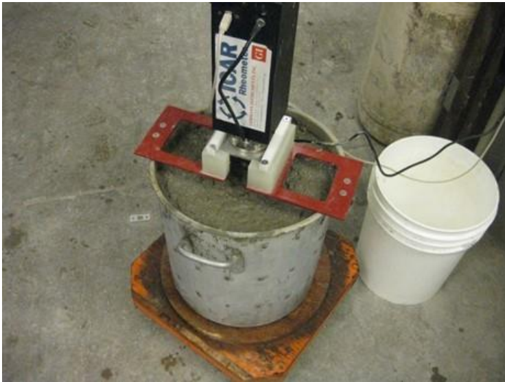
Fig. 6-8 shows the rheometer finding the flowability properties of a mixture.
