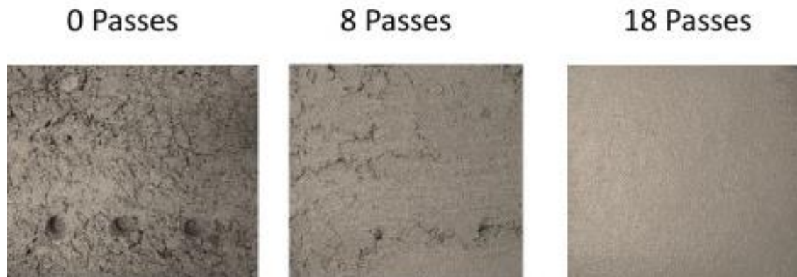
Fig. 8-14 shows poor finishability of mixture 52 with high amounts of #8.
