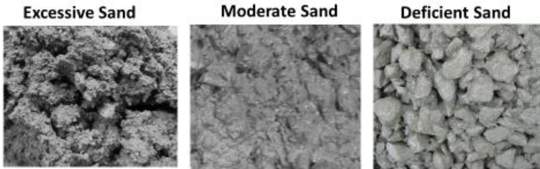
Fig. 8-2 shows from visual observation the excessive and deficient amounts of sand.
