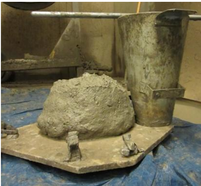
Fig. 6-1 shows the Slump Test being conducted on a flowable concrete mixture.
