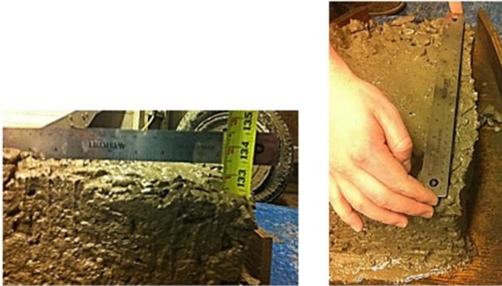
Fig. 5-2 shows edge slumping issues due to poor cohesion.
