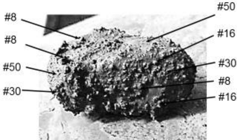
Fig. 9-10 shows a piece of coarse aggregate pulled out of good workability concrete.
