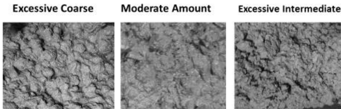
Fig. 9-2 displays the visual observations of excessive amounts of coarse and intermediate sieve sizes.
