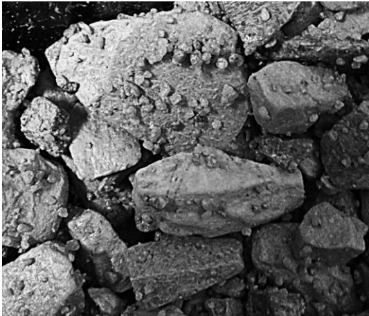
Fig. 9-11 shows wet sand being attached to coarse aggregate.
