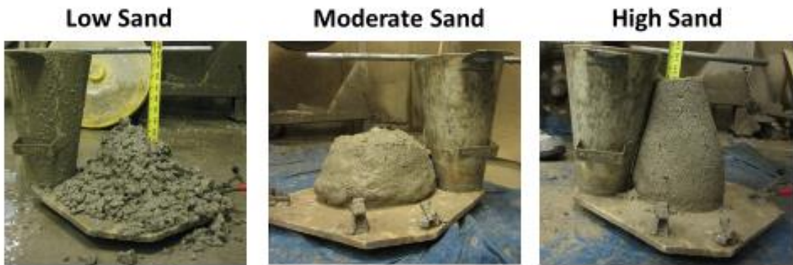
Fig. 8-3 shows the Slump Test measuring the excessive and deficient amounts of sand.
