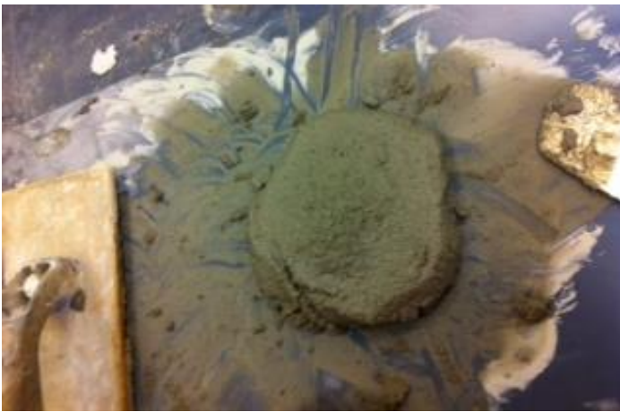
Fig. 9-12 shows a mortar mixture being evaluated for smoothness.
