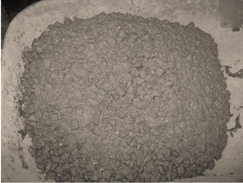
Fig. 8-13 shows poor cohesion of mixture 39 without #8 and #16.
