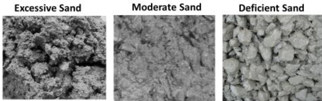
Fig. 9-3 shows from visual observation the excessive and deficient amounts of sand.
