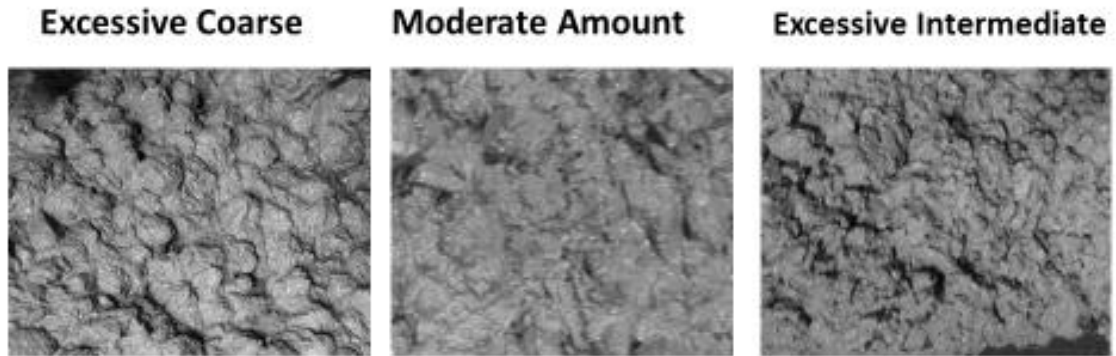
Fig. 7-2. Displays the visual observations of excessive amounts of coarse and intermediate sieve sizes.
