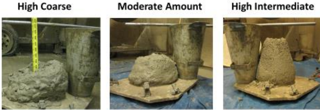
Fig. 7-3. Shows the Slump Test measuring the excessive amounts of coarse and intermediate sieve sizes.
