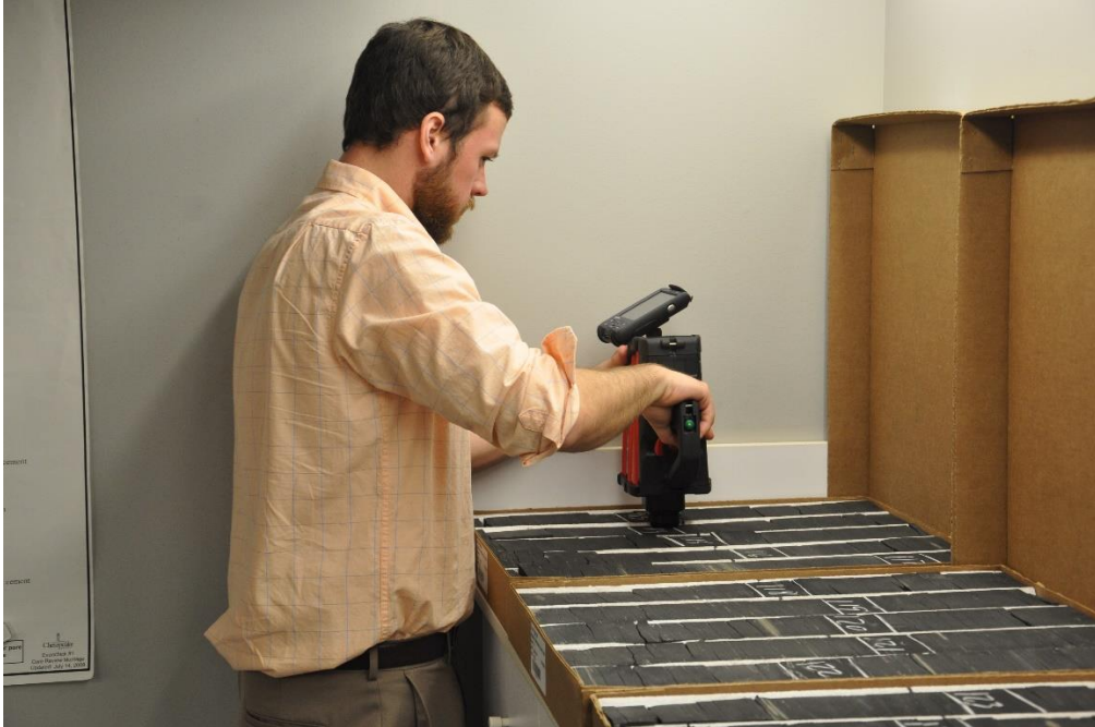
Figure 5: Measuring the core using the 4100 FTIR ExoScan.
