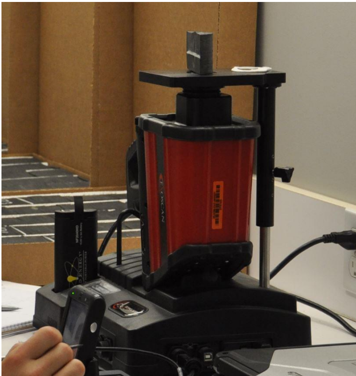
Figure 6: ExoScan stand with a core piece being measured perpendicular to bedding.
