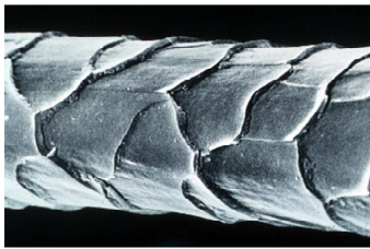
Figure 17- Cuticle Layer of Wool 33
