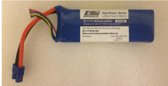
Figure 132: E-flite 3S, 1800mAh battery
