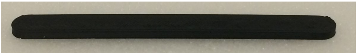
Figure 27: Horizontally printed bending test specimen
