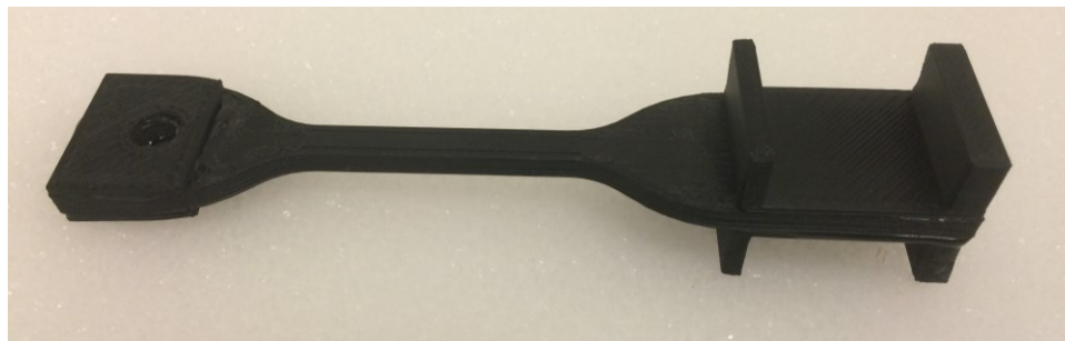
Figure 33: Tensile test sample with grip add-ons
