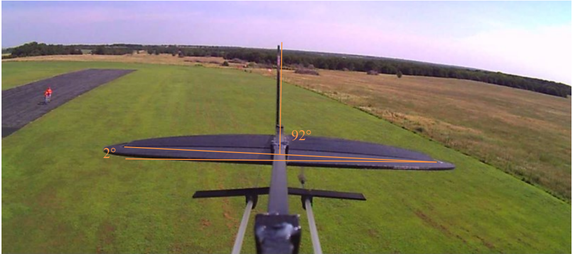
Figure 112: Phoebe tail reference state with angle measurements
