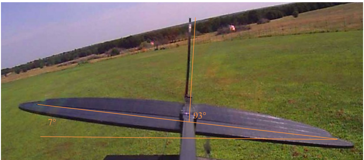
Figure 113: Phoebe tail deflected state with angle measurements
