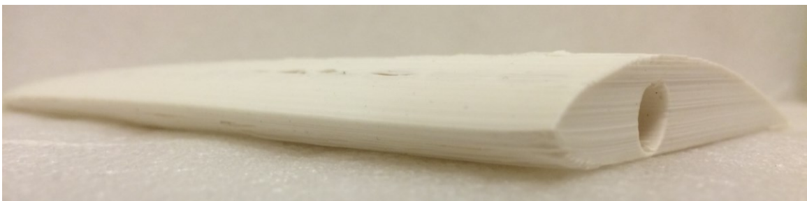
Figure 39: Horizontally printed wing section (leading edge and airfoil profile)
