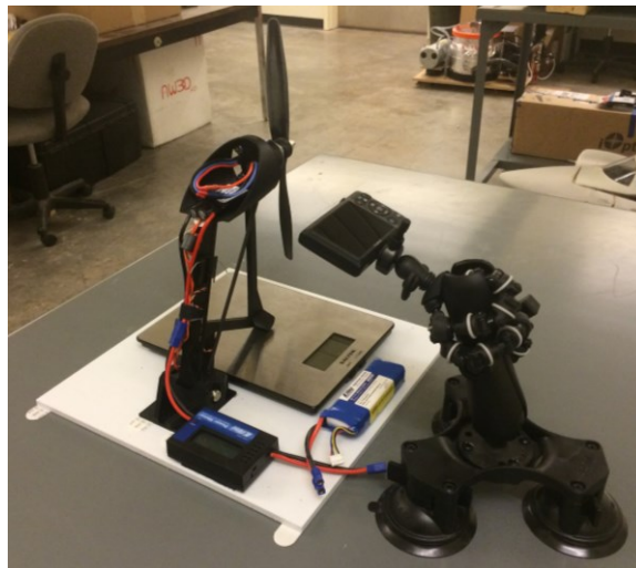
Figure 133: Static thrust stand with test instrumentation and propulsion system
