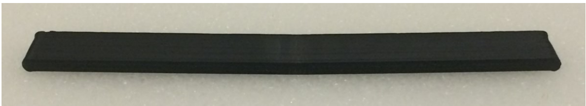
Figure 28: Vertically printed bending test specimen
