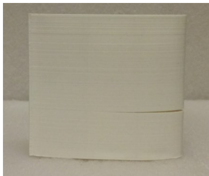
Figure 25: Wing test piece with leading edge split
