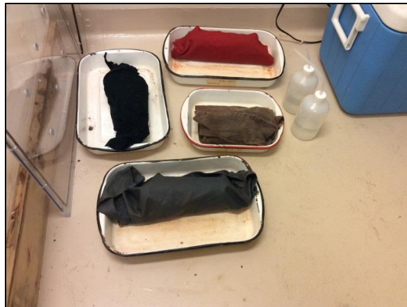
Figure 3.3 Wetting Process of Soil Samples (1)
