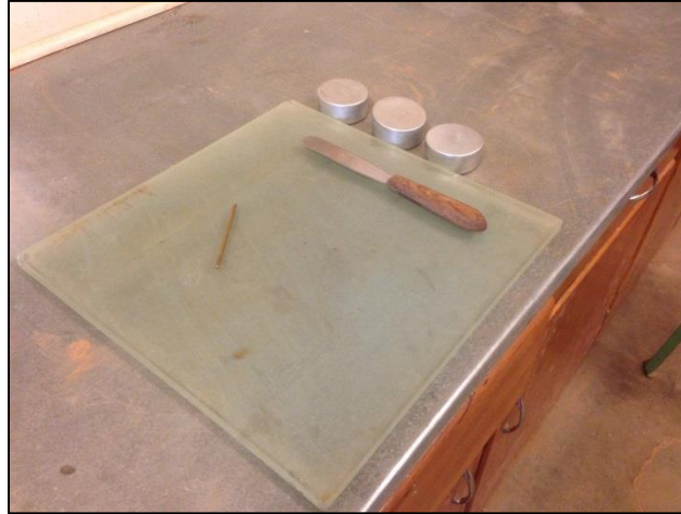
Figure B.2 Plastic Limit Test Setup
