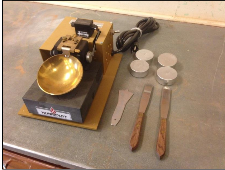
Figure B.1 Liquid Limit Test Setup
