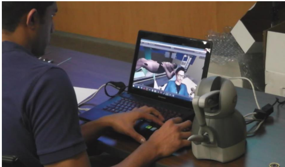
Figure 15. Resident interacting with VEOS using a Phantom haptic interface (Non-immersive virtual surgical environment)
