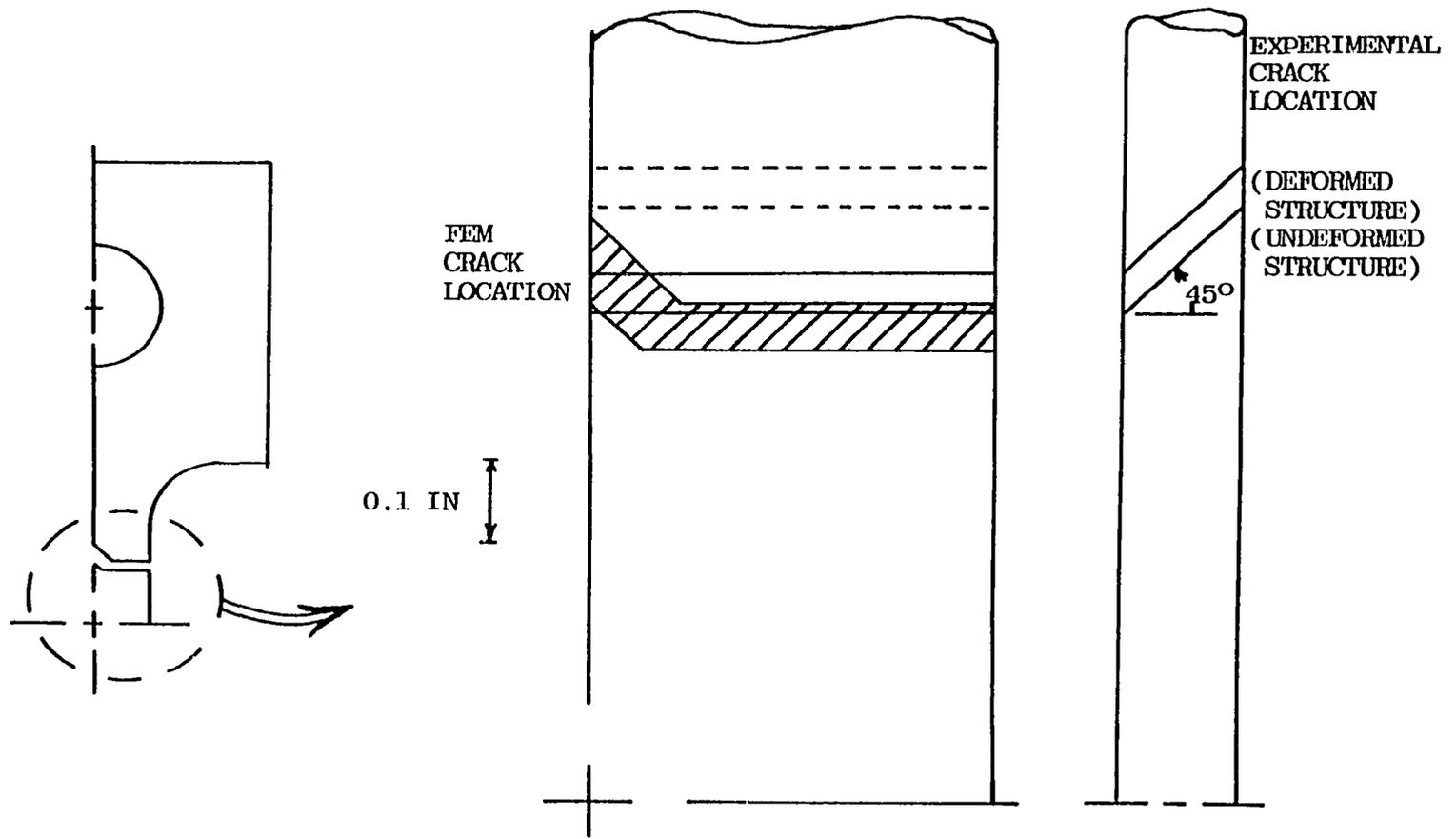
Figure 5.7. Crack Locations, FEM Predictions and Experimental Results for Tensile Test Specimen.
