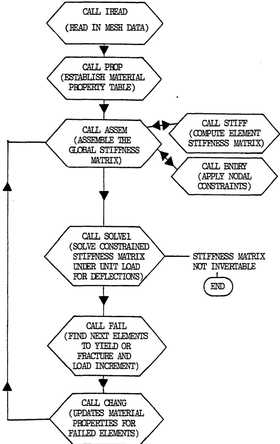
Figure 3.4. Flow Chart for the Program FRACTURE.
