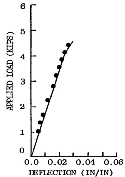
Figure 6.4. Load Deflection Curves for Cracked Specimen Analysis.
