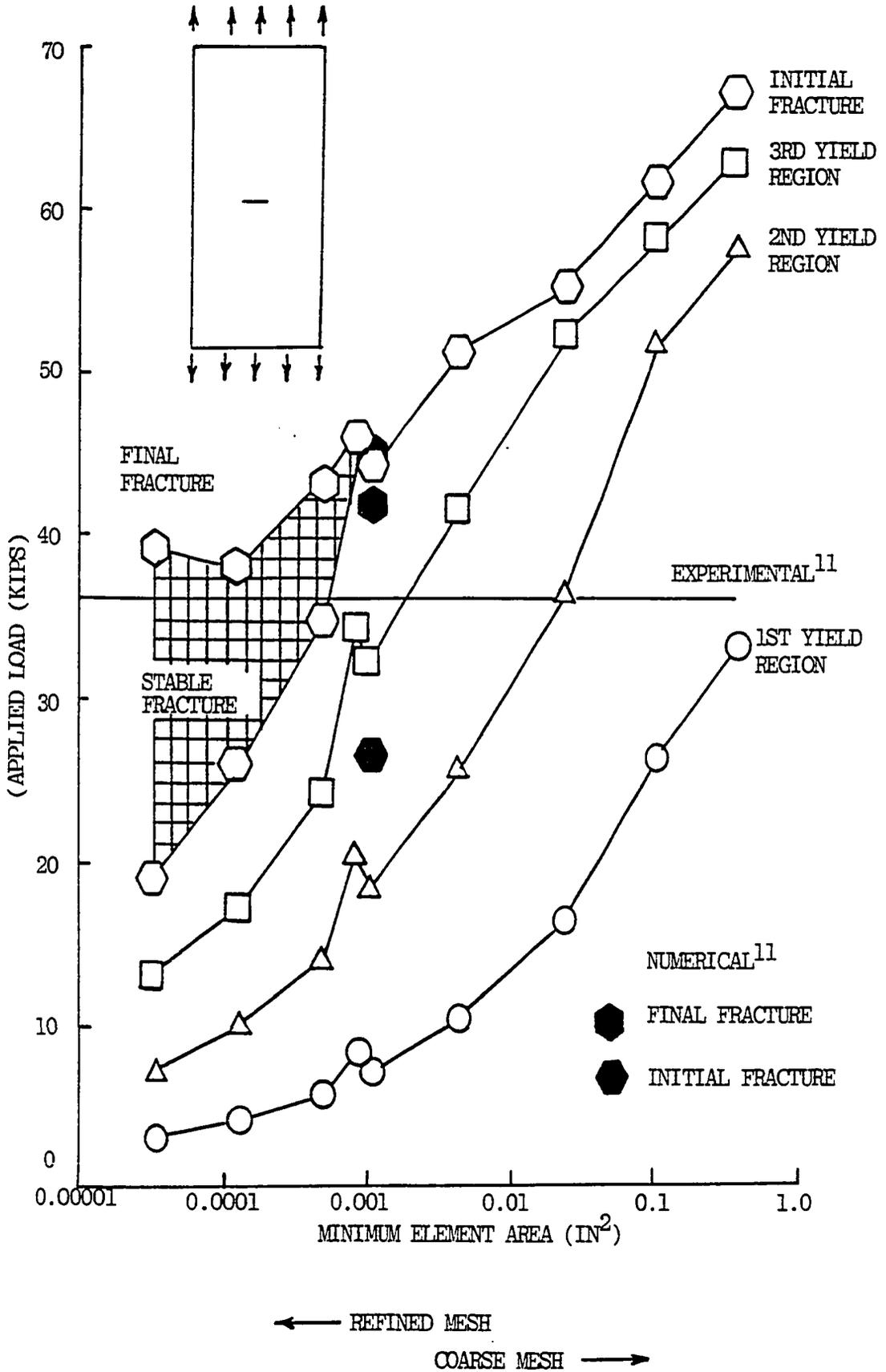
Figure 4.2. Numerical Convergence, Cracked Panel Study.
