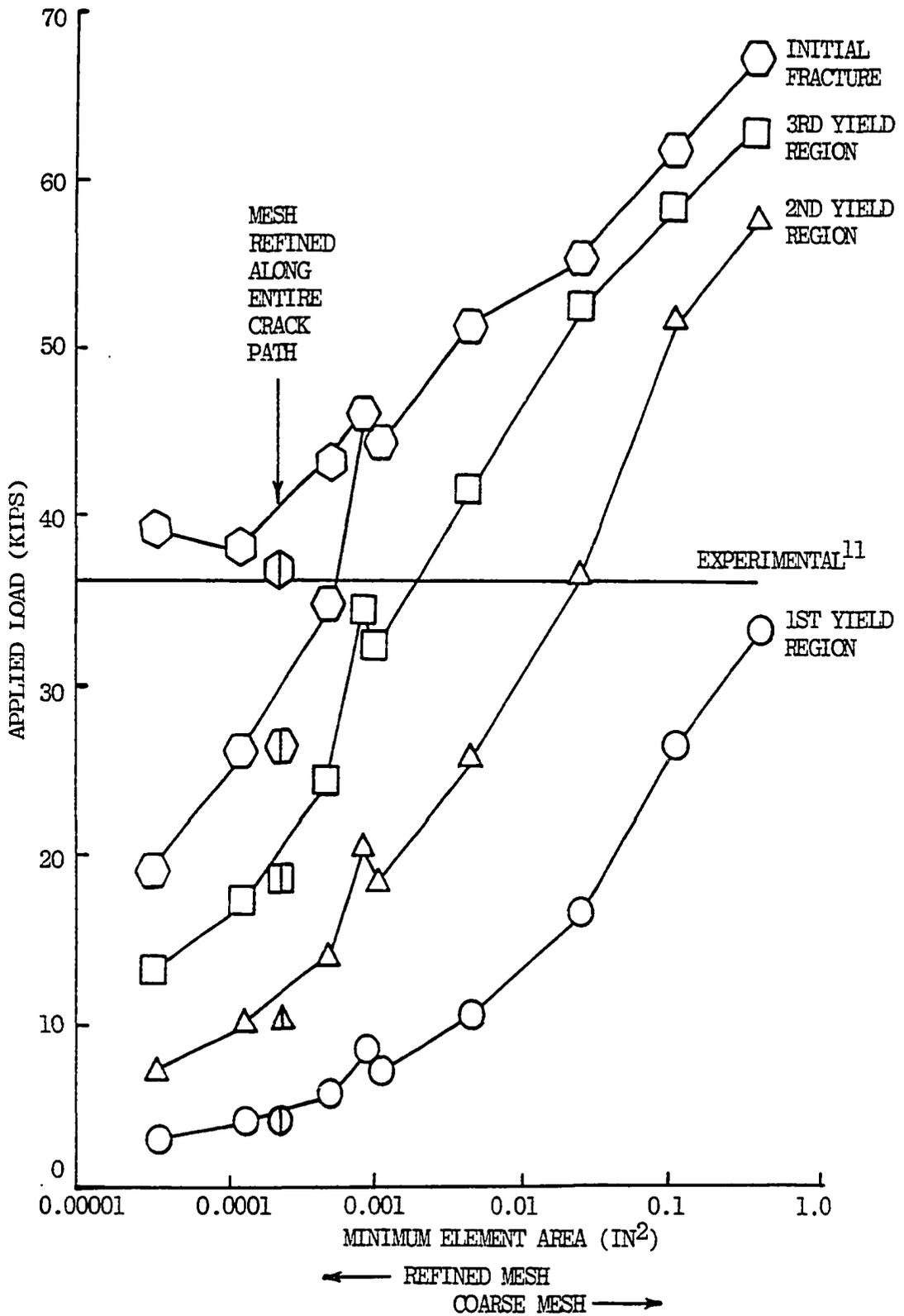
Figure 4.3. Effect of Mesh Refinement Along the Crack Path
