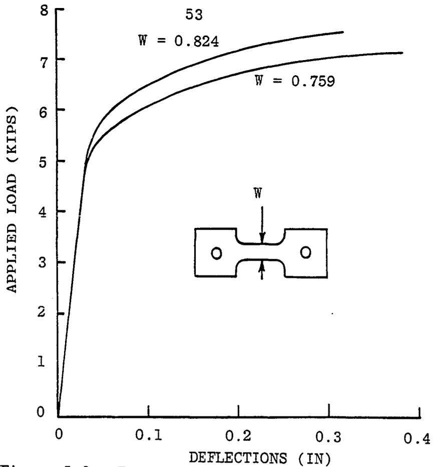
Figure 5.2. Tensile Test Load Deflection Curves.
