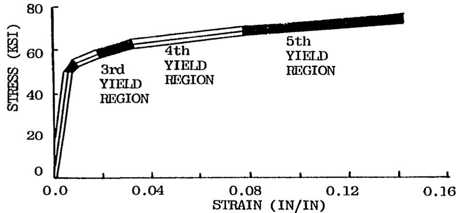
Figure 5.6 (cont). Yield Regions, Tensile Test Specimen.
