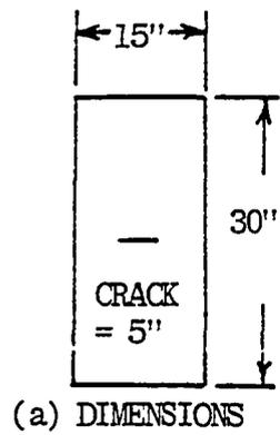
Figure 4.1. Cracked Panel Dimensions and FEM Models.
