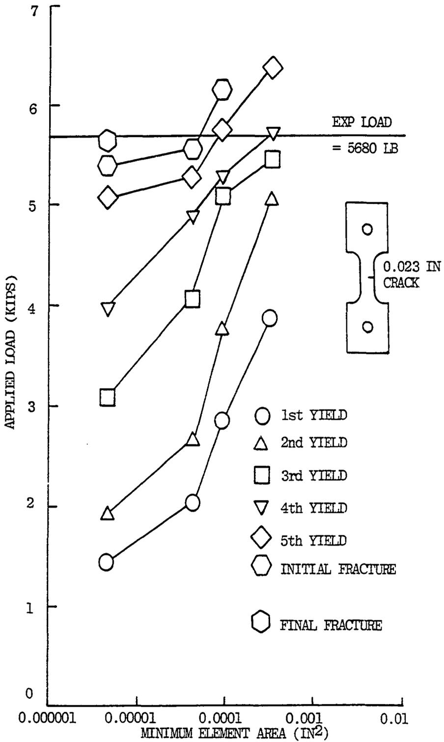
Figure 6.2. Numerical Convergence, Cracked Specimen Analysis.
