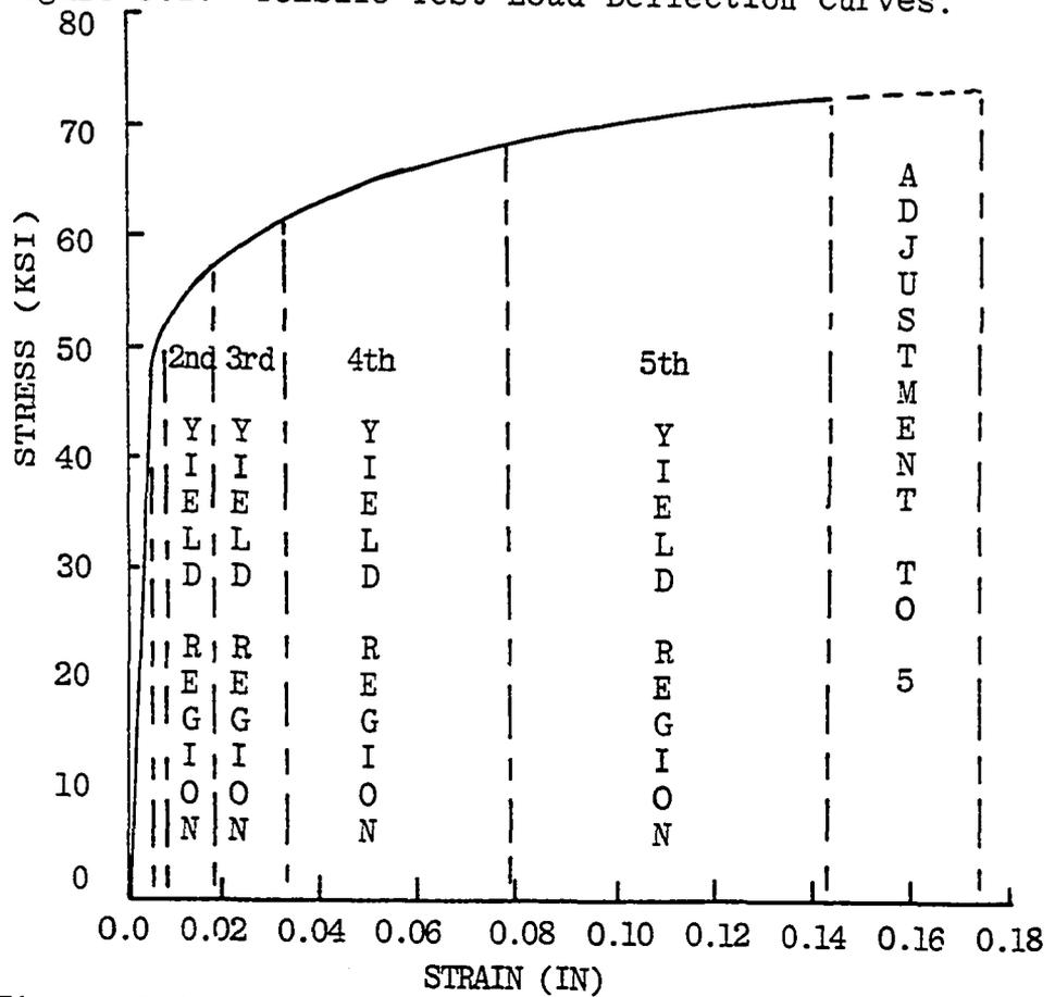
Figure 5.3. Linearized Stress-Strain Curve.
