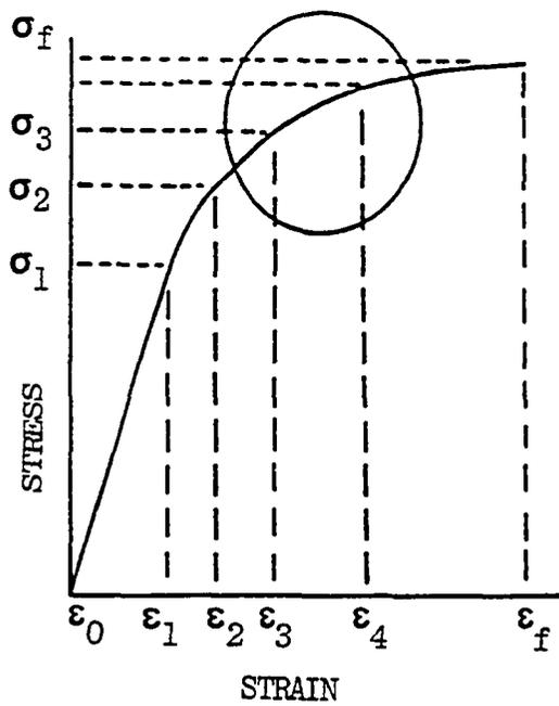
Figure 3.1. Linear Approximation of a Stress-Strain Curve.
