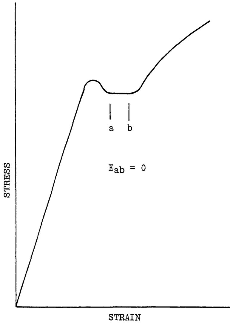
Figure 3.3. Stress-Strain Curve with Zero Modulus Section.
