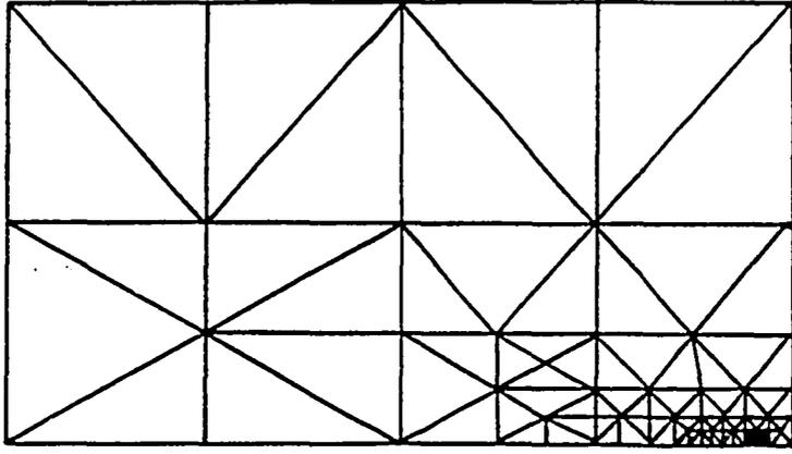
(b) Detail of Mesh for 0.008 In. Crack
