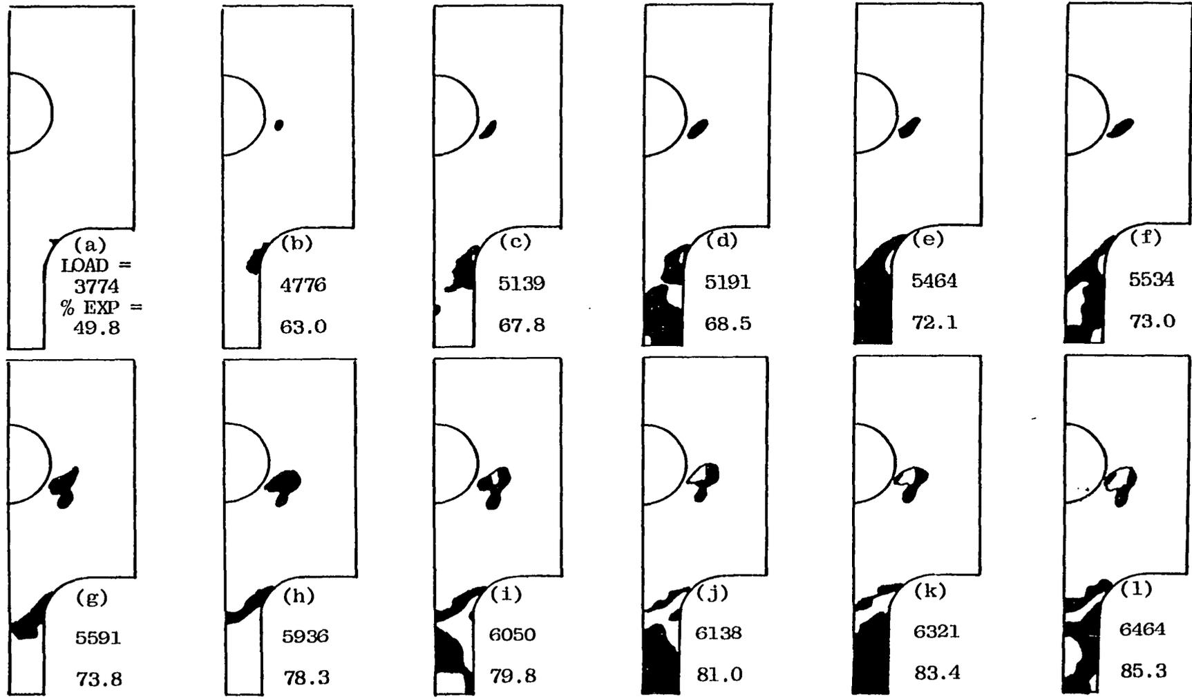
Figure 5.6. Yield Regions for Tensile Test Specimens.
