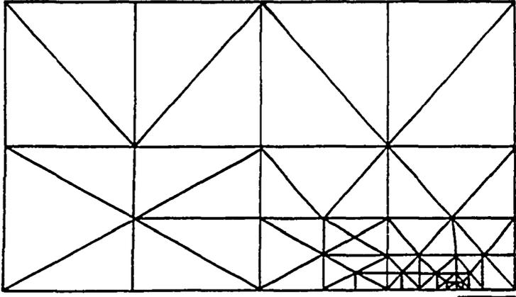
(c) Detail of Mesh for 0.023 In. Crack
