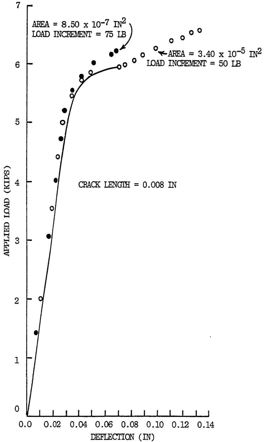
Figure 6.3. Effects of Load Increment and Element Size for the Cracked Specimen Analysis.
