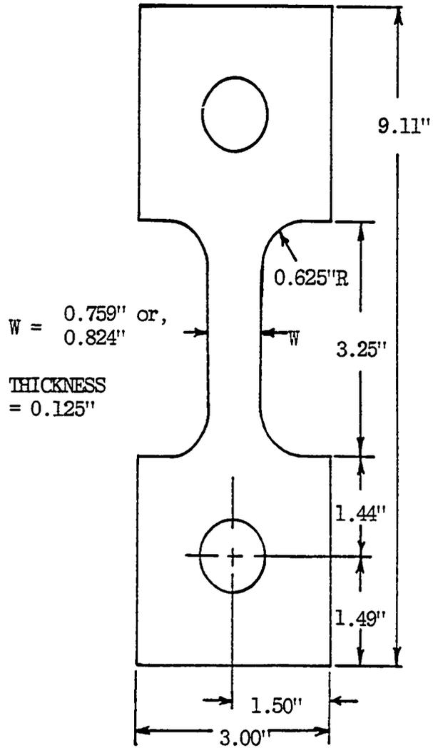
Figure 5.1. Tensile Test Specimen Dimensions.
