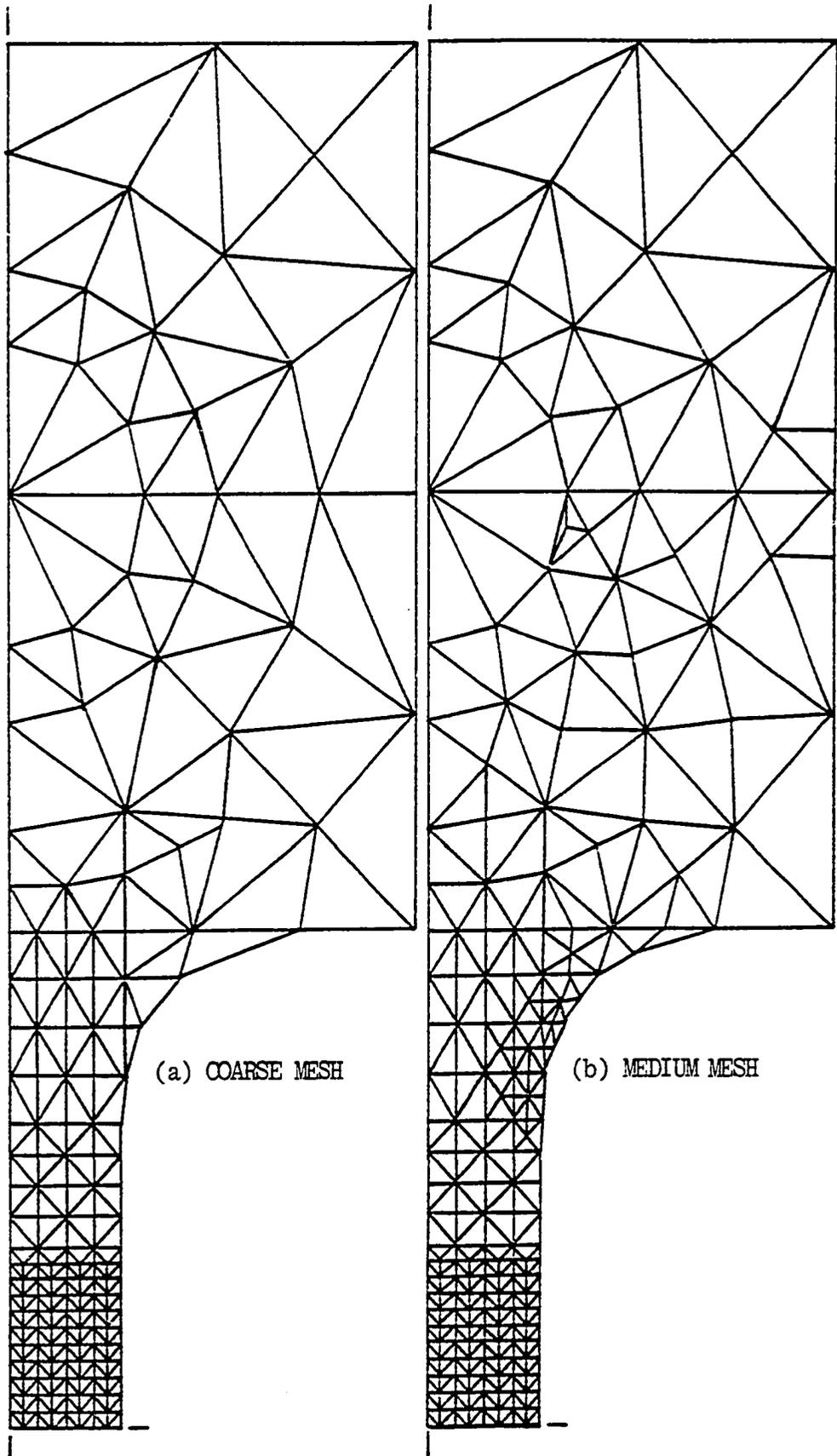
Figure 5.4. Tensile Test FEM Models.
