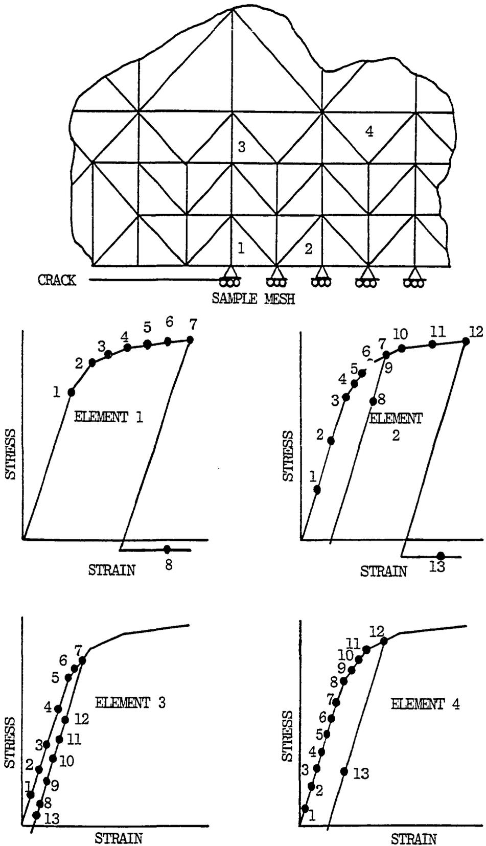
Figure 3.2. Typical Element Response, "Zero Modulus-Unload Reload" Method
