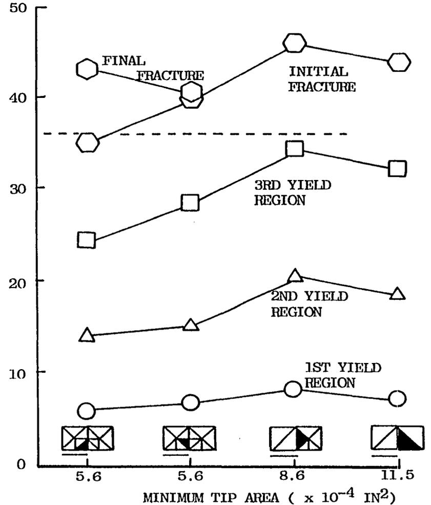
Figure 4.5. Effects of Element Orientation.
