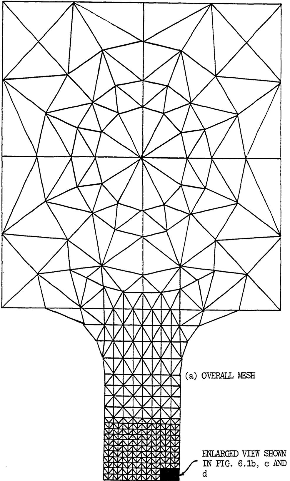
Figure 6.1. FEM Models of Cracked Specimens.
