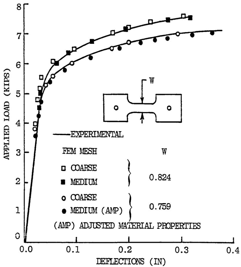
Figure 5.5. FEM Load Deflection Predictions for Tensile Test Specimens.
