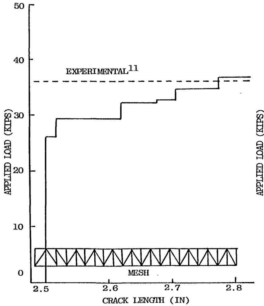
Figure 4.4. FEM Crack Growth Prediction.
