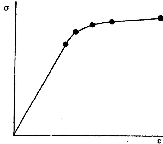
(b) Linearized stress-strain curve
