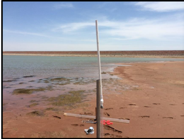
Figure 13: Extraction of push core from Canton Lake, OK.
