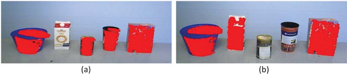
Figure 3.10: Object recognition results 1. The objects from left to right are bowl, milk box, coffee can, cup, cereal box. (a) bowl, coffee can, cup and cereal box have been recognized. (b) bowl, milk box, cereal box have been recognized.
