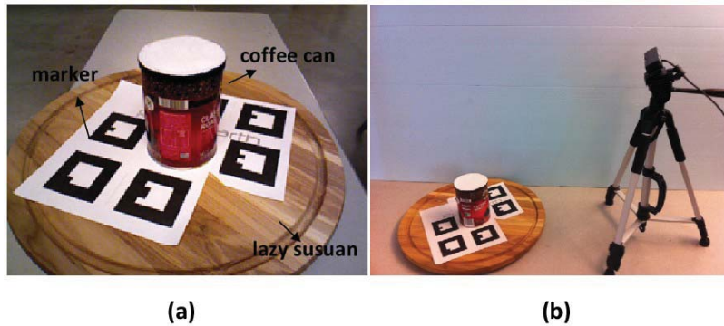
Figure 3.3: Setup for 3D object model modeling. (a) the camera view. (b) the object recording setup.
