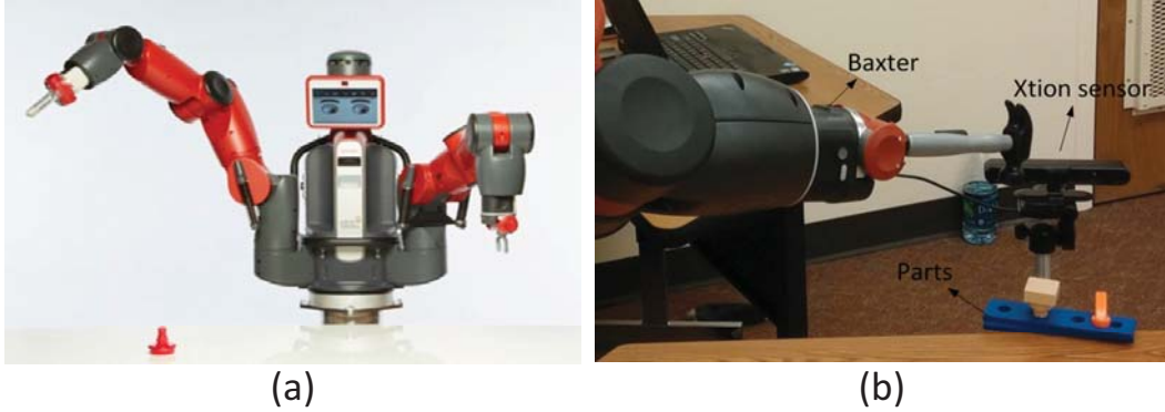
Figure 6.2: The robot implementation setup. (a) The Baxter robot [2]. (b) The workspace of the Baxter robot.
