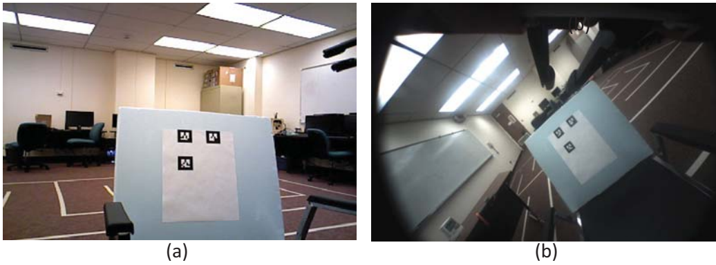
Figure 6.3: Camera views. (a) The Xtion color image view. (b) The left gripper camera view.
