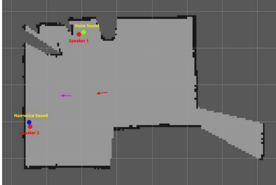
Figure 4.11: Sound position estimation by triangulation
