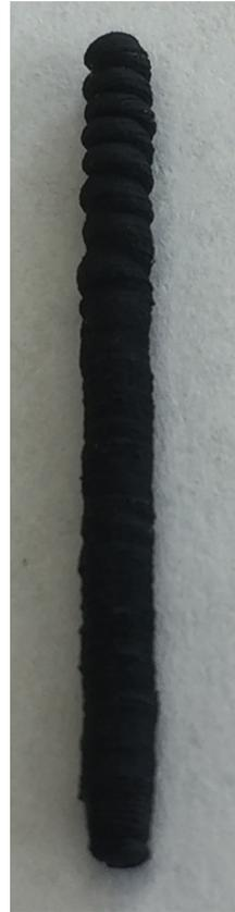
(b) Example of a vertical print with cross-sectional area of  $2.4mm \times 2.4mm$ .
