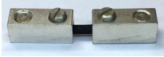
Figure 3.3: *Screw terminals used to in conjunction with an ohmmeter to obtain resistance values of samples. Each side is connected to one of the leads coming from the ohmmeter.*
