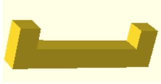
Figure 3.1: Profile of a  $4\text{ mm} \times 4\text{ mm} \times 30\text{ mm}$  sample. The additional material at the ends of the material is used to mount the piece in the testing apparatus.
