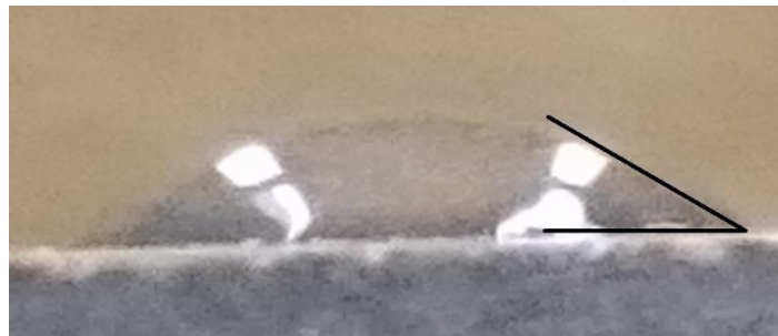
Figure 4. 8 contact angle measurement with image J software
