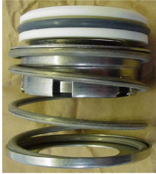
Figure 2-7 A mechanical seal located at the top of protection chamber to prevent fluid from traveling down the drive shaft (Stanghelle, 2009)
