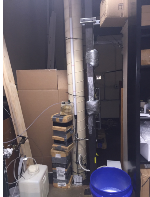
Figure 3-2 Sketch and picture of the water and oil final vertical flow loop setup
