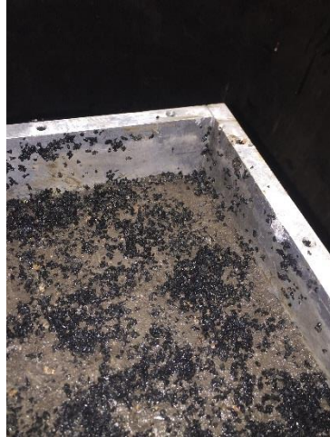
Figure 40. Soil Swell After Testing
