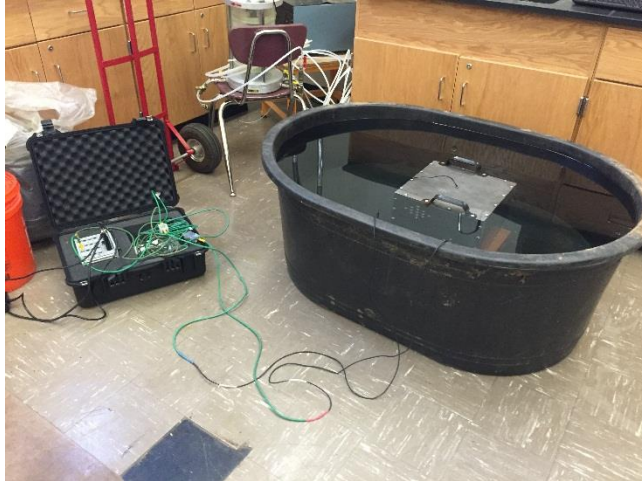
Figure 16. Testing Setup with Submerged Box and Somat DAQ System
