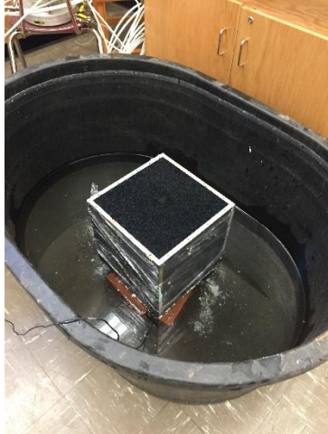
Figure 17. Box with Compacted Soil and Crumb Rubber After Testing
