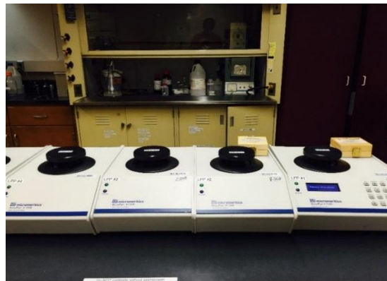
Figure 13: Micrometrics model II LPP Helium pycnometer for measuring proppant grain density.
