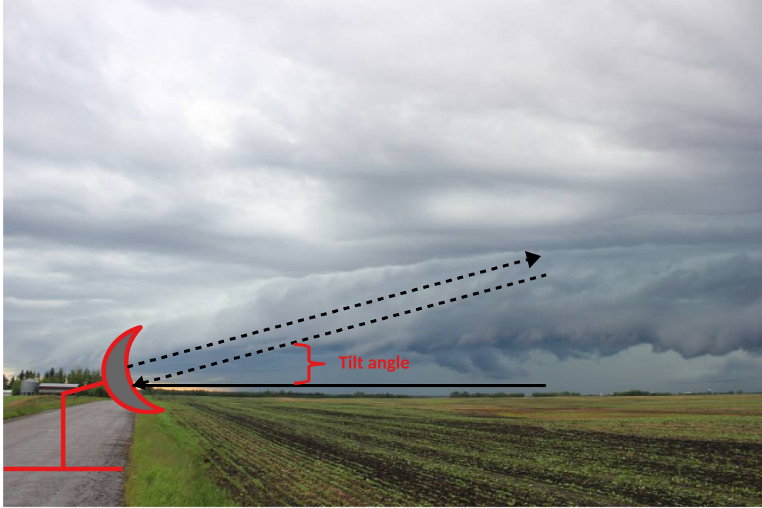
Figure 3.1: Basic radar operation. The radar emits horizontally polarized waves (along the dashed line pointing outward) and receives scattered waves from atmospheric particles.
