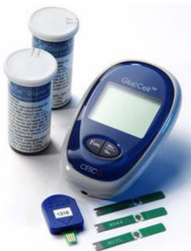
Figure 14. GlucCell™ Glucose Monitoring System 92 Glucose measurements were obtained with the GlucCell™ (CESCO BioProducts). The device is depicted along with two vials of test strips, three individual test strips, and a device tester.
