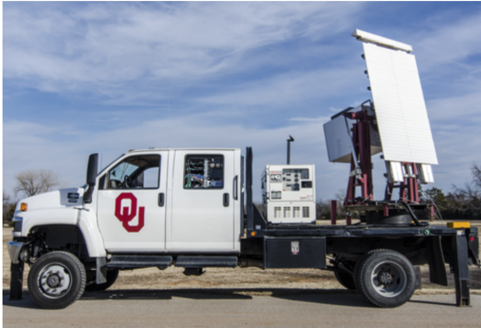
Figure 3.1: The Atmospheric Imaging Radar (Kurdzo et al. 2016). Energy is transmitted in a fan beam, and received by each individual receiving element.
