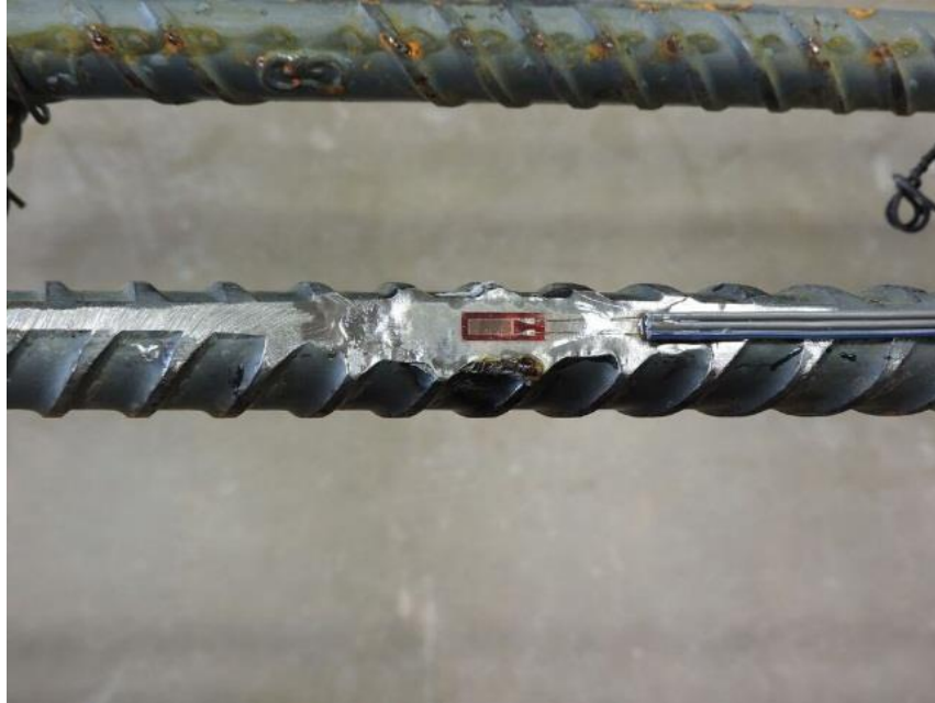
Figure 4.5: Strain Gauge Adhered to Longitudinal Bar
