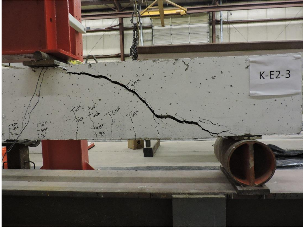
Figure C.19: K-E2-3 Failure Crack Front View
