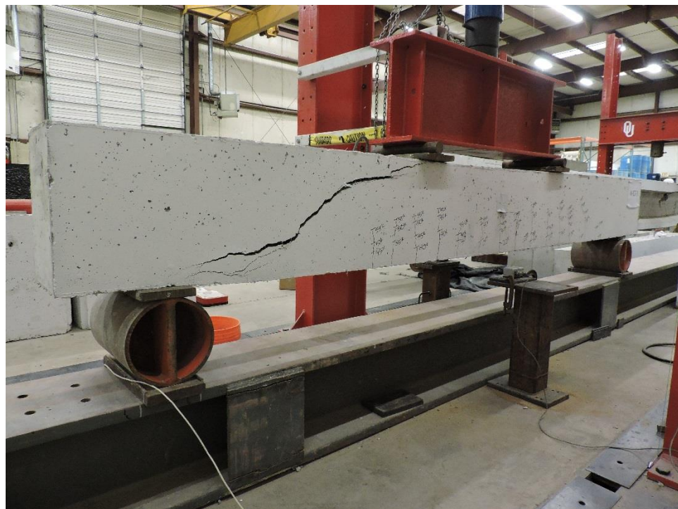
Figure C.6: K-E2-1 Failure Crack Left View
