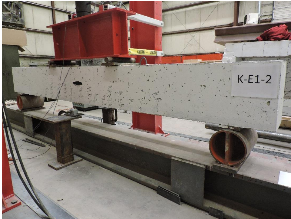
Figure B.7: K-E1-2 Crack Propagation 50 kips
