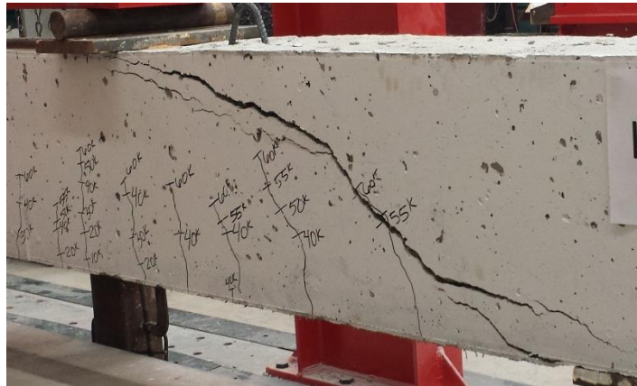
(b) K-E1-2 Failure Crack
