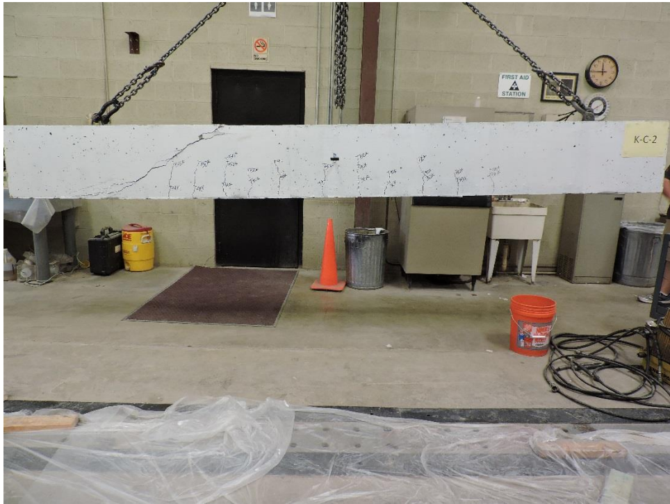
Figure A.13: K-C-2 Failed Beam
