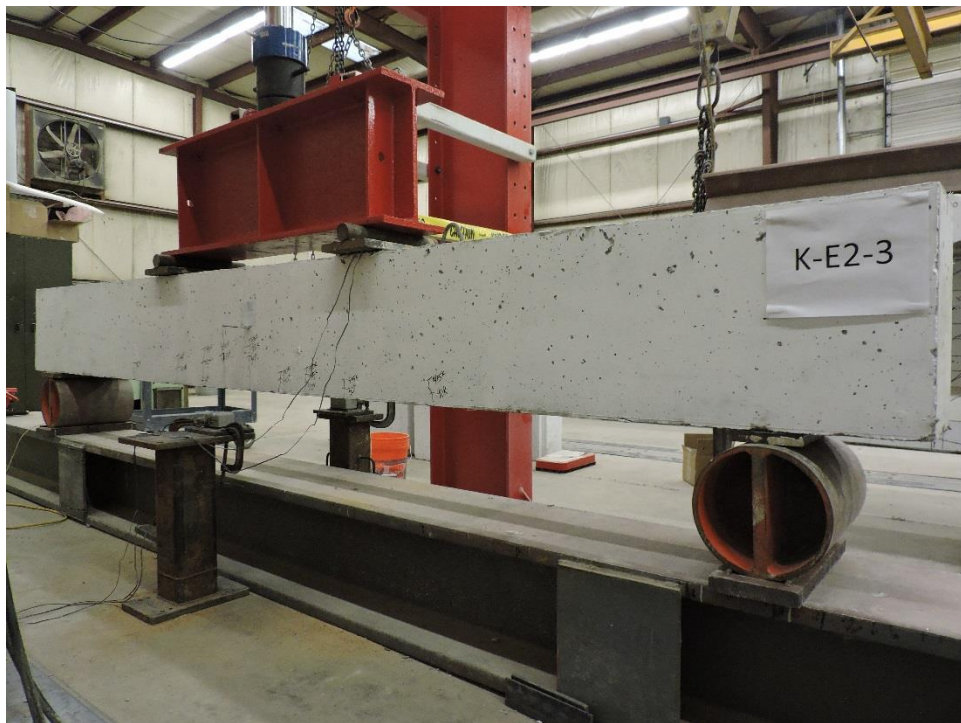
Figure C.16: K-E2-3 Crack Propagation 50 kips
