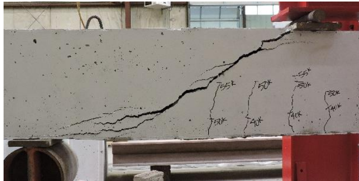
(b) K-C-2 Failure Crack
