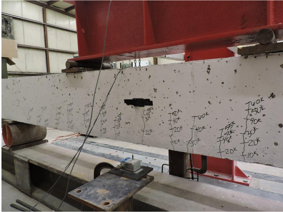
Figure B.9: K-E1-2 Crack Propagation 60 kips
