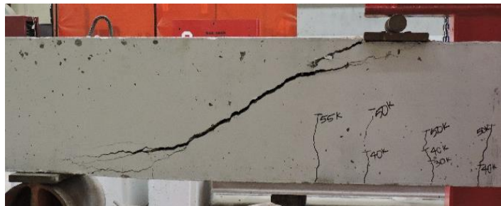
(c) K-C-3 Failure Crack
