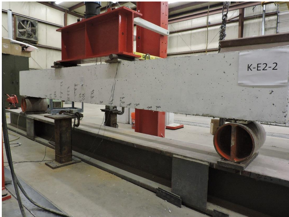
Figure C.10: K-E2-2 Crack Propagation 45 kips
