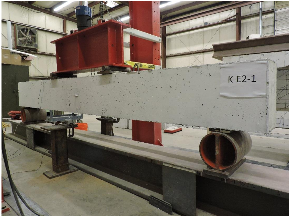
Figure C.2: K-E2-1 Crack Propagation 20 kips
