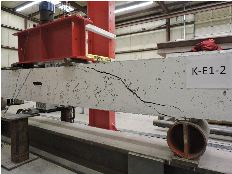
Figure B.10: K-E1-2 Failure Crack Right View
