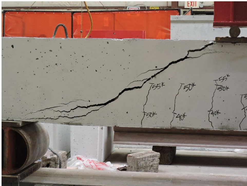
Figure A.12: K-C-2 Failure Crack Front View
