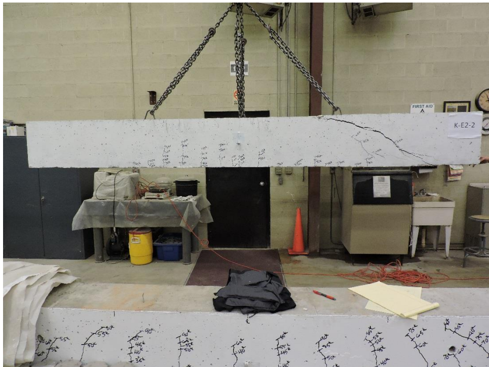
Figure C.14: K-E2-2 Failed Beam
