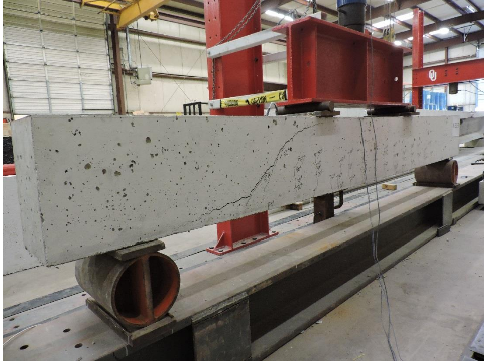
Figure B.13: K-E1-3 Failure Crack Left View
