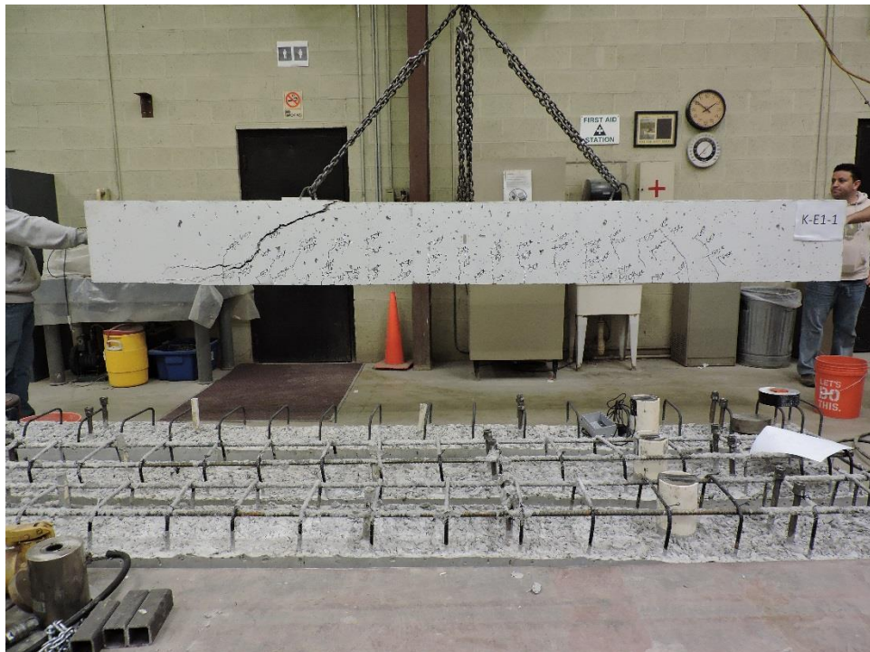
Figure B.6: K-E1-1 Failed Beam
