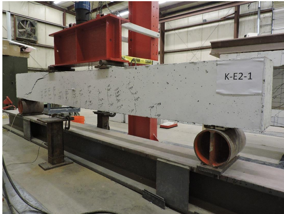
Figure C.5: K-E2-1 Failure Crack Right View
