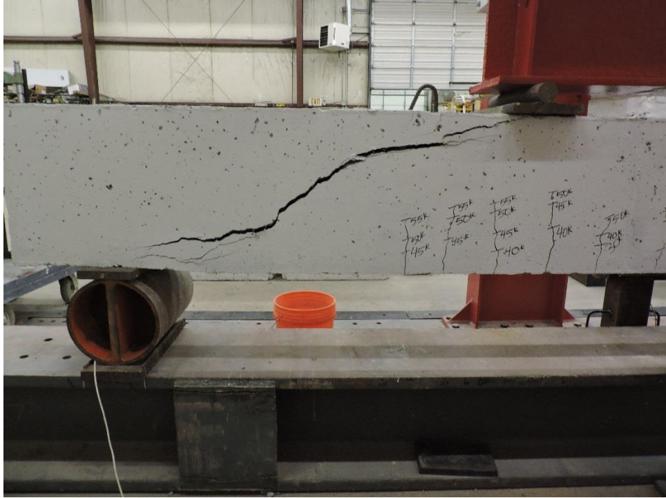
Figure C.7: K-E2-1 Failure Crack Front View
