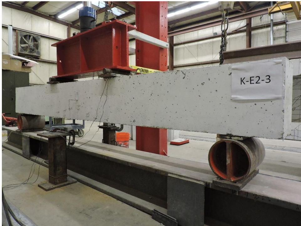
Figure C.15: K-E2-3 Crack Propagation 40 kips
