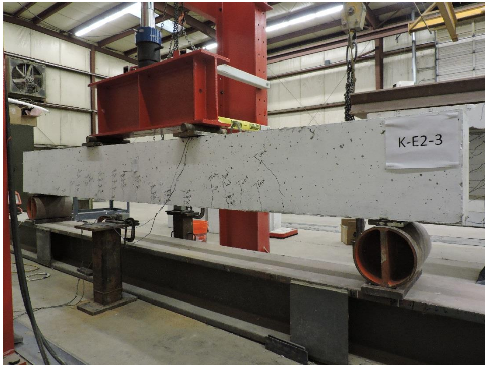
Figure C.17: K-E2-3 Crack Propagation 65 kips
