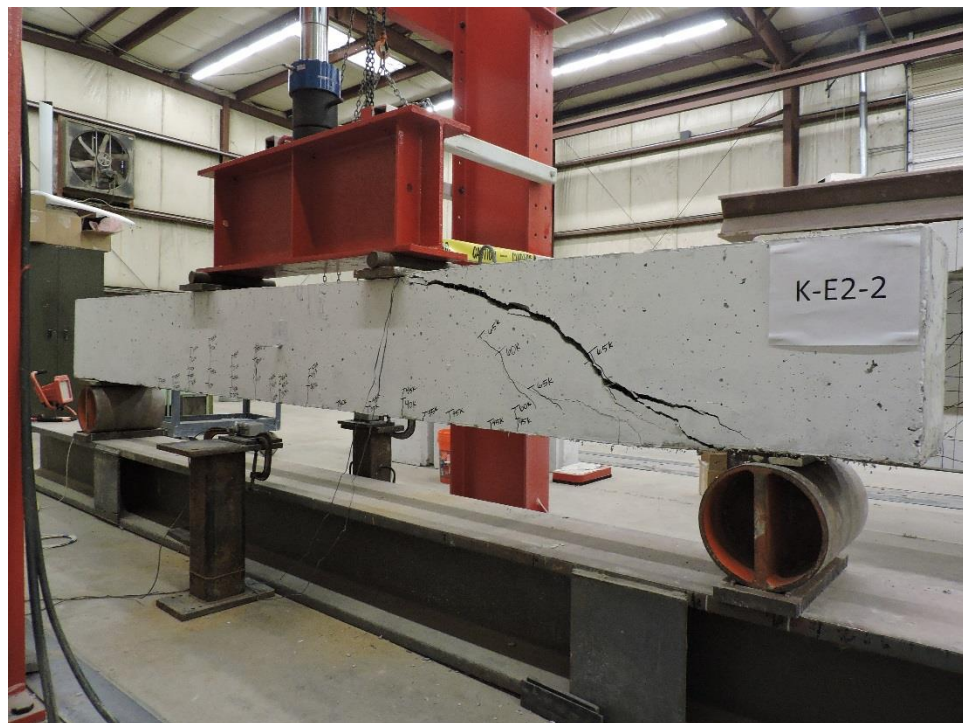
Figure C.12: K-E2-2 Failure Crack Right View
