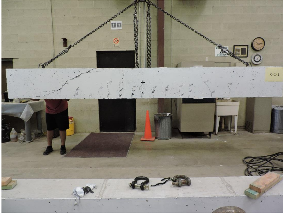
Figure A.7: K-C-1 Failed Beam
