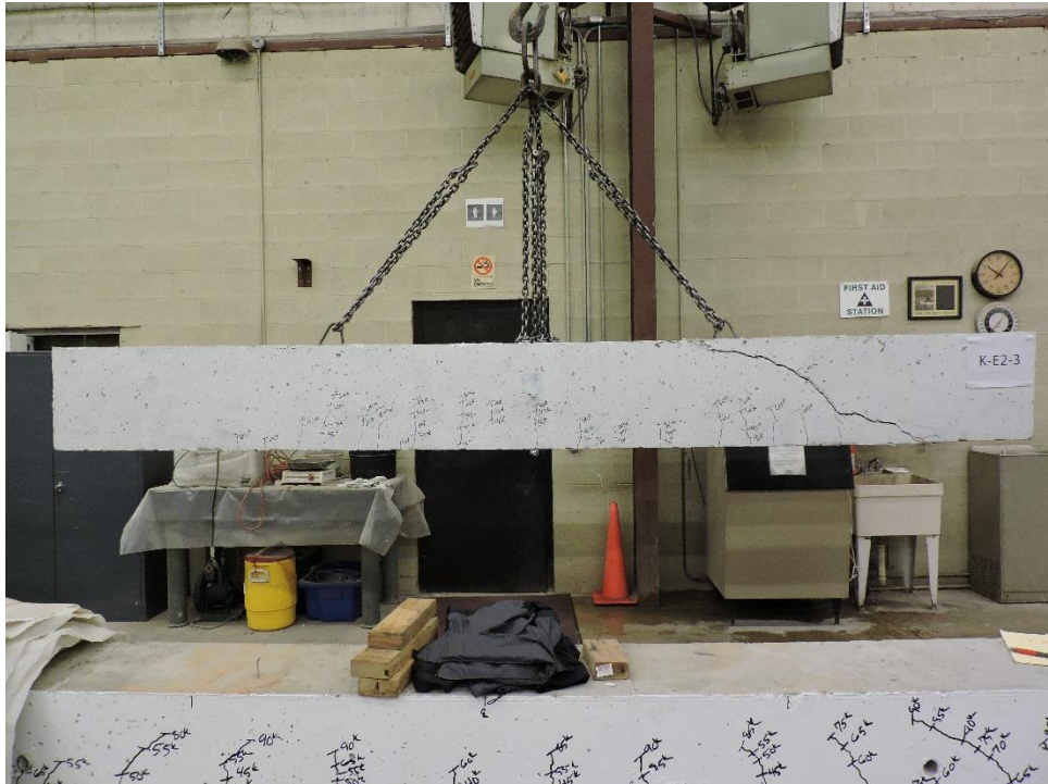
Figure C.20: K-E2-3 Failed Beam
