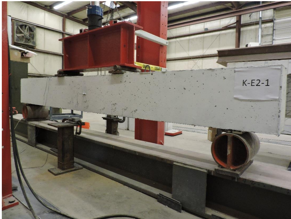
Figure C.3: K-E2-1 Crack Propagation 30 kips
