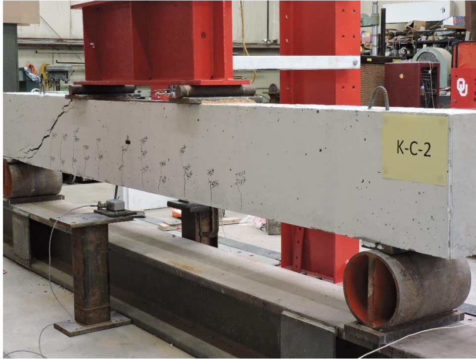
Figure A.11: K-C-2 Failure Crack Right View
