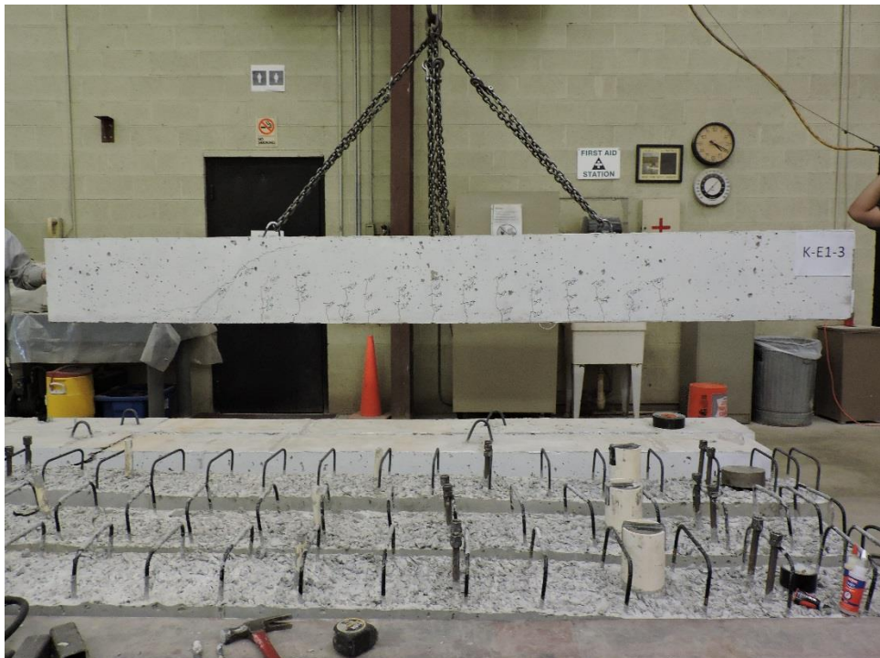
Figure B.14: K-E1-3 Failed Beam
