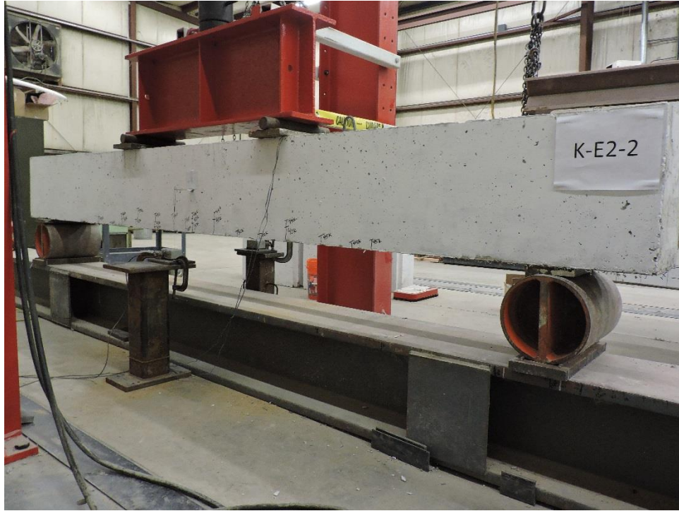
Figure C.9: K-E2-2 Crack Propagation 35 kips
