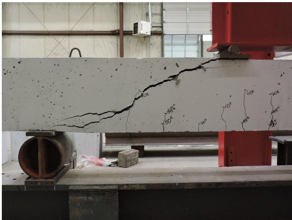
Figure A.6: K-C-1 Failure Crack Front View
