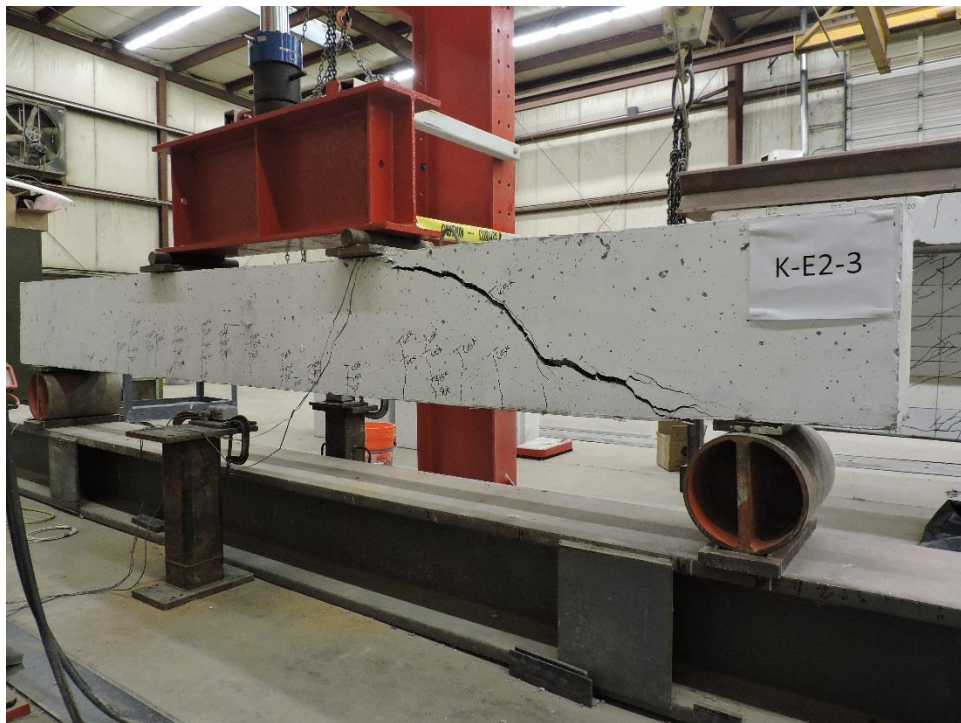
Figure C.18: K-E2-3 Failure Crack Right View
