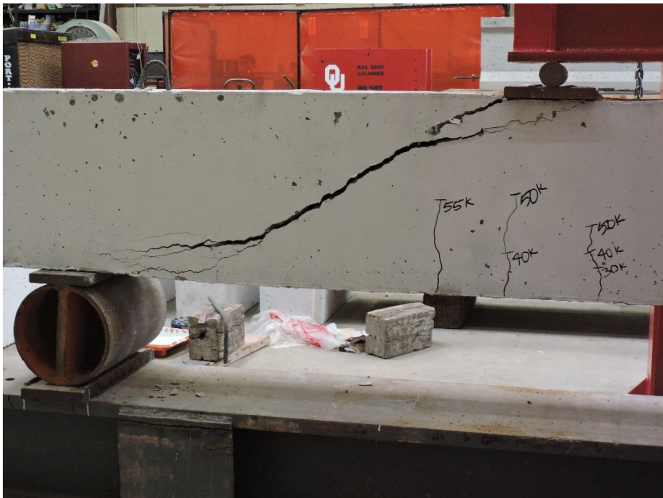
Figure A.18: K-C-3 Failure Crack Front View
