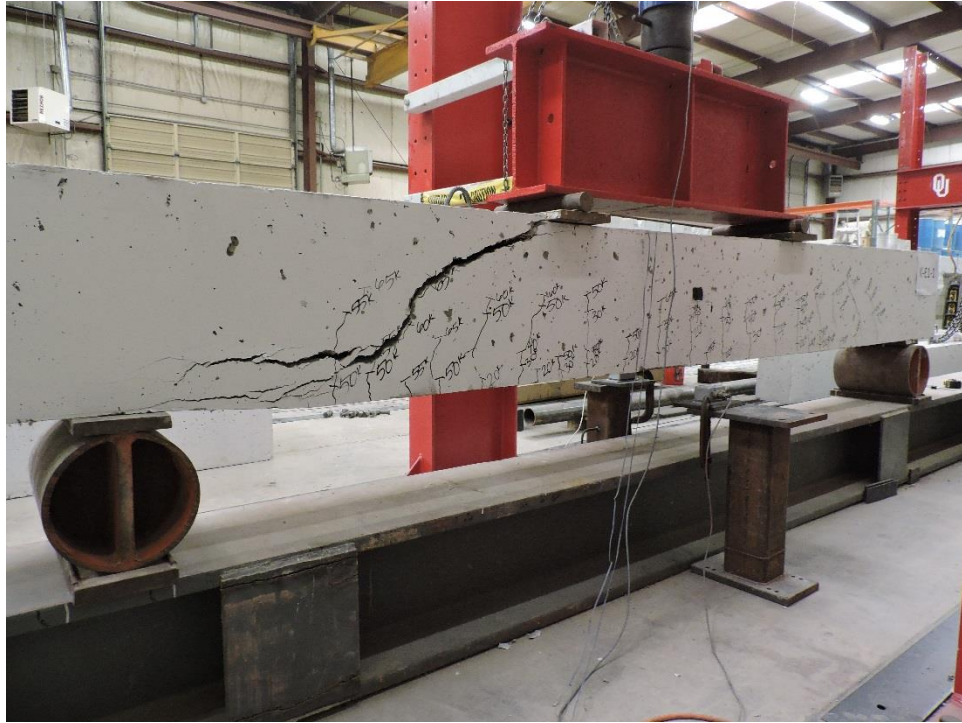
Figure B.5: K-E1-1 Failure Crack Left View
