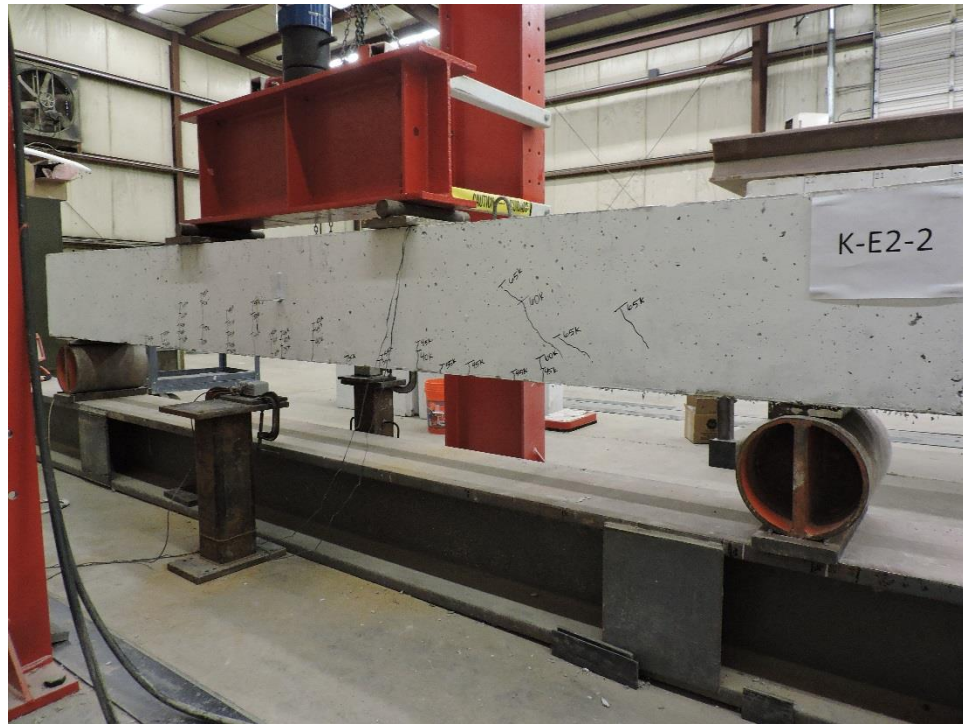
Figure C.11: K-E2-2 Crack Propagation 65 kips
