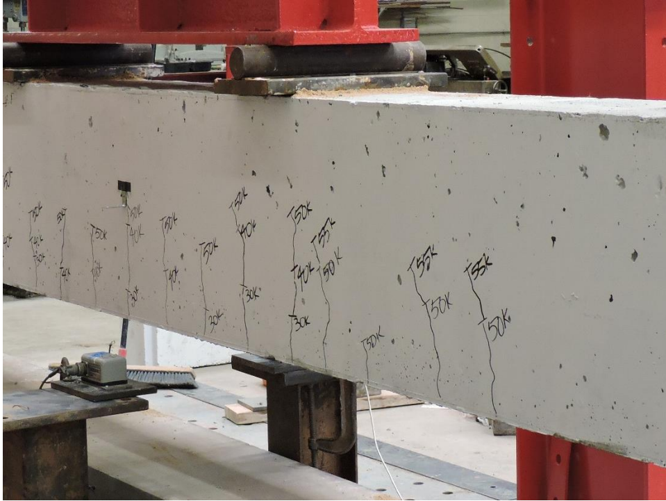
Figure A.15: K-C-3 Crack Propagation
