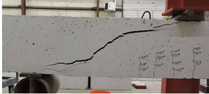
(a) K-E2-1 Failure Crack
