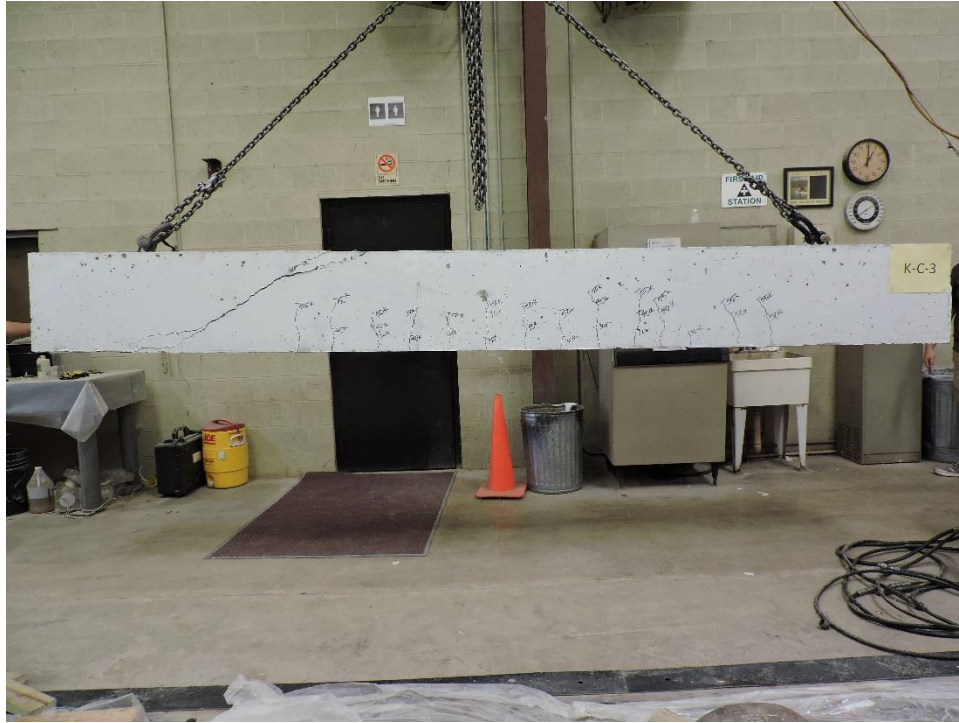
Figure A.19: K-C-3 Failed Beam
