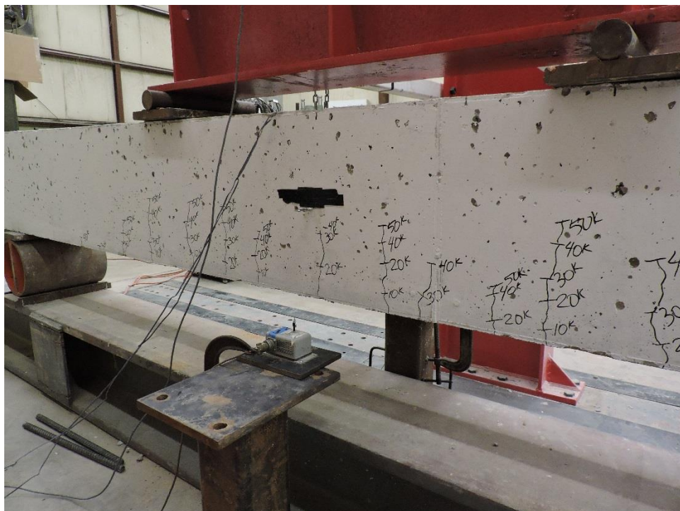
Figure B.8: K-E1-2 Crack Propagation 50 kips
