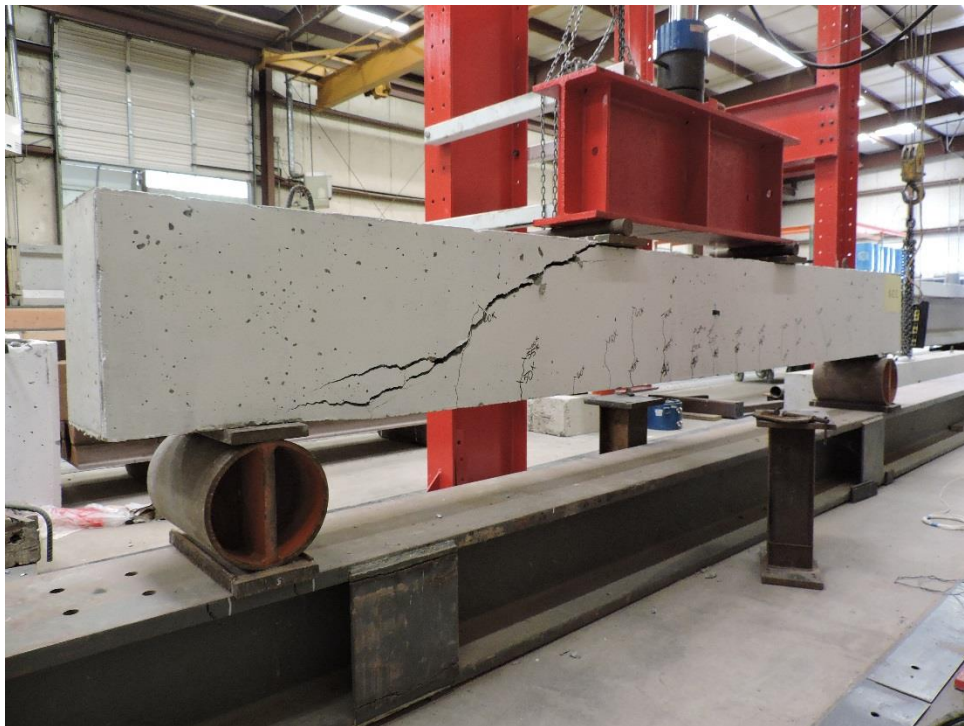
Figure A.4: K-C-1 Failure Crack Left View
