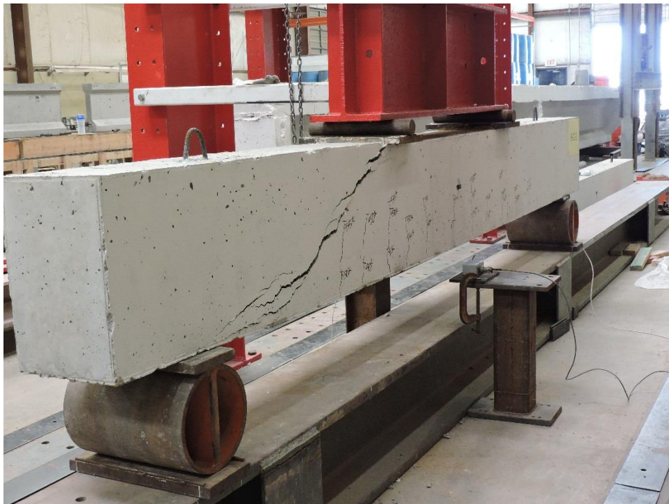
Figure A.10: K-C-2 Failure Crack Left View
