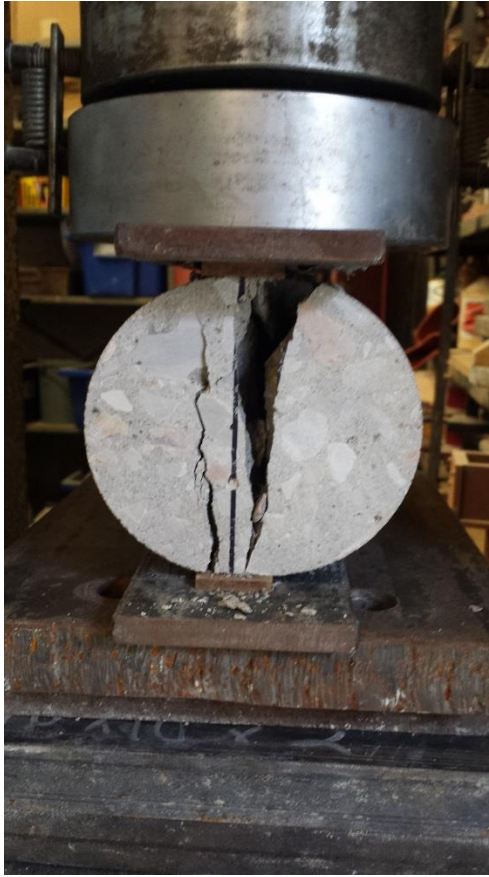
Figure 3.3: Splitting Tensile Test
