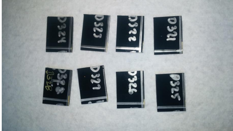
Figure 6: Samples with 1.0% nanotube weight content 1.0in x 0.75in planar size 2.0mm thickness
