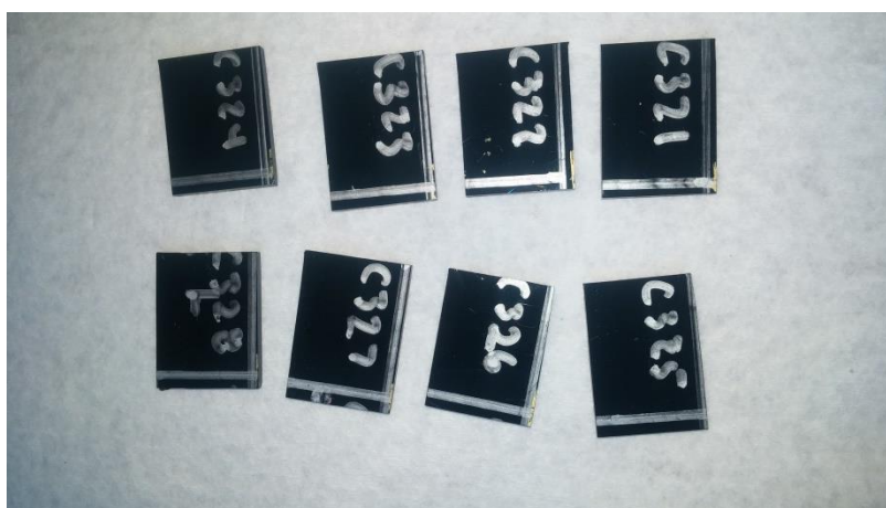
Figure 5: Samples with 0.5% nanotube weight content 1.0in x 0.75in planar size 2.0mm thickness
